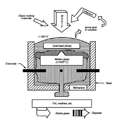
Figure 1. Electric furnace vitrification.
