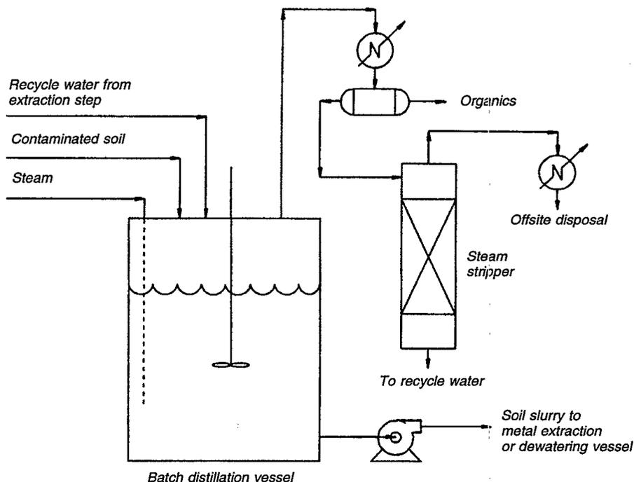
Figure 1. Batch steam distillation step.
