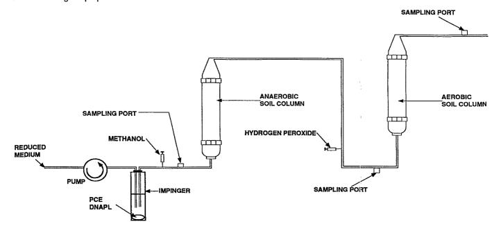
Figure 1. Sequential anaerobic/aerobic treatment.
