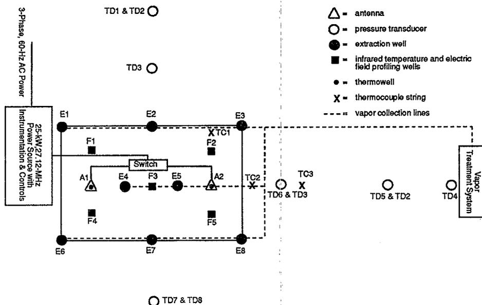
Figure 1. Schematic diagram of KAI RFH system.
