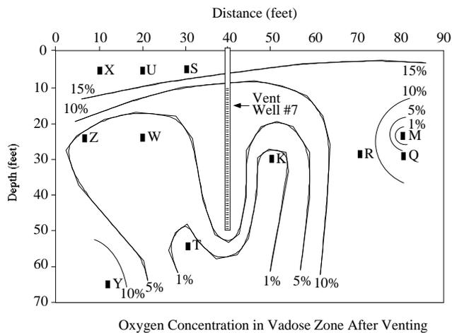
**Figure 8. Oxygen concentration in vadose zone after venting.**
