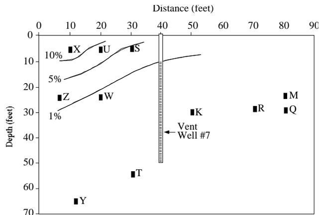
**Figure 7. Oxygen concentration in vadose zone before venting.**
