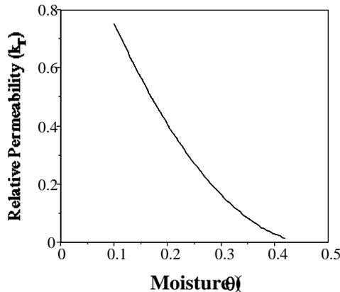
Figure 3. Relative permeability vs moisture content of clay.
