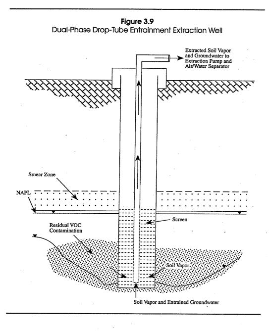
In soil with high hydraulic conductivities, it may be necessary to use a bleed air line to introduce air at the bottom of the drop tube to initiate air and liquid flow up the tube. This approach consists of a small-diameter tube, typically 1.25 cm (1/2 in.) diameter or less, installed along the side of the
