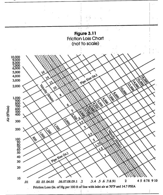
A chart like this, drawn to scale, can be used to compute friction losses in a piping system. For example, determine the friction loss incurred when 70 ft<sup>3</sup>/min flows through a 2 in. pipe, 50 ft long.
