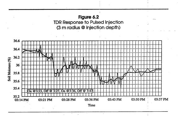
Time series moisture content data collected during pulsed sparging shows a distinct response to each air injection pulse, increasing the displacement of groundwater and improving mixing.
