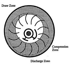
Liquid-Ring Pump Operating Principle
