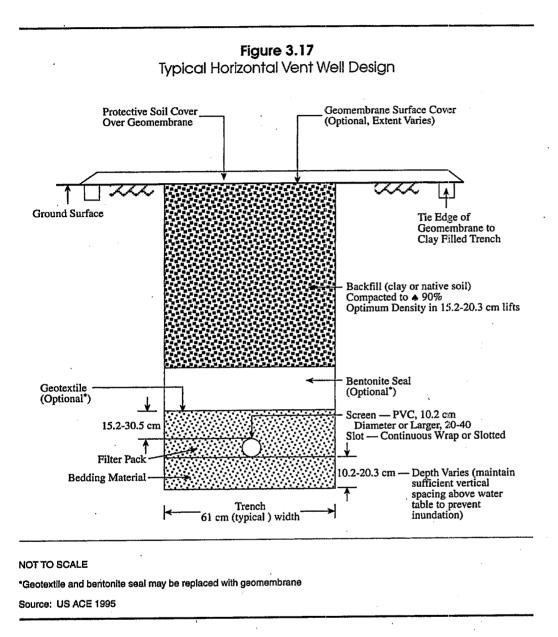
a. *Casing*. Although PVC casing is commonly used, flexible or rigid polyethylene pipe may be more efficient for certain excavation methods such as trenching machines. The pipe must resist the crushing pressures of the backfill and compaction equipment. Reference should be made to the
