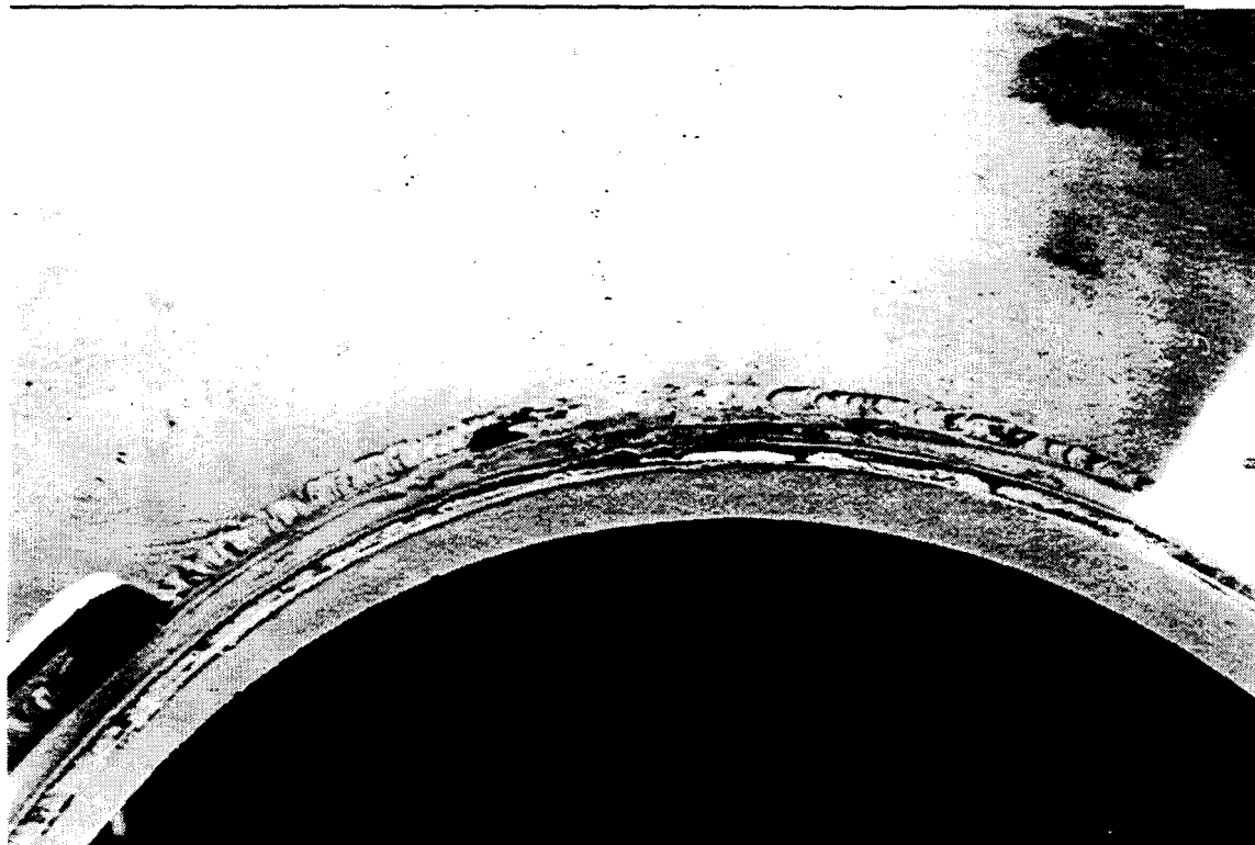
Figure 4: One of the top loading ports on the 150 cubic foot blender showing how the insulation jacket is attached (weld) and access door tabs.
