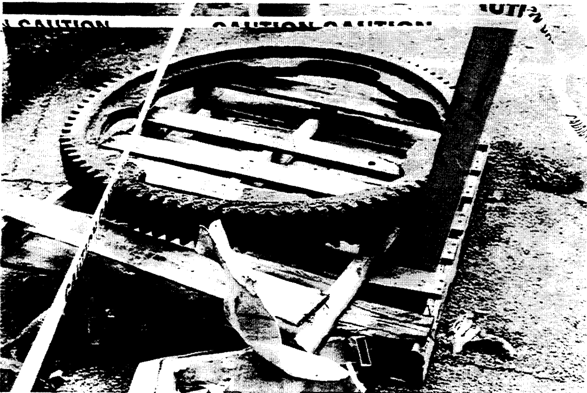
Figure 16: The gear drive side of the blender: a) the shaft (drive side) and b) the portion of the gear that fractured and separated from the blender in the accident.
