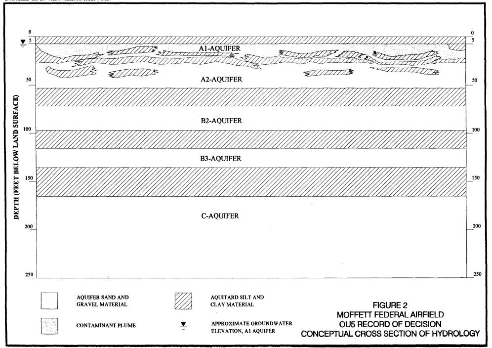
The C aquifer is confined under a laterally extensive clay aquitard (B/C aquitard) that is present beneath Moffett Field between depths of 130 and 160 feet below land surface (bls). The B/C aquitard is a thick, laterally continuous aquitard and the vertical hydraulic gradient is directed upward between the C aquifer and overlying aquifers.
