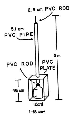
Figure 3 - Jar Sampling Device
