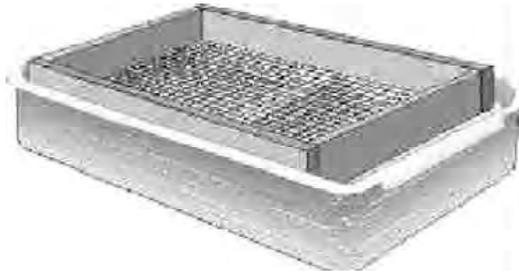
FIGURE 4: FRAMED SCREEN FOR SEPARATING VEGETATION FROM INVERTEBRATES DURING DIPNETTING.
