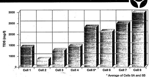
The concentration effect of evaporation can be seen in the increase of total dissolved solids as water moves through the cells.
