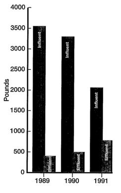
After three years of testing and extended research on JBEW, interesting results have surfaced. The Experimental Wetland is improving the quality of the effluent—it is lower in both phosphorus and nitrogen when it leaves the cells. Research has shown, although plants serve important functions in the filtering, the soils have proved to be the main elements in binding up the phosphorus, thereby preventing it from reaching the nearby Tualatin River.
