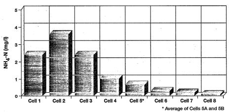
The concentration of ammonium nitrogen is reduced as the water flows through the cells.
