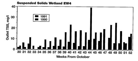
fish story developed in 1990. The solids in the wetland effluents were steadily increasing with each passing week. The source of the problem was found: a large number of carp were growing up in the wetlands. These fish foraged in the wetland sediments, causing resuspension of solids. They entered as fry in the pumped water, and grew to 8-10 inches
