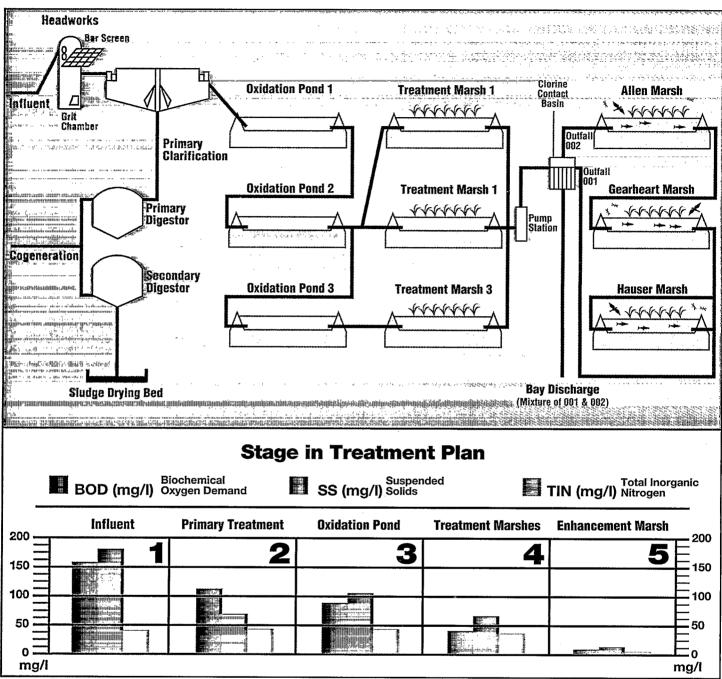
rcata's present wastewater treatment plant consists of seven basic components. These are the headworks, primary clarification, solids handling, oxidation pond, treatment marshes, enhancement marshes and disinfection. Each one of these components will be detailed as follows.
