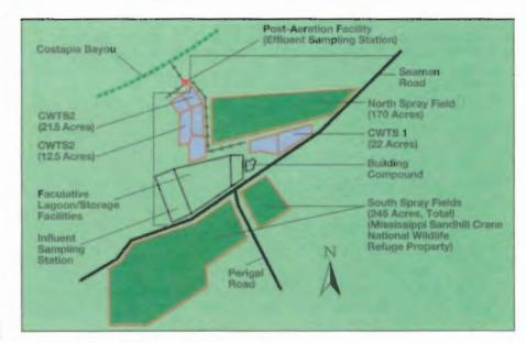
was sufficient to treat the wastewater produced within the service area, which is primarily from household sources. However, following heavy rainfall events, hydraulic capacity of the land treatment facility was exceeded, and excess flow was bypassed directly into Costapia Bayou. Wetlands were constructed to increase the site's overall treatment capacity to 2.6 mgd and to eliminate this periodic bypass.
