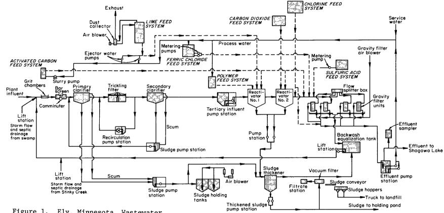
Figure 1. Ely, Minnesota, Wastewater Treatment Plant Normal Flow Schematic
