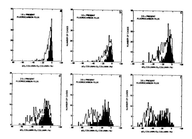
Frequency distributions of Monte Carlo model results for changes in total column ozone as a function of fluorocarbon flux. The shaded areas show the cases for which the NO, NO2, and ClO concentrations all fell within the range of measurements at  $25~\rm km$ .
