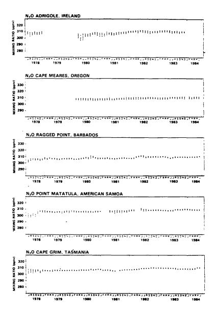
Rates of increase in tropospheric nitrous oxide at the five monitoring stations above are: 0.77%, 0.27%. 0.24%, 0.09%, and 0.18%. While the rates of increase appear to be larger in the Northern hemisphere than in the southern hemisphere, there is little variation in actual concentrations. Data are from the Atmospheric Lifetime Experiment.
