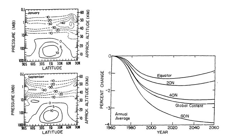
Calculated percent changes in ozone from 1960 to 2060 for constant CFC-11 and CFC-12 emissions and annual increases in CH4 and N2O concentrations of 1 percent and 0.25 percent, respectively. Model does not include CFC-113 or Halons, and assumes constant emissions of CCl4 and methyl chloroform.
