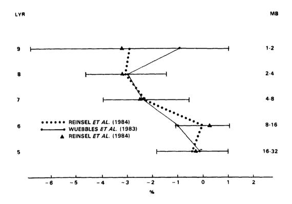
Changes in ozone by altitude for 1970 to 1980. The data "analysis indicate statistically significant trends in the upper Umkehr layers 7 and 8 of the order of -0.2 to -0.3 percent per year over the period 1970-1980, with little trend in the lower layers 5 and 6.
