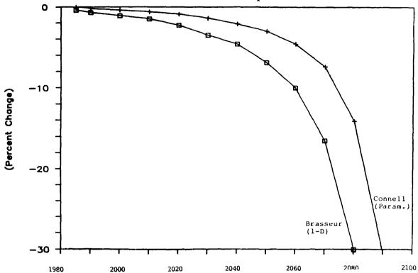
Time-dependent change in ozone, as calculated by the 1-D model of Brasseur and DeRudder (1986) and Connell's parameterization of the LLNL 1-D model. Trace gas assumptions are shown in Exhibit 5-30 and may be summarized as:
