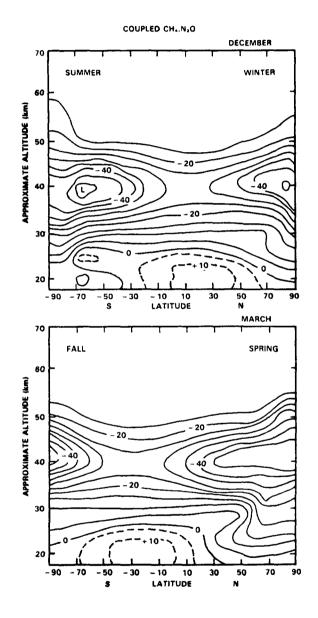
Steady-state changes in ozone by latitude and altitude as calculated by the GS 2-D model. For Scenario S2C: Clx = 8 ppbv plus 2 x CH4 and 1.2 x N2O. Top panel shows results for December, bottom panel for March. Changes are relative to reference atmosphere with 1.3 ppbv Clx.
