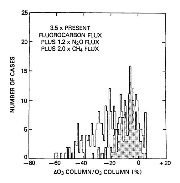
Frequency distribution of Monte Carlo model results for changes in total column ozone for 3.5 times the present fluorocarbon flux, 1.2 x N2O flux, and 2 x CH4 flux. The shaded area shows the cases for which the NO, NO2, and ClO concentrations all fell within the range of measurements at 25 km.
