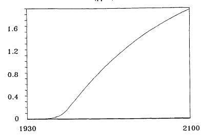
If future emission of CFC-12 were held constant at today's levels (A), atmospheric concentrations would continue to rise for over 100 years (B). Computed with simplified model of source and loss terms. See Appendix to Chapter 2.
