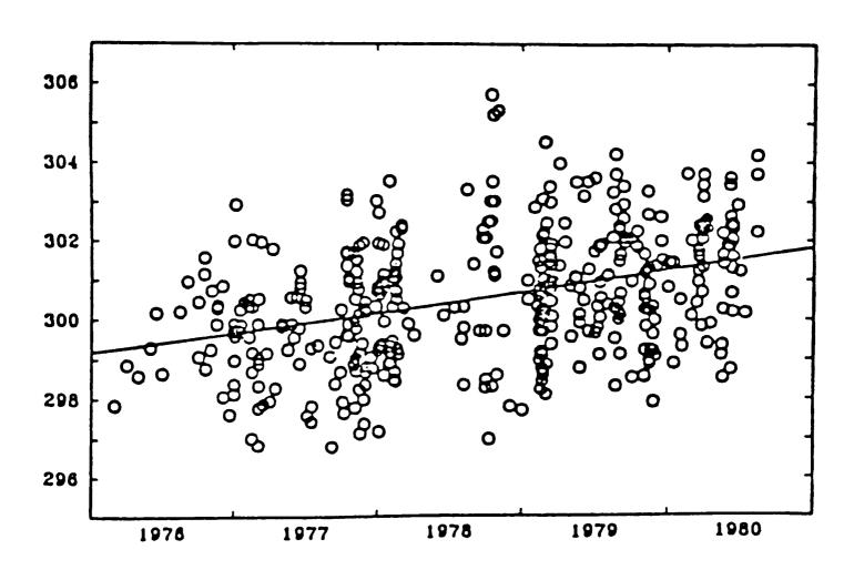
Measurements of tropospheric nitrous oxide concentrations. Data were collected at several monitoring sites and aboard vessels in the major world oceans. Concentrations are increasing at approximately 0.2 percent per year.
