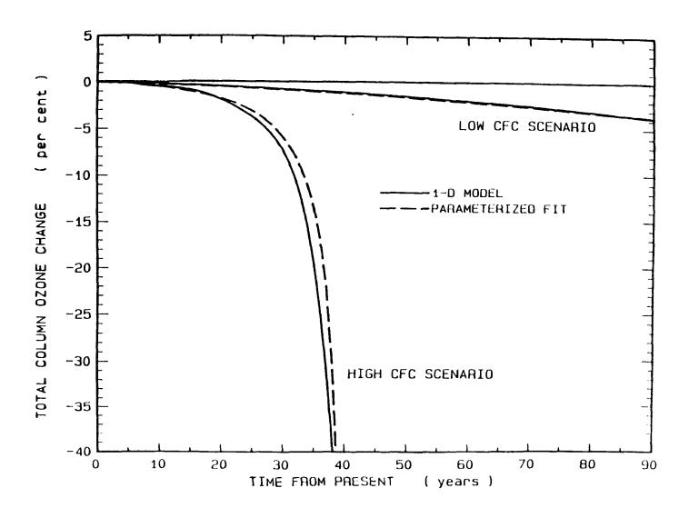
Time-dependent change in ozone as calculated by LLNL 1-D model and parameterized fit for two divergent scenarios of growth in CFCs and other trace gases. "Differences between the parameterization and the full 1-D model are generally less than one percent except at very large depletions."
