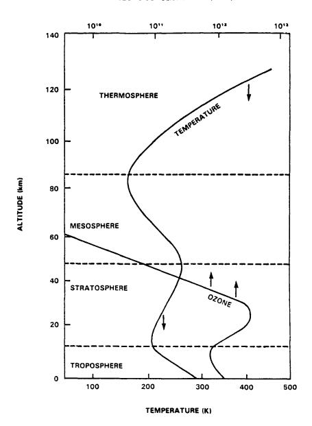
The ozone layer has a peak concentration in the lower stratosphere between about 20 and 25 kilometers altitude. In the troposphere, temperature decreases with altitude. In the stratosphere, temperature increases with altitude.
