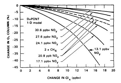
Results from Owens and Fisher of Dupont. Calculated ozone change is presented as a function of stratospheric Clx for different values of stratospheric NOy (NO, NO2, NO3, N2O5, C1ONO2, NHO4, and HNO3). For large background NOy (about 30 ppb) the decrease of ozone is small and very nearly linear with increasing Clx, but for small background NOy (13 ppb), ozone is strongly and non-linearly reduced by Clx.
