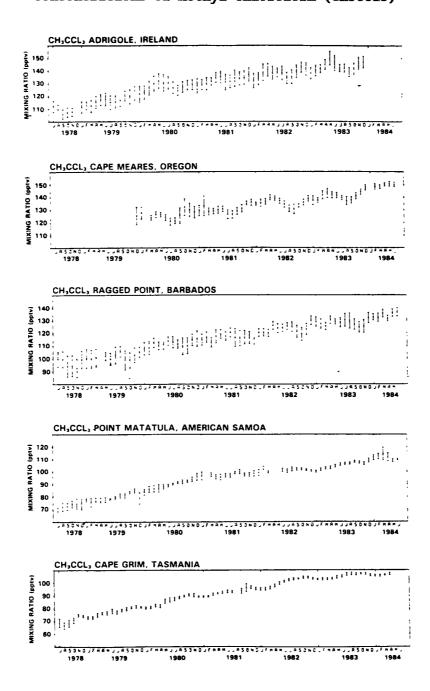
Average concentrations of methyl chloroform are increasing at approximately seven percent per year. Data are from the Atmospheric Lifetime Experiment.
