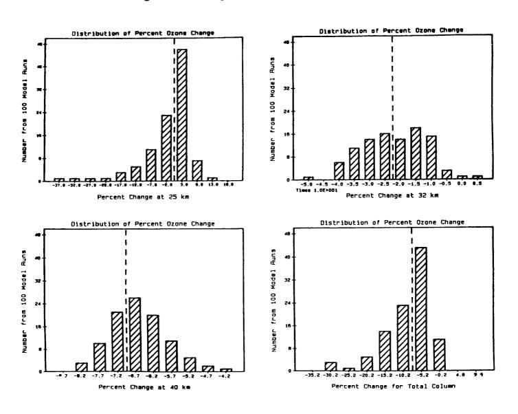
Frequency distributions of Monte Carlo model results for changes in ozone. Top left panel shows results for 25 km, top right for 32 km, bottom left for 40 km, and bottom right for total column ozone. Perturbations are: 15 ppbv Clx, 2x CH4, and 1.2x N20.
