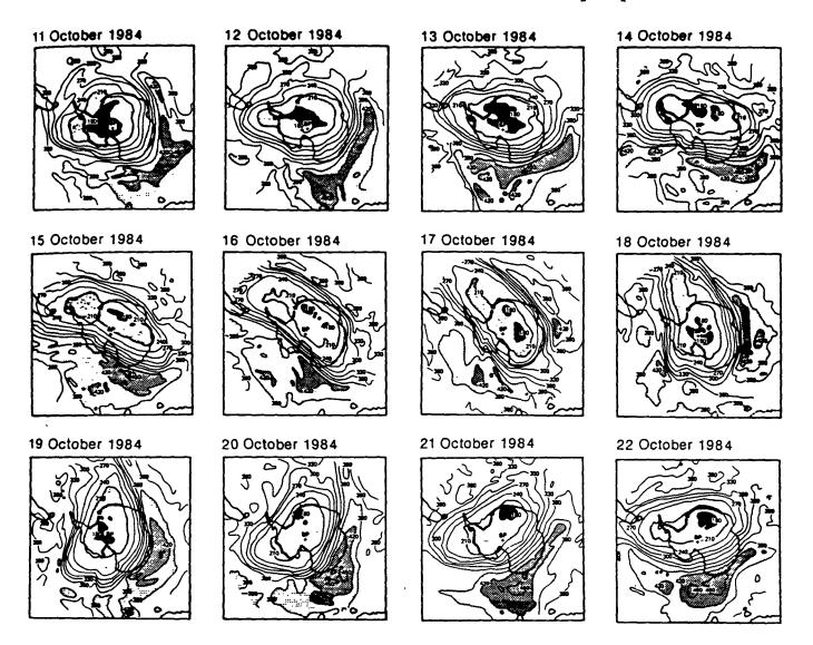
"Twelve-day sequence (11-22 October 1984) of TOMS measurements of total ozone content. The data are shown in south polar projections, with the pole indicated by a cross (SP) and Halley Bay shown by an asterisk. Contours are every 30 Dobson units (1 DU =  $10^{-3}$  atm cm). The region shown extends to  $45^{\circ}$  latitude and the Greenwich meridian is towards the top of each diagram. Shaded regions indicate total ozone values <180 and 210 DU and >390 and 420 DU."
