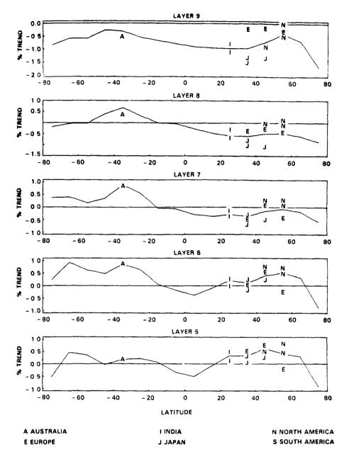
Ozone trend estimates for November 1978 to April 1982, as determined by SBUV data, are indicated by solid line. Superimposed letters indicate results from Umkehr stations.
