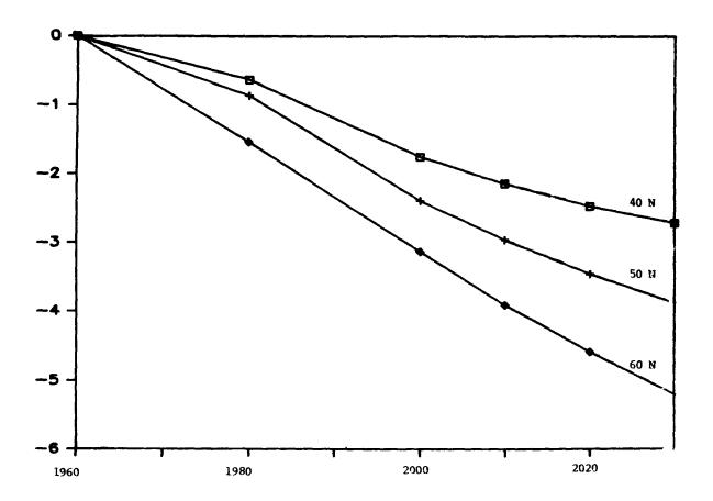
Results shown for 1.2 percent growth per year in CFC emissions, 1 percent growth in CH4 concentrations, 0.25 percent growth in N20 concentrations, and approximately 0.5 percent growth in CO2 concentrations. Methyl chloroform and CCl4 are essentially capped; halons eliminated. Changes shown for  $40^{\rm o}$ N,  $50^{\rm o}$ N, and  $60^{\rm o}$ N. Temperature feedback considered in model.
