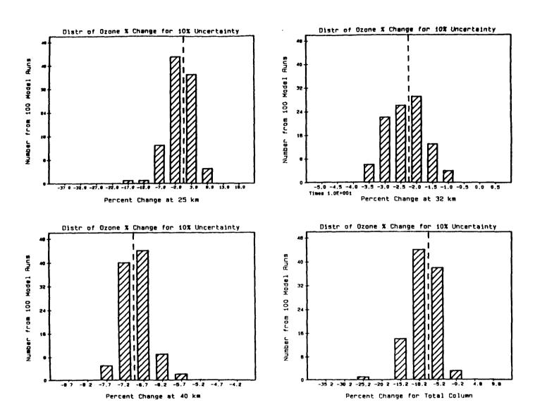
Frequency distributions of Monte Carlo model results for changes in ozone, when uncertainties in input parameters are reduced to 10 percent. Top left panel shows results for 25 km, top right for 32 km, bottom left for 40 km, and bottom right for total column ozone. Perturbations are: 15 ppbv Clx, 2x CH4, and 1.2x N20.
