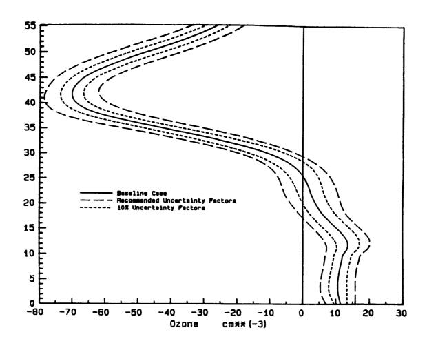
Results from Monte Carlo analysis of uncertainties regarding rate constants. Solid line shows calculated changes in ozone by altitude for mean values of input parameters. Dashed lines show calculated changes for recommended uncertainty factors. Dotted lines show calculated changes for uncertainties which have been reduced to 10 percent. Perturbations are: 15 ppbv Clx, 2x CH4, and 1.2x N2O.
