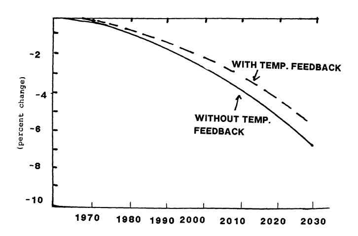
Results shown are for globally and seasonally average depletion for model experiment with and without temperature feedback from  ${\tt CO2}$  cooling.
