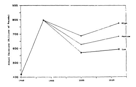
Future carbon monoxide emissions from combustion, as projected by Kavanaugh (1986). The case of the expected decline is the penetration of efficient engines into world markets, the substitution of cleaner fuels, and the increased use of pollution reduction equipment in transportation.
