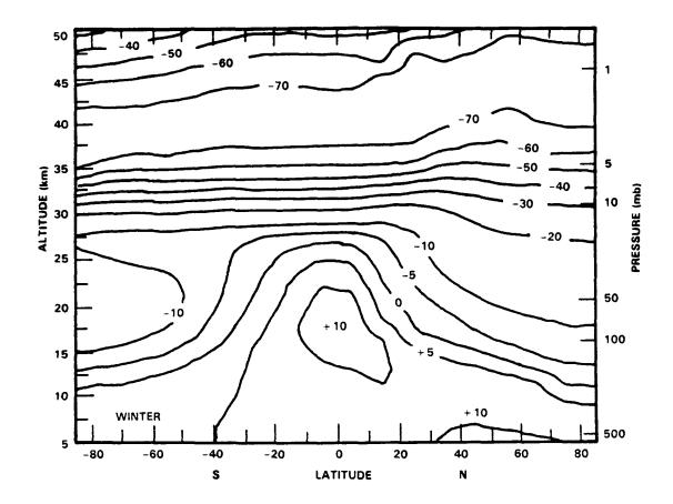
Steady-state changes in ozone by latitude and altitude in winter as calculated by the MPIC 2-D model for Scenario SMC: ClO - 15.3 ppbv plus 2 x CH4 and 1.2 x N2O. Changes are relative to reference atmosphere with 2.7 ppbv ClO.
