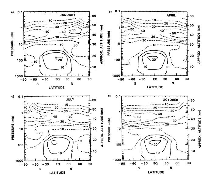
Results from AER 2-D model, for scenario #S2A, relative to reference atmosphere with 1.3 ppb Clx (see Exhibit 5-9). Panel a shows percent change in ozone in January, panel b in April, panel c in July, and panel d in October.
