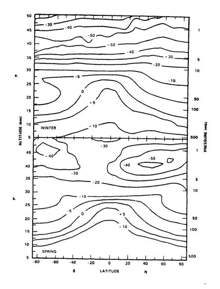
Steady-state changes in ozone by latitude and altitude as calculated by the MPIC 2-D model. For Scenario SMB: Clx = 9.5 ppbv plus 2 x CH4 and 1.2 x N2O. Panel a shows results for winter, panel b for spring. Changes are relative to reference atmosphere with 2.7 ppbv Clx.
