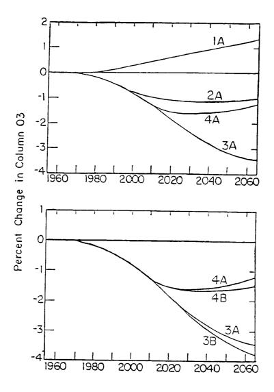
Time-dependent change in ozone as calculated by the AER 1-D model for several scenarios of growth in trace gas emissions and concentrations, shown in Exhibit 5-29. The results indicate that global average depletion over one percent will occur if growth in CFCs and other potential ozone depleters continues.
