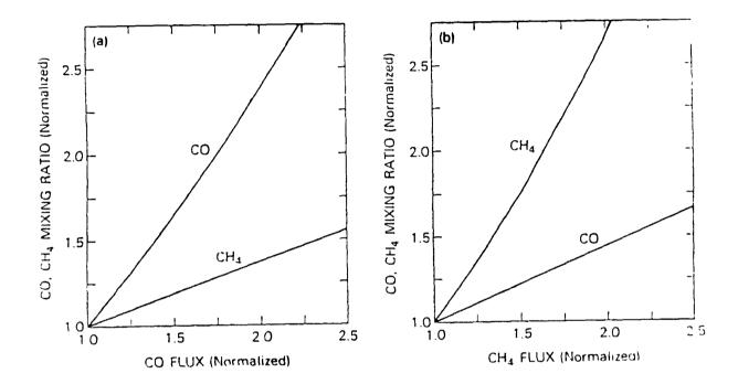
As a consequence of coupling between CO and CH4, due to their reactions with OH, concentrations of CH4 can increase both through increases in CO fluxes (a) and CH4 fluxes (b).
