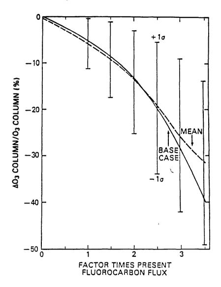
The calculated change in total column ozone as the fluorocarbon flux increases. The sold line shows the base case, which uses the mean value for each input parameter. The dashed line shows the mean depletion from the 329 model runs. The vertical bars show the 1-sigma uncertainty limits.
