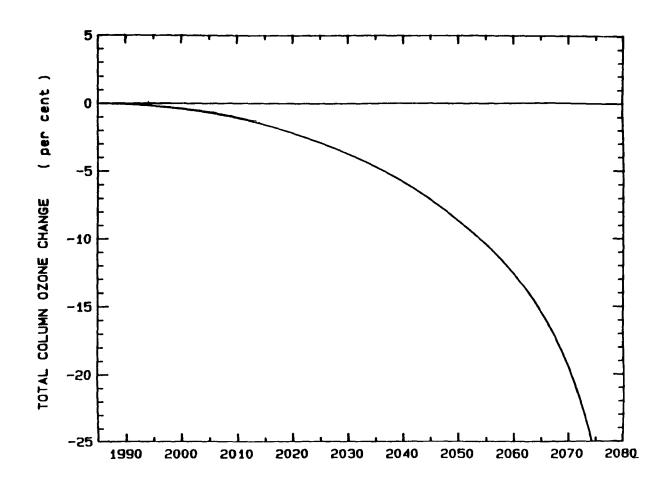
Total column ozone change for "reference case" scenario of trace gases: ~2.5 percent growth in CFC emissions, concentrations of CH4 at 1 percent, N2O at 0.25 percent, and carbon dioxide at ~0.6 percent.
