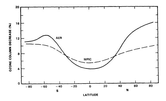
Ozone column decrease in April for Clx increase of about 7 ppbv. The AER 2-D model shows more variation with latitude than the MPIC model. This difference can be attributed to differences in transport, especially the rate of horizontal mixing.
