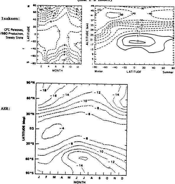
Results from IS 2-D model, for an increase in Clx from 1.0 ppbv to 7.2 ppbv. The bottom panel depicts changes of 1.3 to 8.2 ppbv Clx for the AER 2-D model. Both panels show change in the total ozone column as a function of latitude and time of the year.
