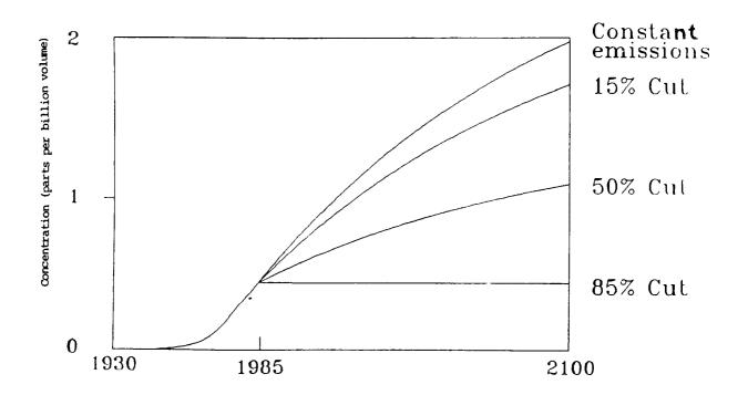
For CFC-12, holding emissions constant at 85% of today's level (a 15 percent cut), would allow concentrations to increase by a factor of four. Only an emission cap at 15 percent of today's level (an 85 percent cut) could hold concentrations constant. Computed with simplified model of source and loss terms. See Appendix to Chapter 2.
