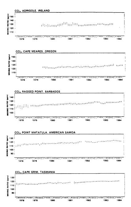
Average concentrations of carbon tetrachloride are increasing at approximately one percent per year. Data are from the Atmospheric Lifetime Experiment.
