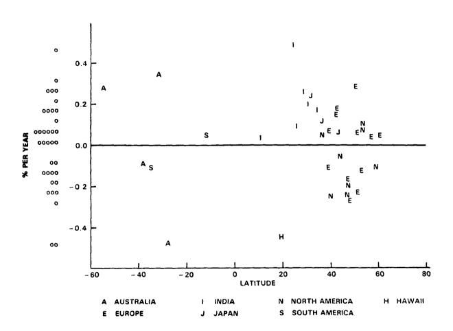
Recent ozone trend estimates from ground-based observation networks. Horizontal axis shows latitude of measurement. Legend identifies each site. Vertical axis shows histogram of trend estimates.
