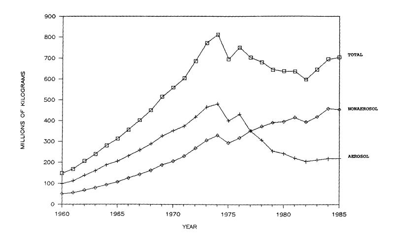
Total reported production of CFC-11 and CFC-12 increased rapidly throughout the 1960s and 1970s, reaching a maximum of 813 thousand metric tons in 1974. Aerosol applications declined since the mid-1970s, while nonaerosol applications continued to increase. (Note: aerosol/nonaerosol divisions prior to 1976 are estimates.)
