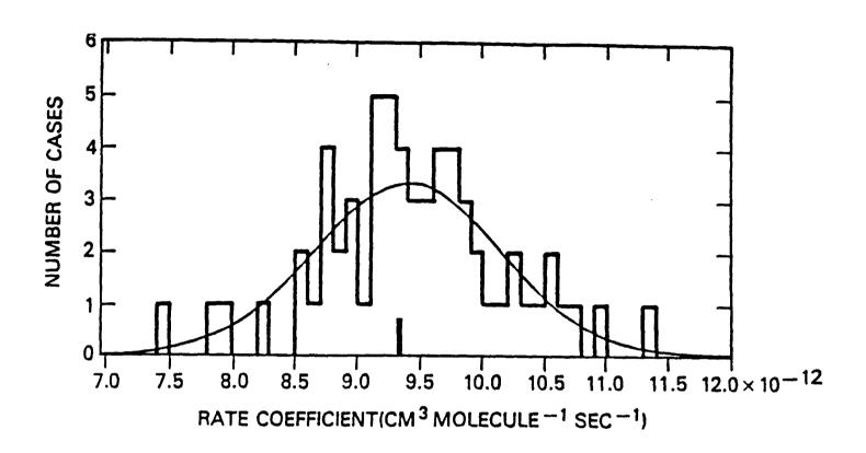
Histogram of individual data points for the rate coefficient of the reaction  $0 + NO2 \longrightarrow PO2 + NO$ . The measurements have been fit to a smooth curve that forms a probability distribution to be used in Monte Carlo calculations.
