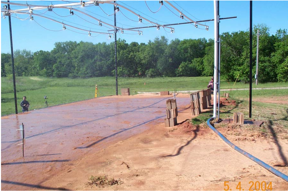
Figure 4-6. Pump connection to the simulator
