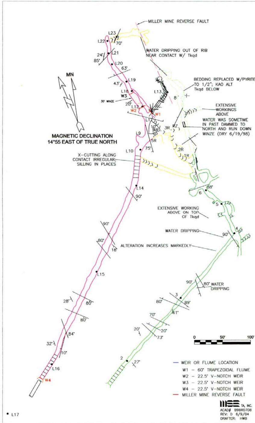
Figure 2-1. Initial Miller Mine underground workings plan map showing the weir, flume, and sample port locations W1, W2, W3, and W4 (AutoCAD drawing B98R0708)
