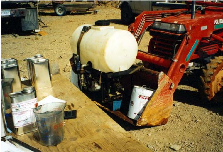
**Figure 5-2. Kubota tractor that transported the grout and grout equipment into the abandoned underground workings of the Miller Mine.**
