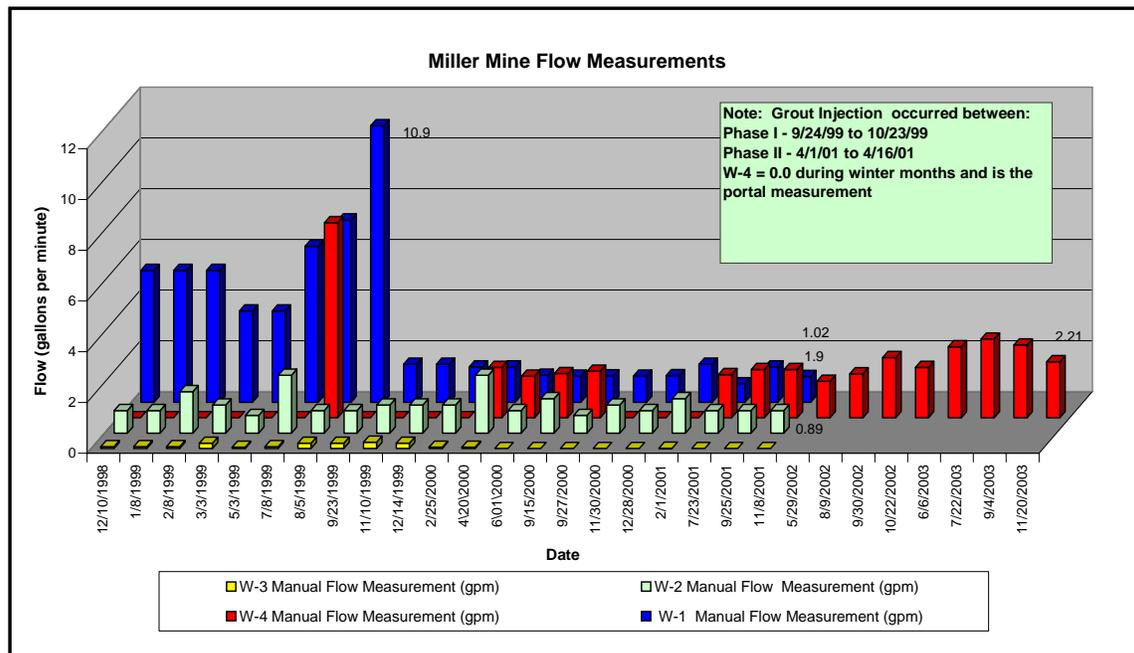
Figure 6-2. Miller Mine flow measurement taken at the respective locations throughout the mining system. Note that the Miller Mine became unstable, and measurements for W1, W2, and W3 were discontinued in November 2001.
