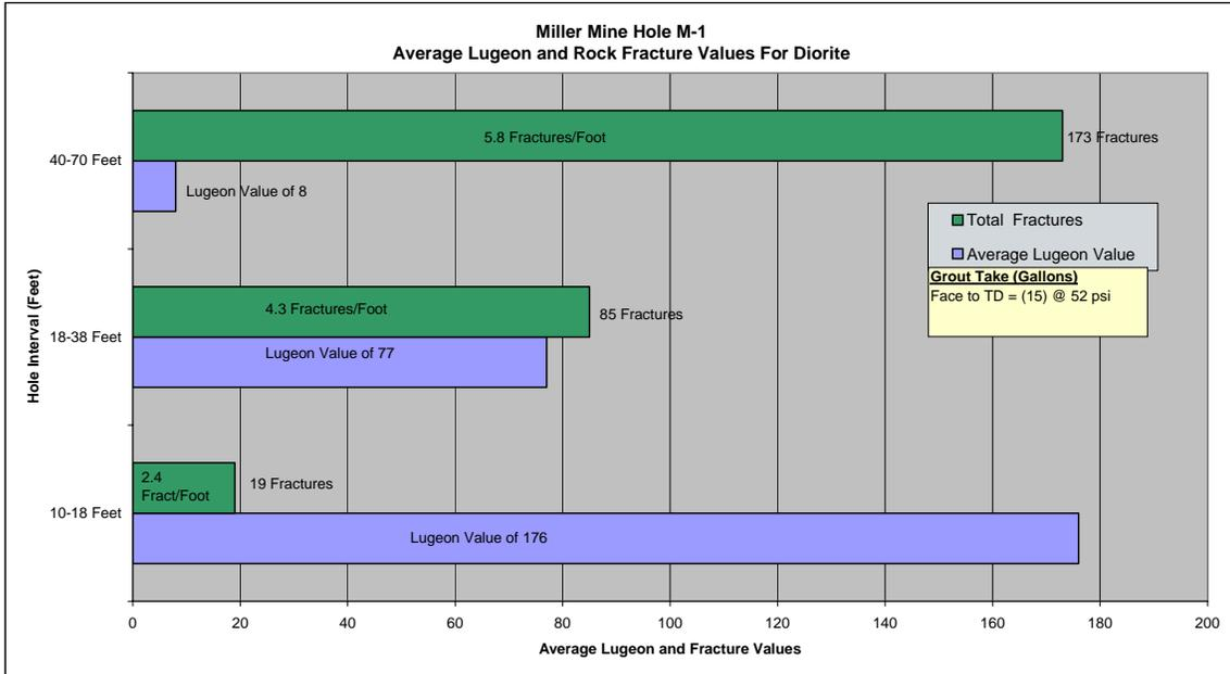
Figure 4-1. Plot of the average Lugeon and fracture density for grout hole M1.
