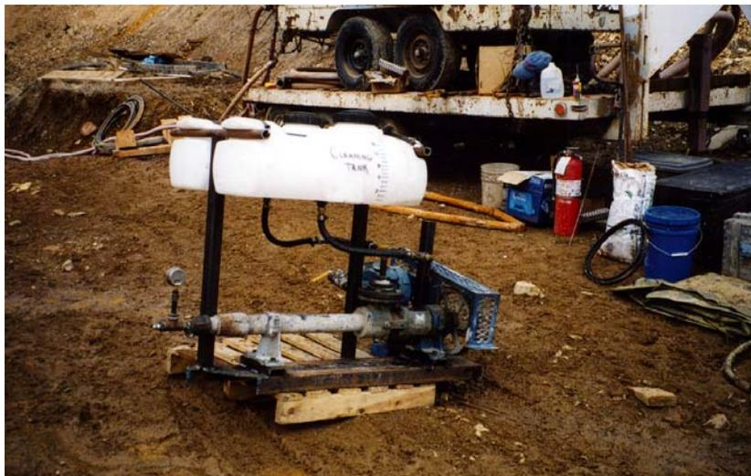
**Figure 3-2.** Photograph of the grout pump, tanks, and flowmeter system for the Stage I grout injection in 1999.
