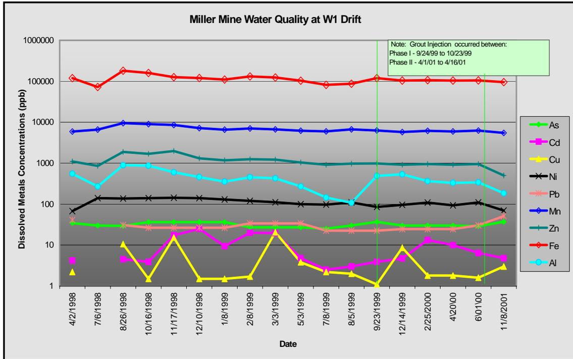
Figure 6-3. Miller Mine water quality results for the W1 drift, the area where most of the dissolved metals were originating. The water quality results reflect the dissolved metals concentrations at W1 micrograms per liter.
