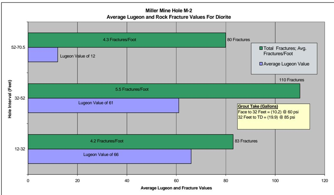
Figure 4-2. Plot of the average Lugeon and fracture density for grout hole M2.
