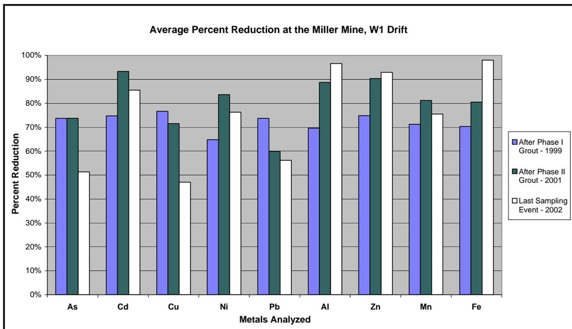
Figure 6-4. Average percent reduction for metals loading at the W1 drift prior and after each phase of grouting.
