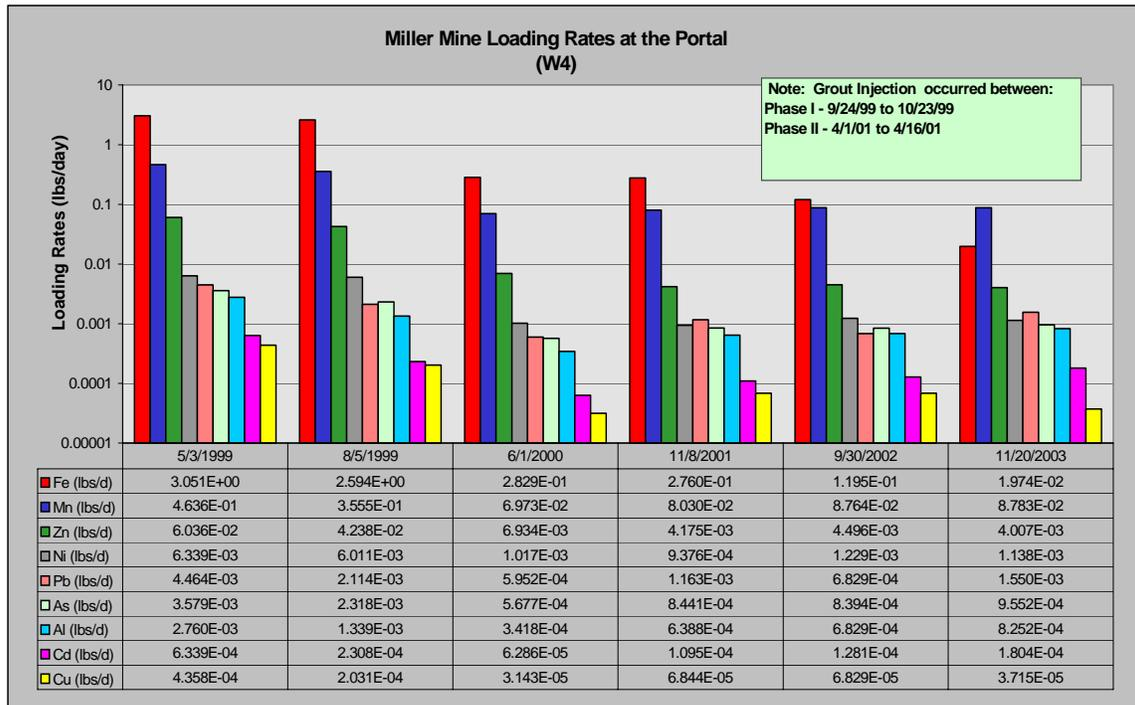
Figure 6-8. Metals loading for the Miller Mine portal (sampling results from port, W4).
