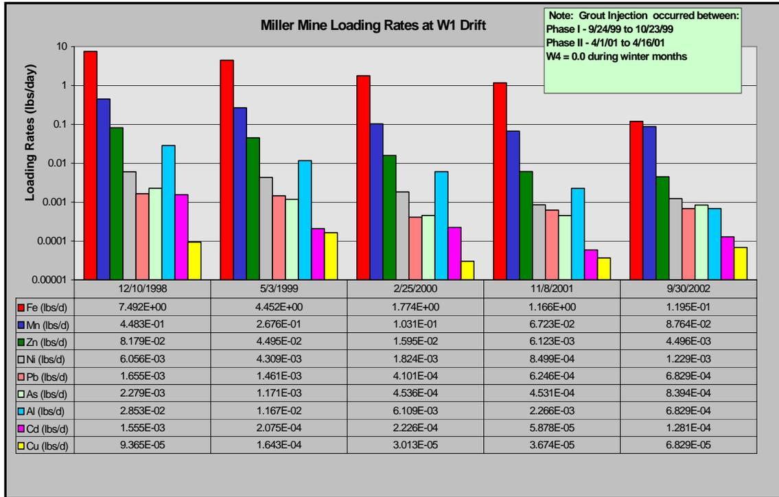
Figure 6-5. Metals loading at the W1 drift sample port located in the underground workings of the Miller Mine.
