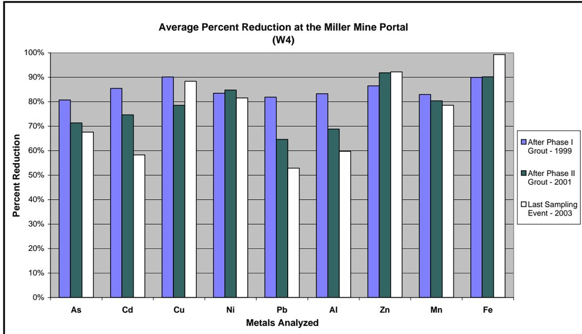
Figure 6-7. The average percent reduction in metals loading at the Miller Mine portal after grout injection.
