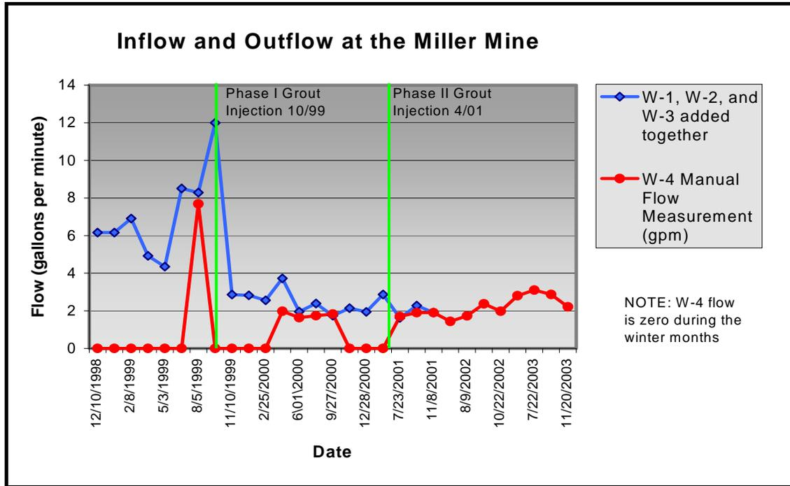
Figure 6-1. Inflow (W1, W2, W3 added together) and outflow (W4) measurements compared over time to evaluate losses and fluctuations due to grout injection.
