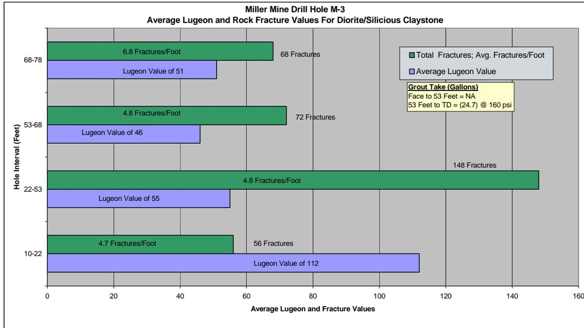
Figure 4-3. Plot of the average Lugeon and fracture density for grout hole M3.
