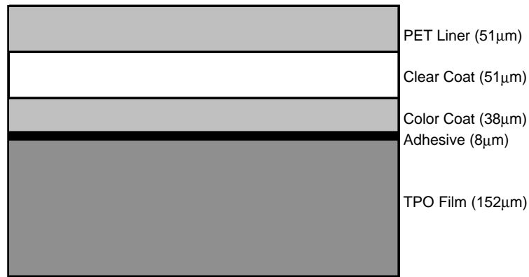
Figure 2-1. Cross-section of 3M ISF (PET Liner is removed prior to application)
