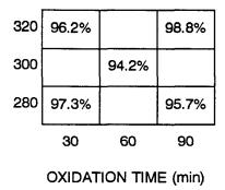
Figure 5. Percent Destruction of PAH in Solids as a Function of Operating Conditions.
