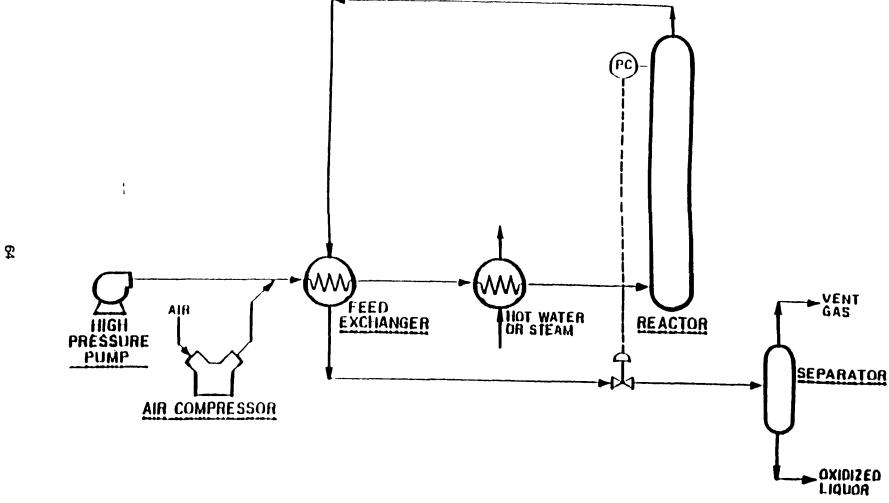
Figure 1-1. Wet Oxidation Flow Diagram (Source: Zimpro Passavant)
