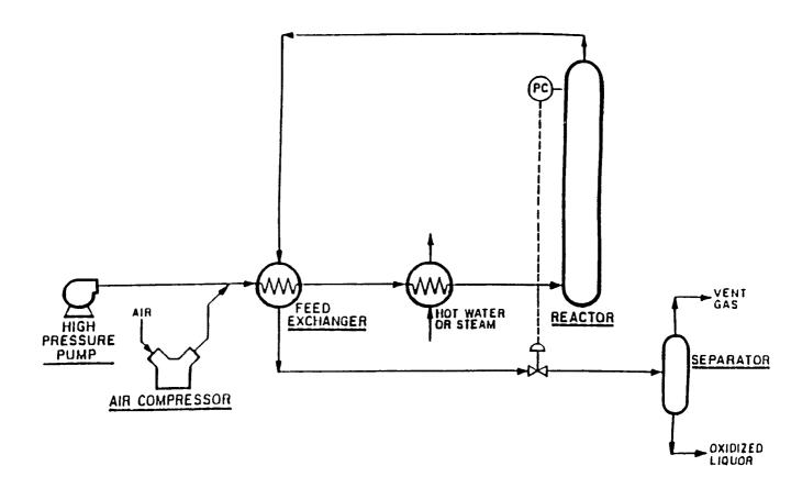
Figure 3. Flow Diagram for the Zimpro Wet Air Oxidation Process. (Source: Zimpro Passavant Environmental Systems, Inc.)
