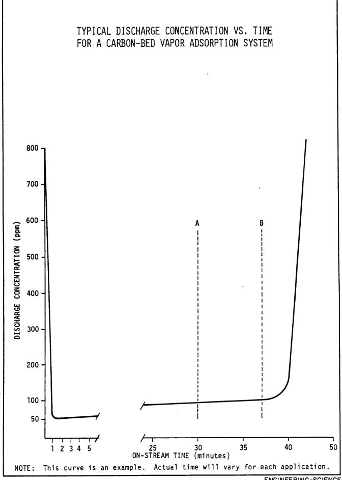
This is not an exact measure of adsorption system capacity, but it can indicate significant deterioration.
