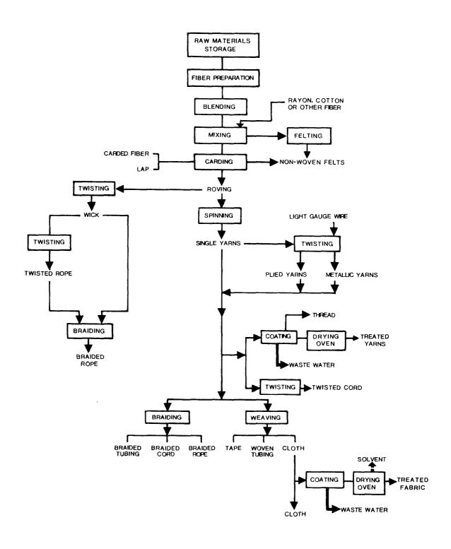
FIGURE 1-ASBESTOS TEXTILE MANUFACTURING OPERATIONS (From handbook of Asbestos Textiles)
