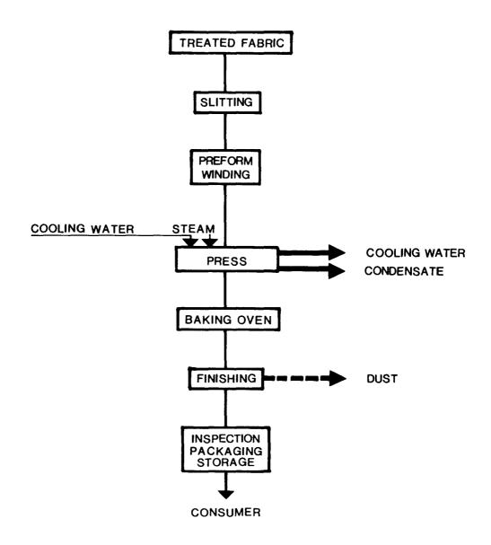
FIGURE 5-WOVEN CLUTCH FACINGS MANUFACTURING OPERATIONS
