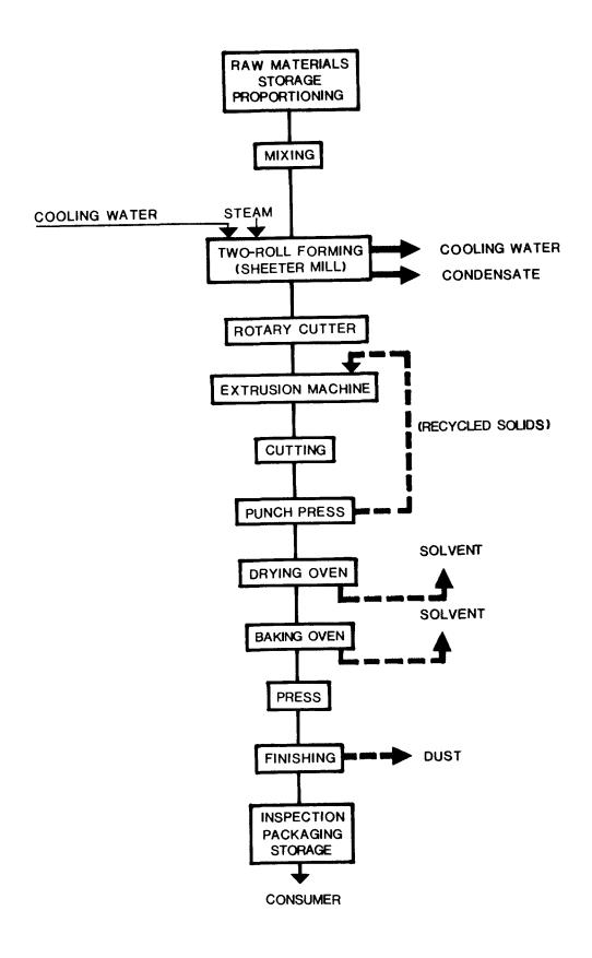
FIGURE 4 - MOLDED CLUTCH FACINGS MANUFACTURING OPERATIONS
