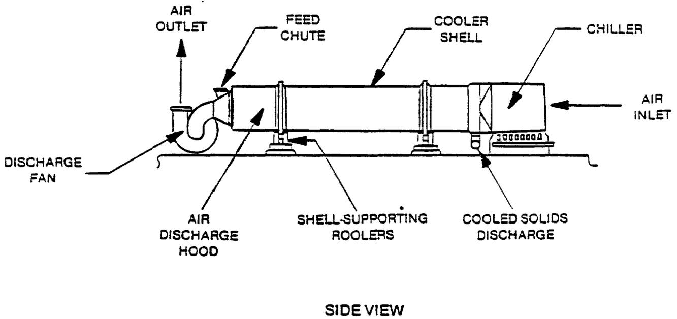
Figure 3-12. Rotary drum cooler.
