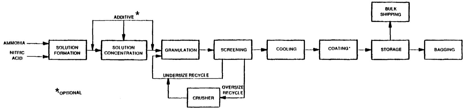
Figure 3-4. Drum granulation or pan granulation process flow diagram.
