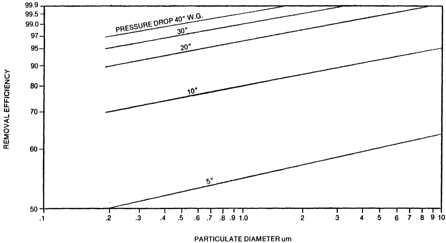
Figure 4-9. Collection efficiency vs. particle diameter for a venturi scrubber.<sup>25</sup>
