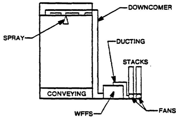
Figure 7-2. Control equipment configuration for low density prill towers - 363 Mg/day (400 TPD).
