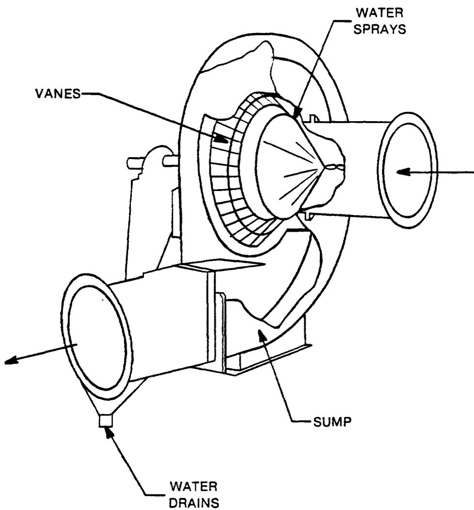
Figure 4-12. Mechanical centrifugal scrubber.<sup>31</sup>
