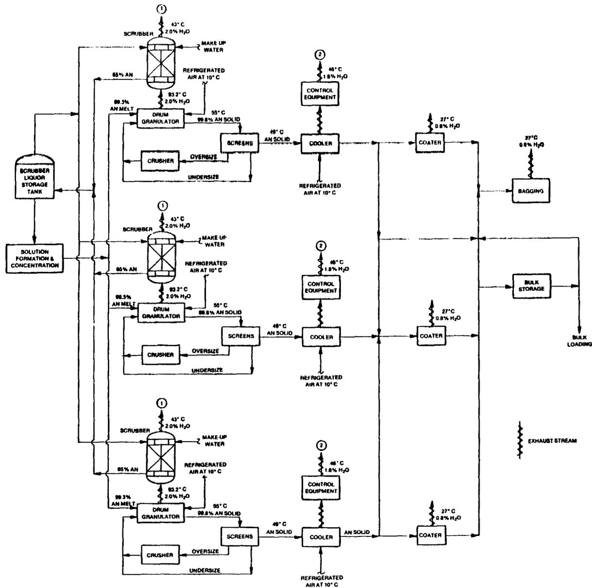
Figure 5-5. 1089 Mg/day (1200 TPD) granulation plant.
