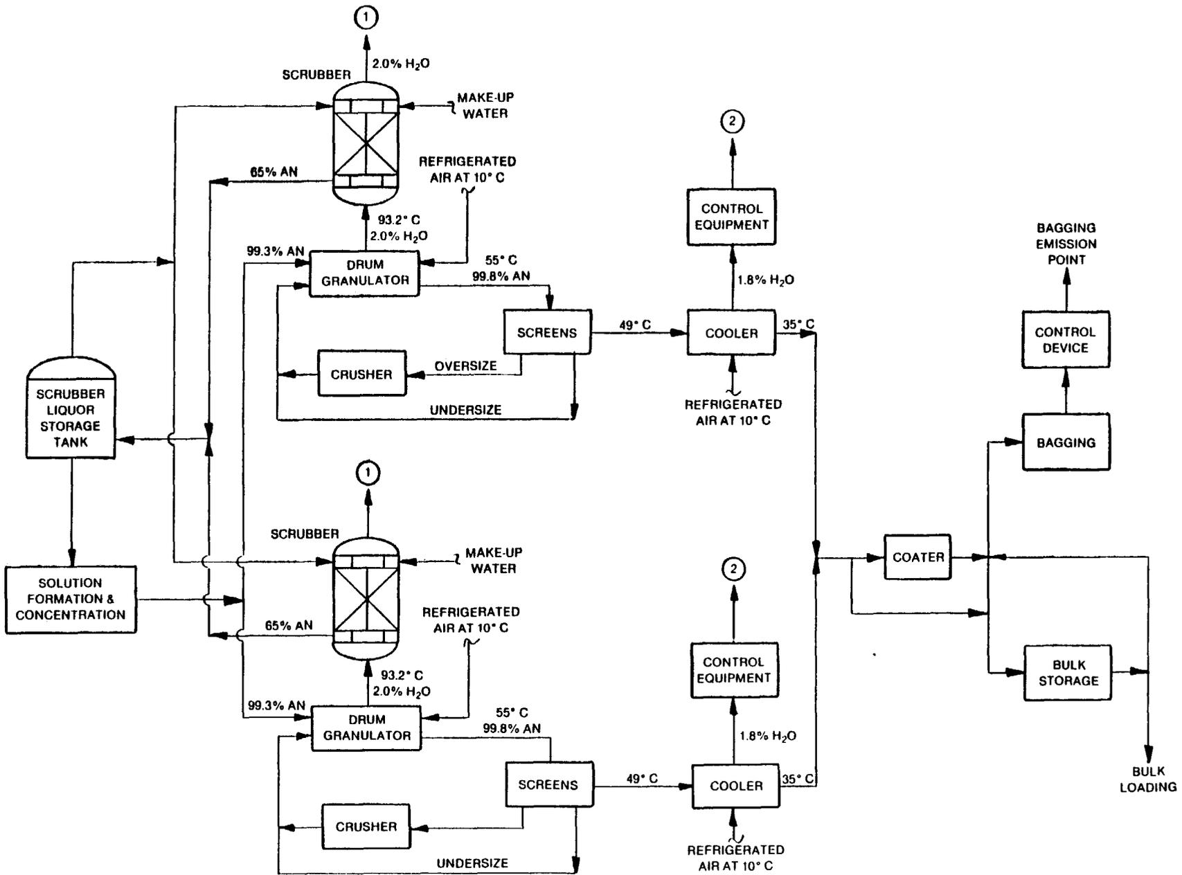
Figure 5-4. 726 Mg/day (800 TPD) granulation plant.
