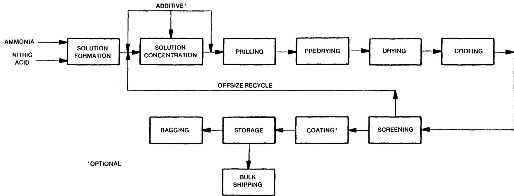
Figure 3-3. Low density ammonium nitrate prilling process flow diagram.
