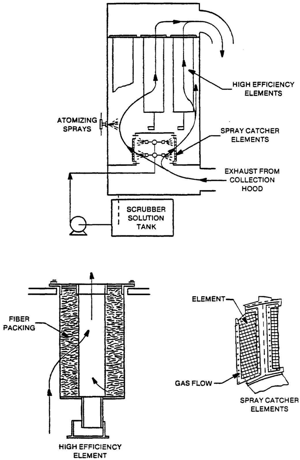
Figure 4-2. Detail of a wetted fibrous filter scrubber.<sup>10,11</sup>
