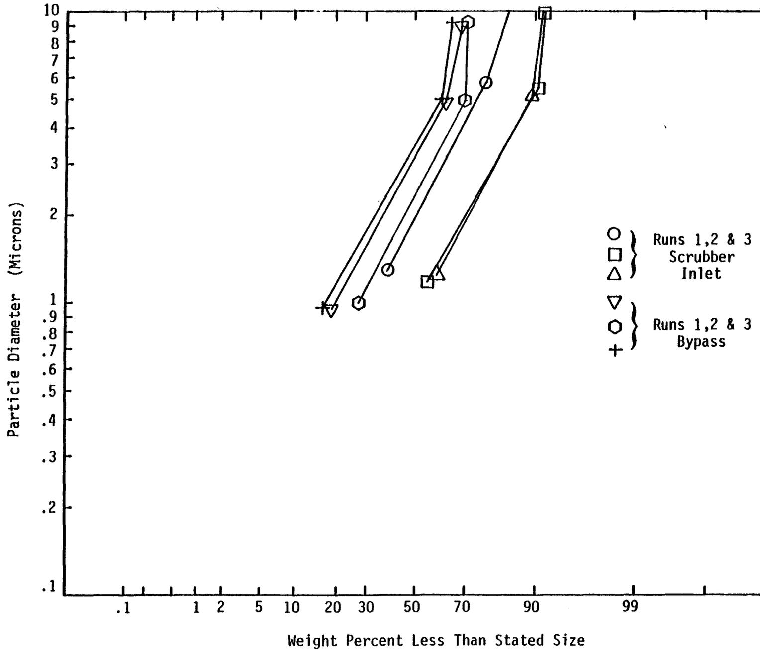
Figure 4-15. Particle size distribution from the bypass and the scrubber inlet at a low density prill tower.
