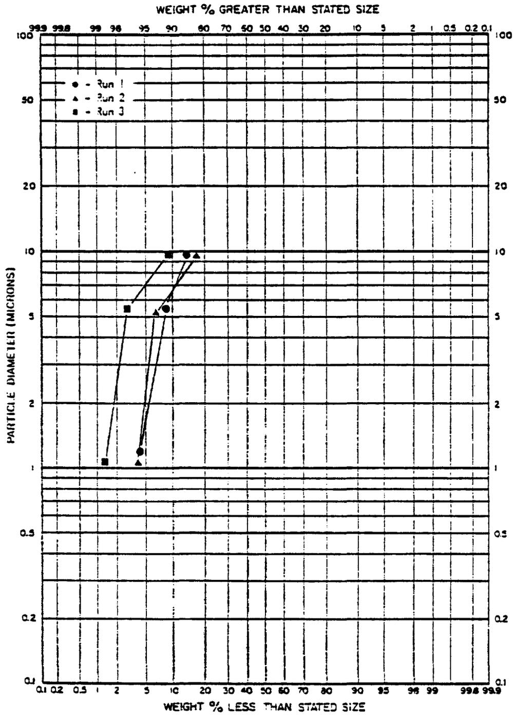
Figure A-14. Plant Z: Particle size results at the fluidized bed cooler bypass.
