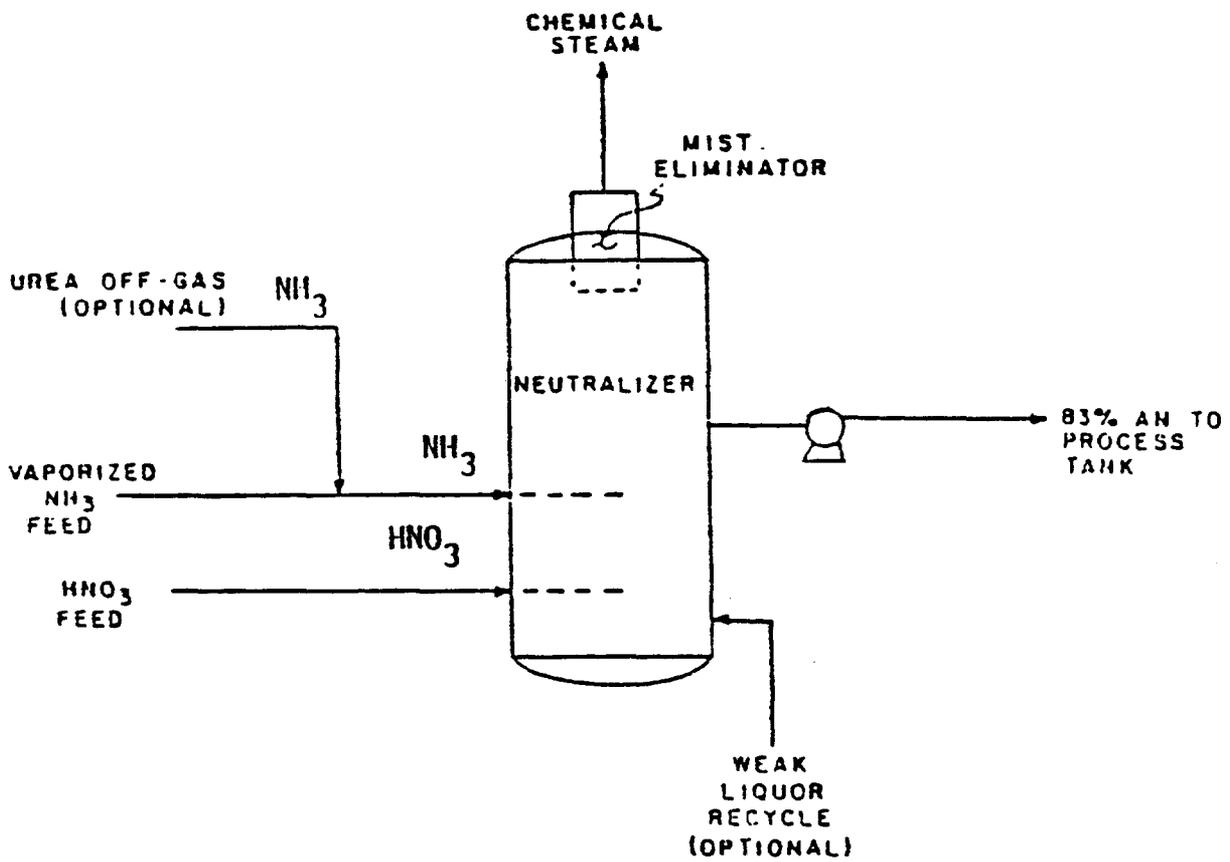
Figure 3-5. Single stage neutralizer.
