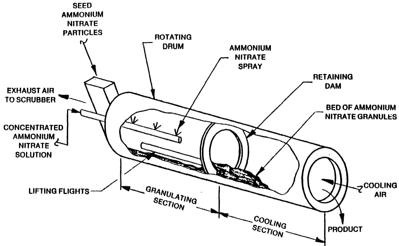
Figure 3-10. Rotary drum granulator.
