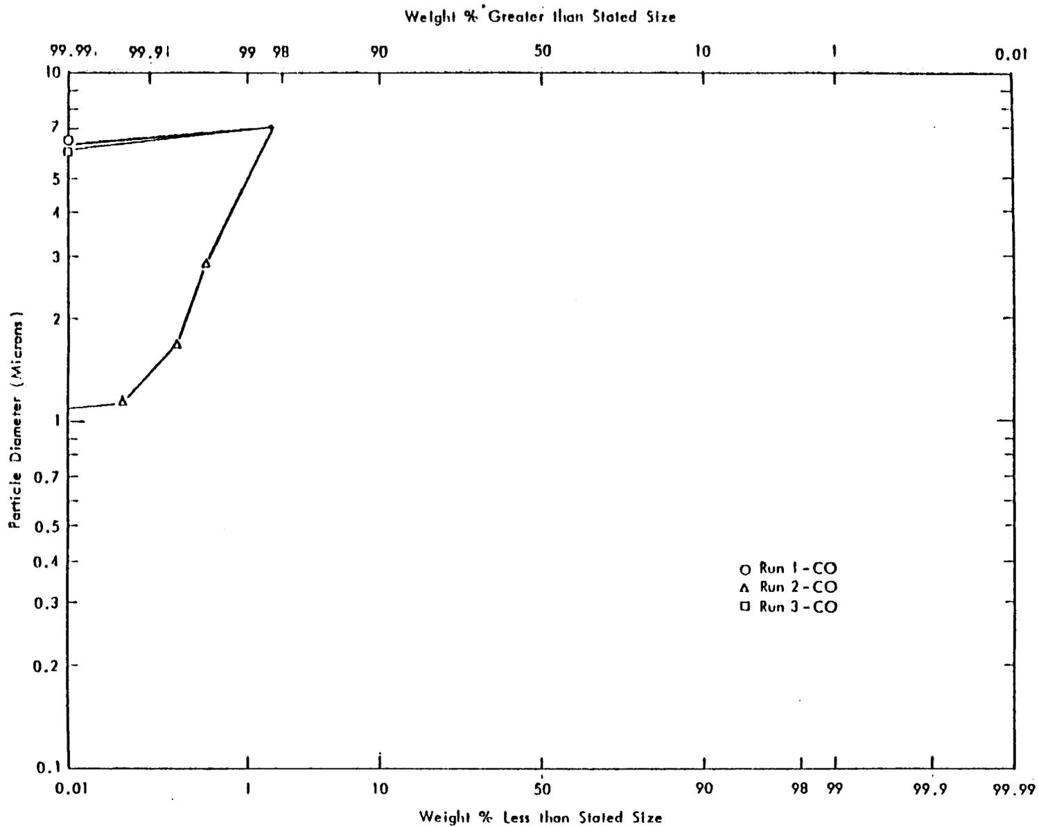
Figure A-2. Plant B: Particle size results at the rotary drum cooler outlet.
