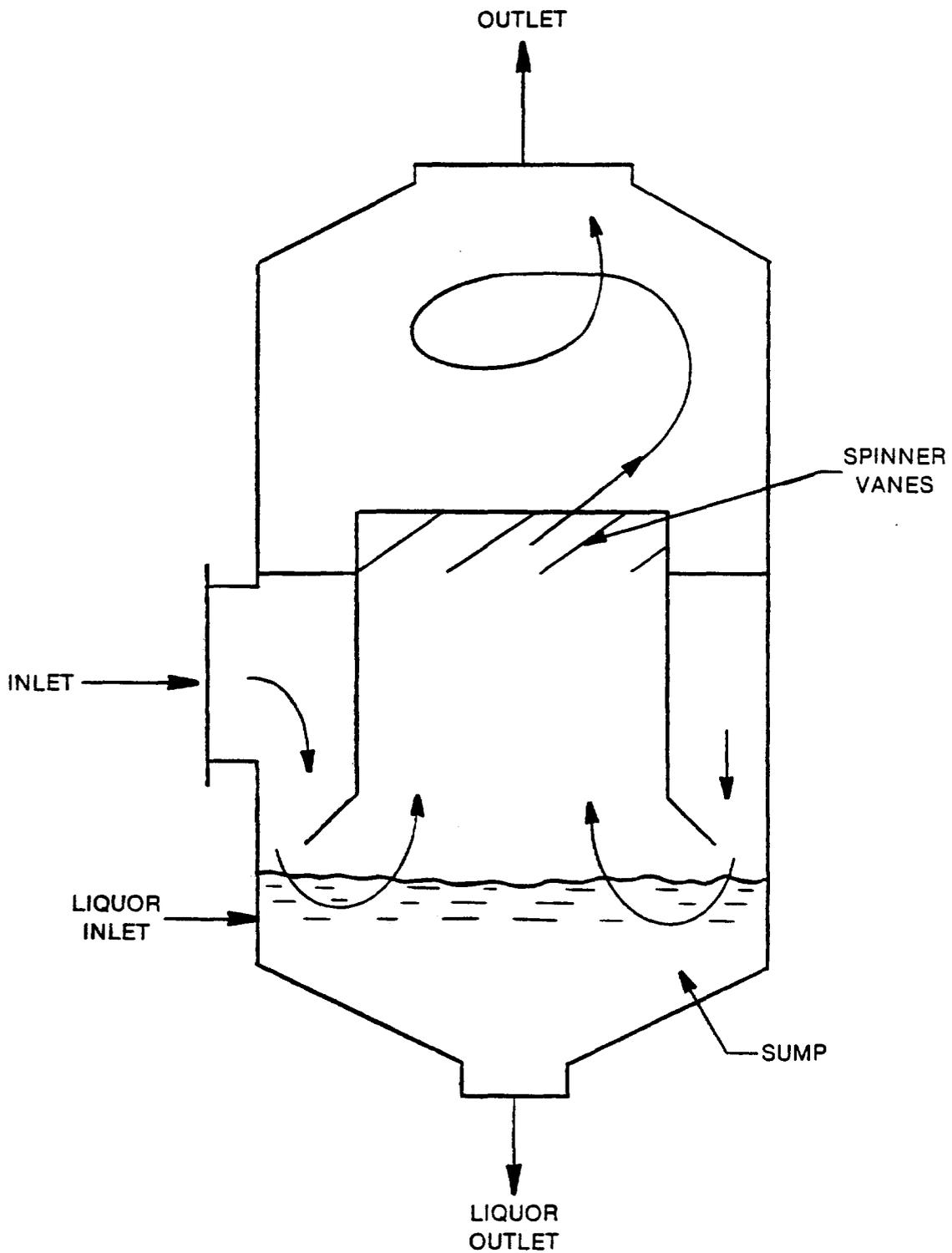
Figure 4-10. Typical entrainment scrubber.<sup>29</sup>
