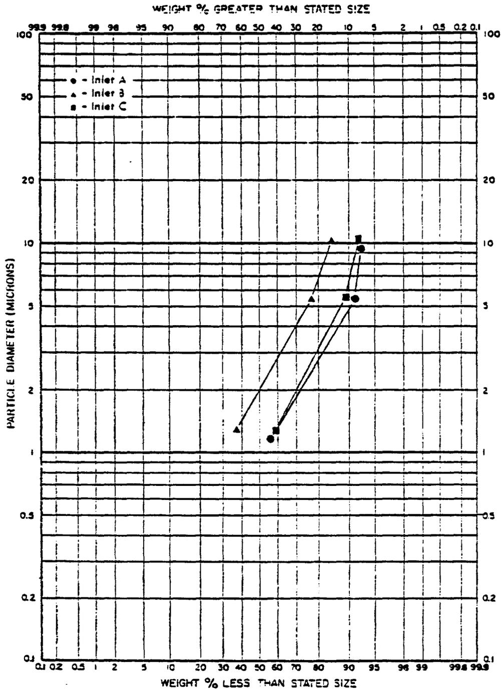
Figure A-9. Plant Z: Particle size results at the prill tower scrubber inlet.
