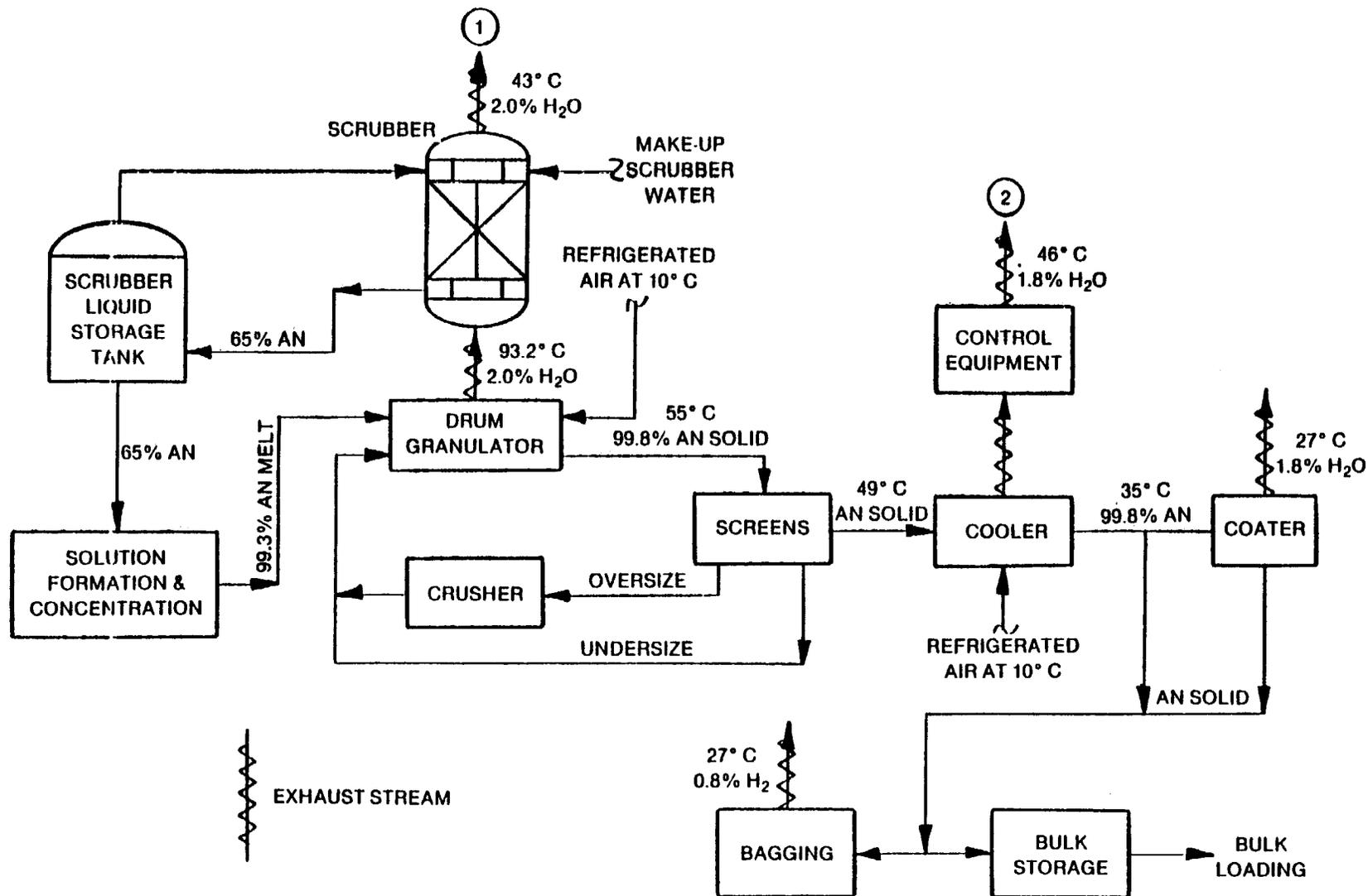
Figure 5-3. 363 Mg/day (400 TPD) granulation plant.
