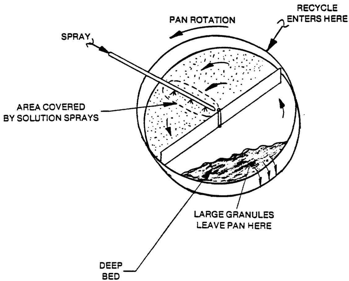
Figure 3-11. Top view of pan granulator.
