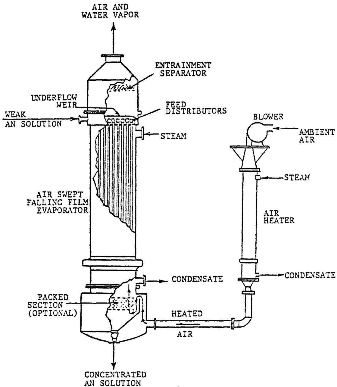
Figure 3-6. Air swept falling film evaporator.
