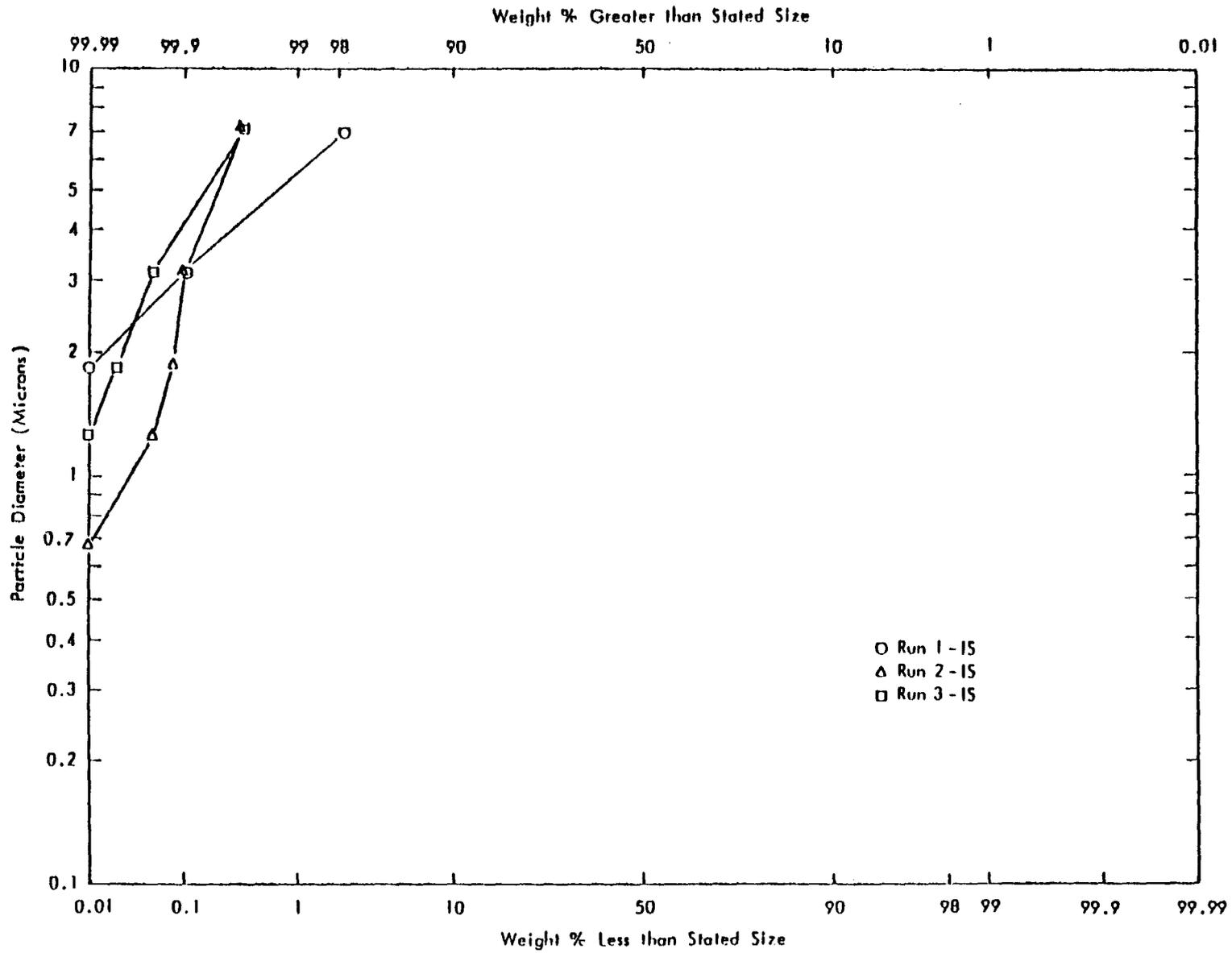
Figure A-1. Plant B: Particle size results at the rotary drum granulator scrubber inlet.
