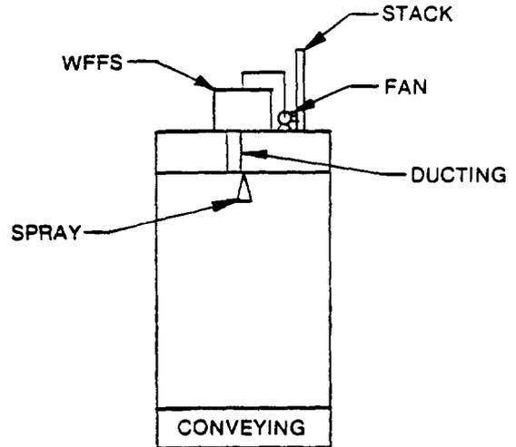
Figure 7-1. Control equipment configuration for high density prill towers - 363 Mg/day (400 TPD).
