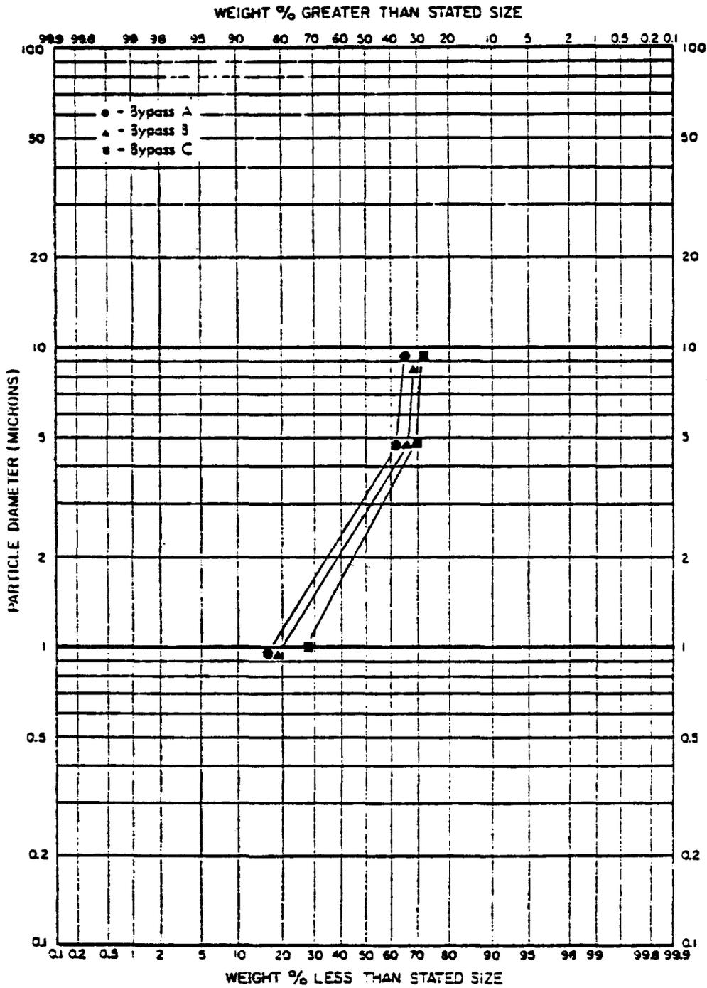
Figure A-10. Plant Z: Particle size results at the prill tower bypass.
