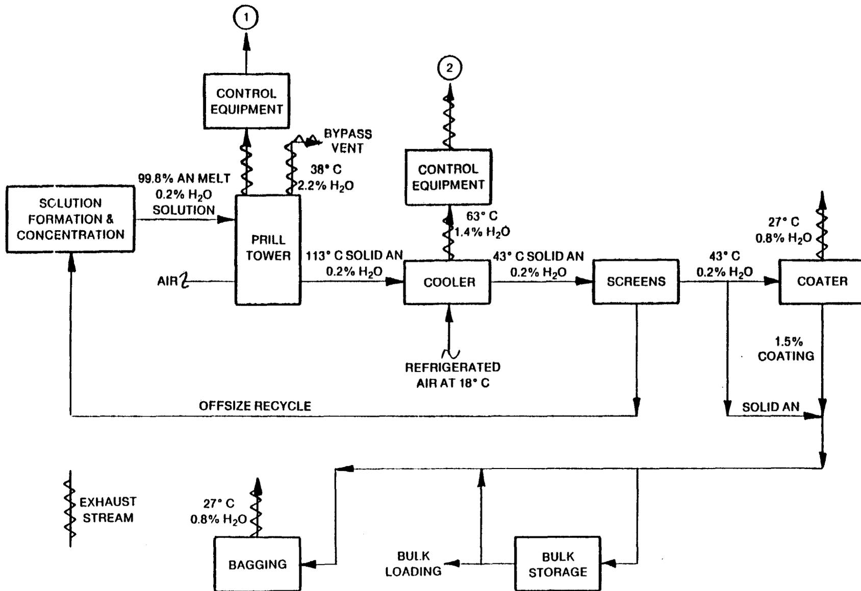
Figure 5-1. High density prill plant.
