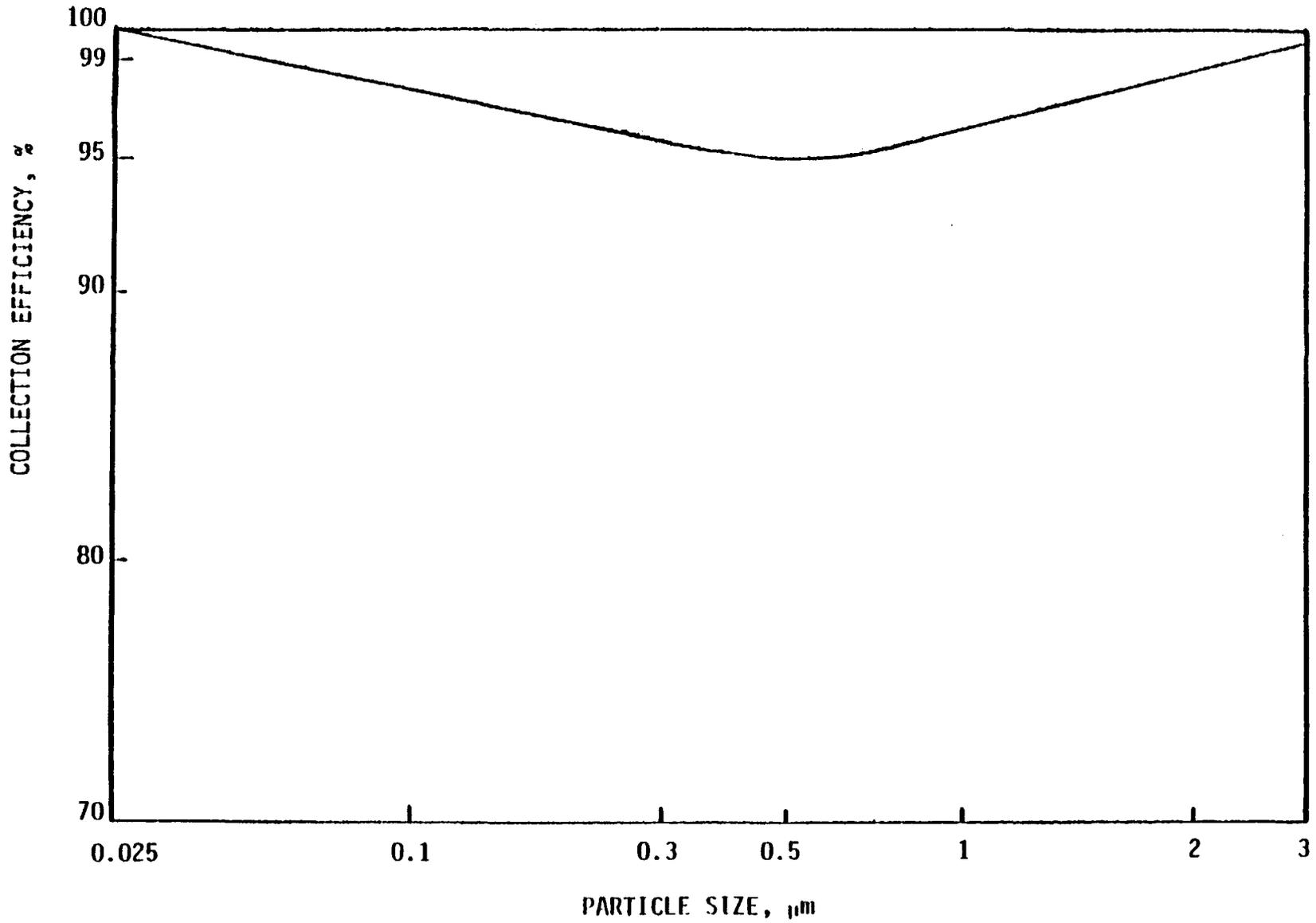
Figure 4-3. Collection efficiency vs. particle size for a wetted fibrous filter scrubber.<sup>14</sup>
