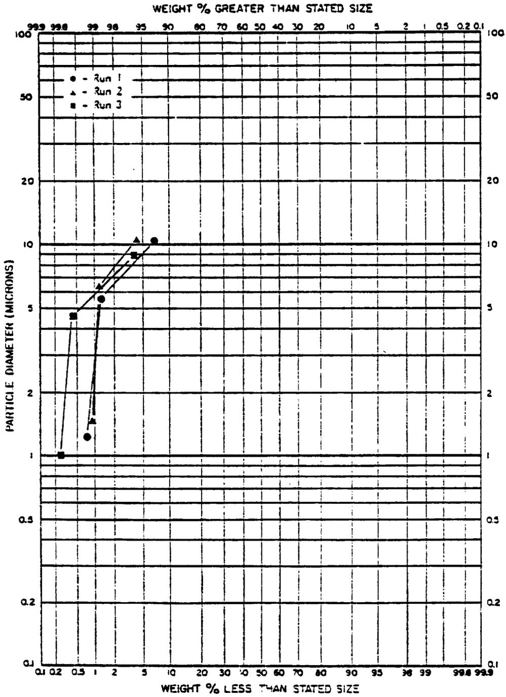
Figure A-12. Plant Z: Particle size results at the dryer outlet.
