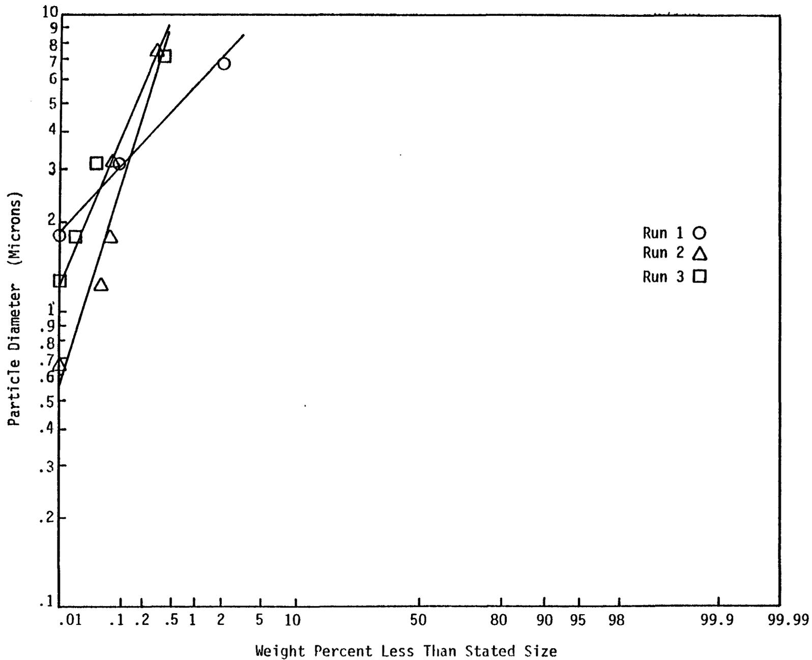
Figure 4-16. Particle size distribution of uncontrolled emissions from a rotary drum granulator.<sup>50</sup>
