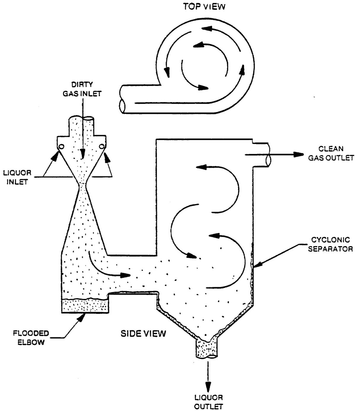
Figure 4-8. Venturi and cyclonic scrubber.
