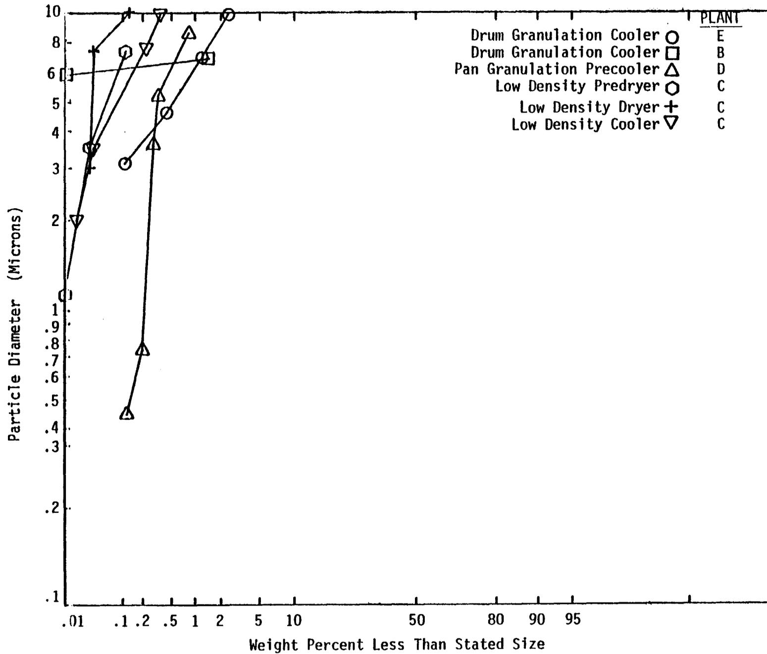
Figure 4-17. Average particle size distribution from solids finishing processes.
