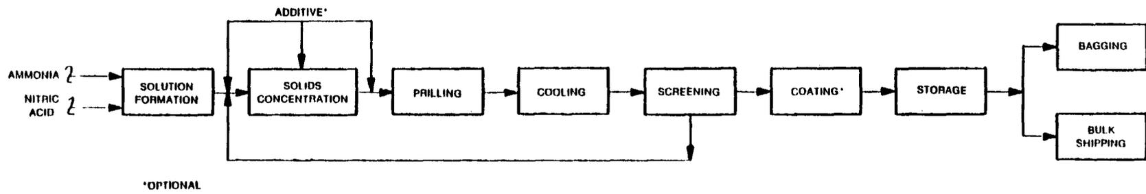
Figure 3-2. High density ammonium nitrate prilling process flow diagram.
