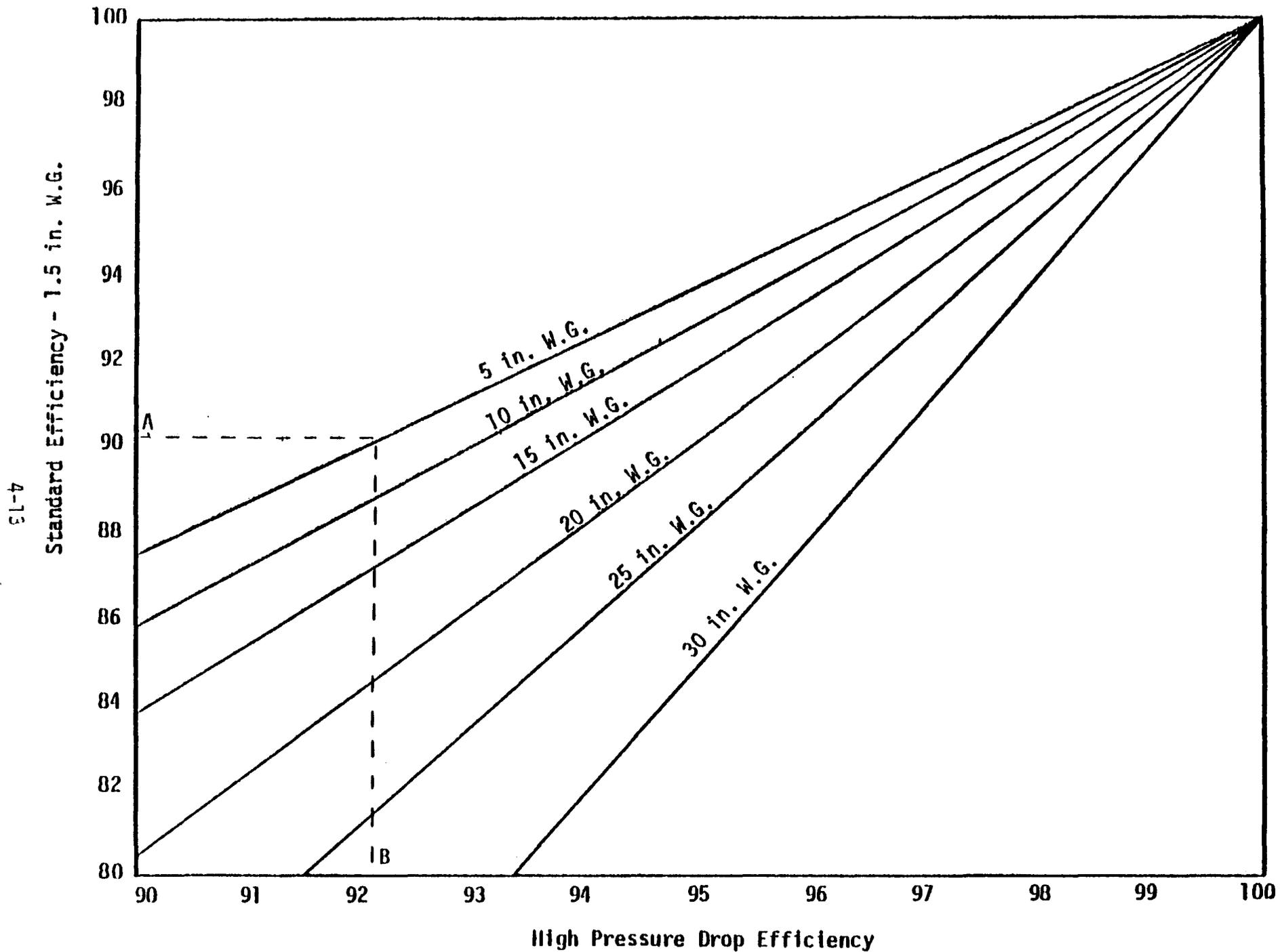
Figure 4-6. Effect of pressure drop on tray-type scrubber efficiency.<sup>16</sup>
