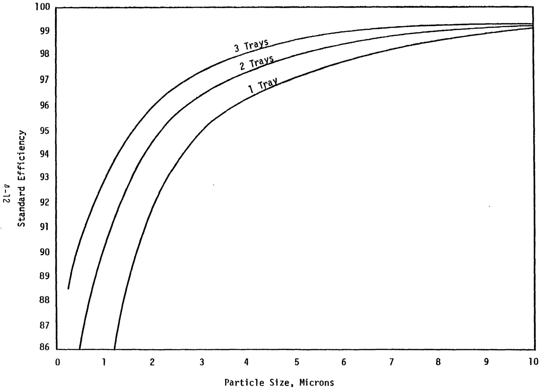
Figure 4-5. Standard fractional efficiency for tray-type scrubber.<sup>16</sup>
