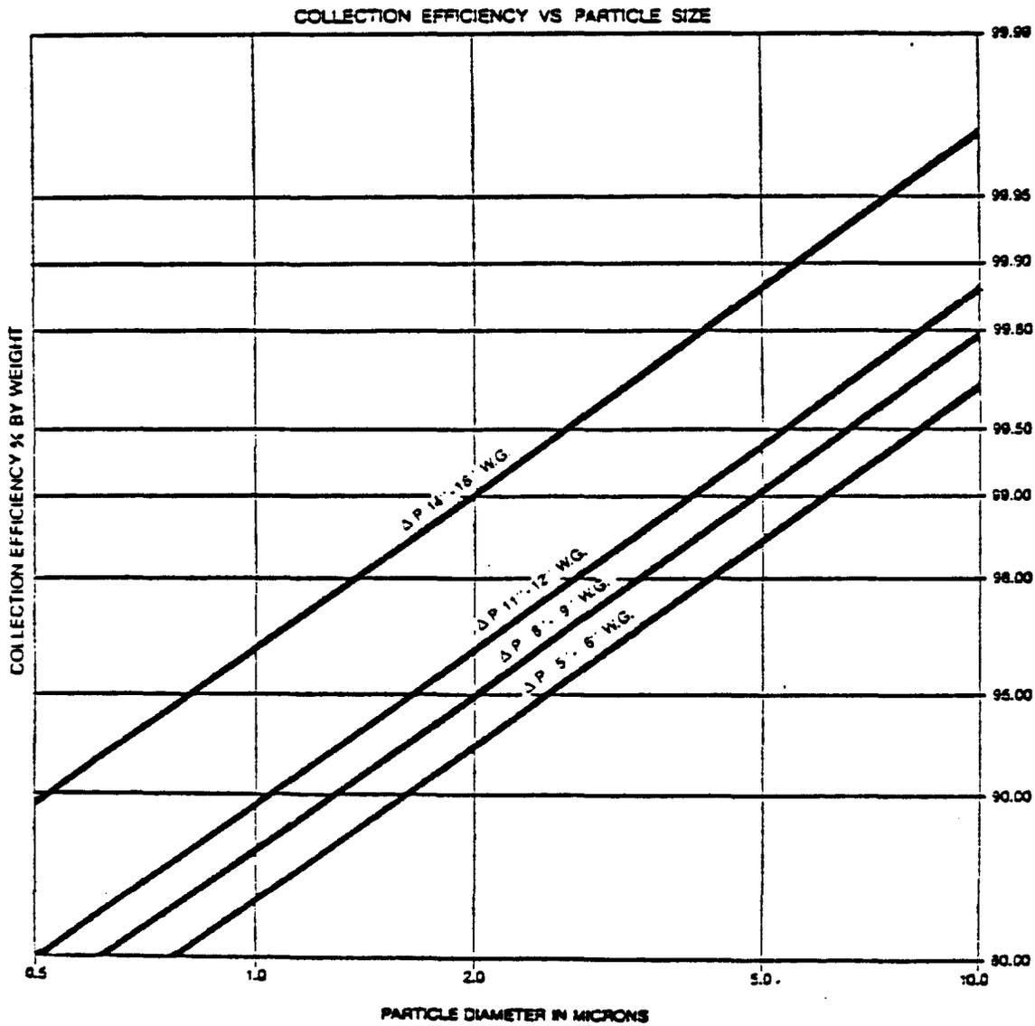
Figure 4-11. Collection efficiency of entrainment scrubbers as a function of particle size and pressure drop (courtesy of the Western Precipitation Division of Joy Manufacturing Company).<sup>27</sup>
