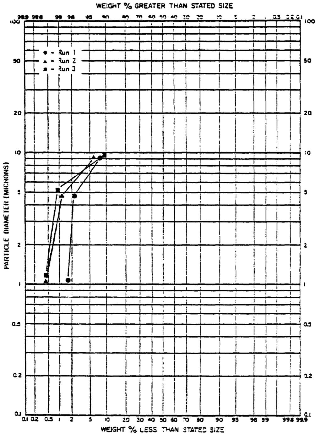
Figure A-11. Plant Z: Particle size results at the predryer outlet.
