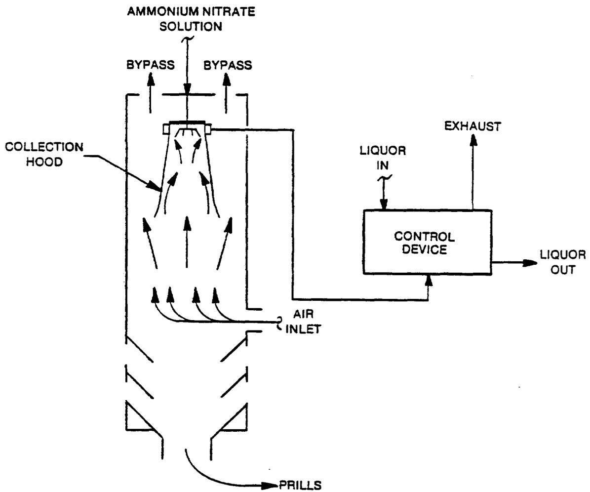
Figure 4-1. Prill tower / collection hood configuration.
