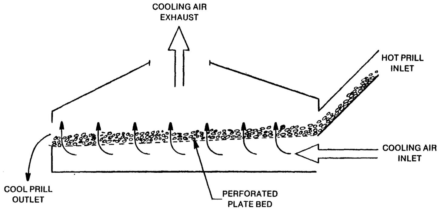
Figure 3-13. Fluidized bed cooler.
