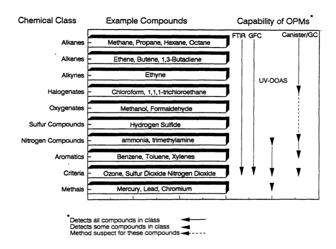
Figure 4-7. Compounds Measurable by Various Methods.
