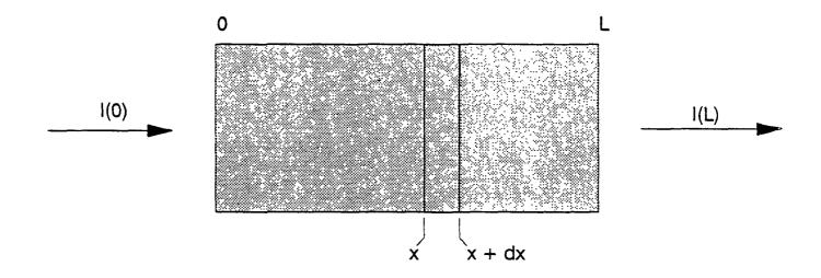
Figure A-1. Light Incident on an Absorbing Medium.
