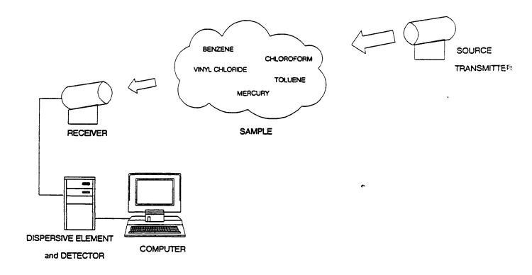
Figure 4-1. Bistatic Configuration of an OPM System.
