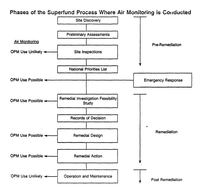
Figure 2-1. Phases of the Superfund Process where Air Monitoring is Conducted.
