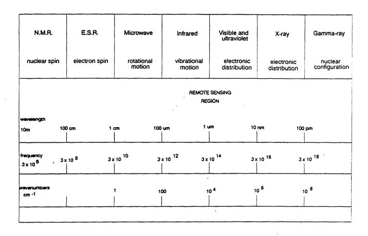
Figure 4-3. Electromagnetic Spectrum.
