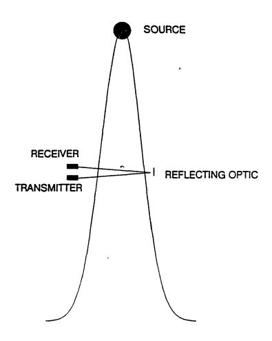
Figure 5-2. Multipassing the Light Beam.
