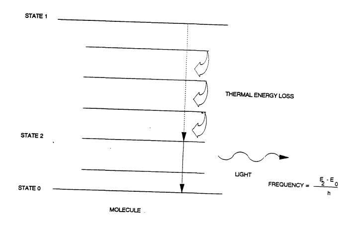
Figure 4-5. Light Emission Process.
