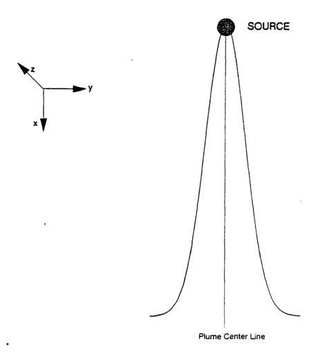
Figure 4-8. Dispersion in the "xy" plane.
