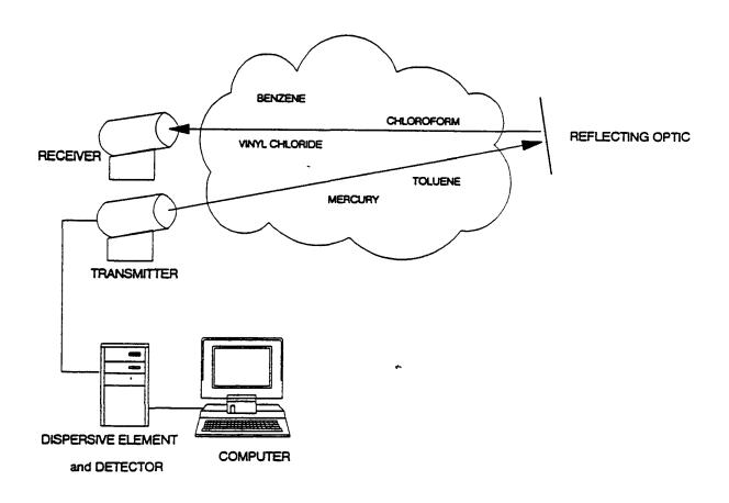
Figure 4-2. Monostatic Configuration of an OPM System.
