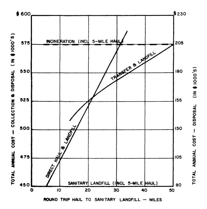
FIGURE 3. EFFECT OF HAUL DISTANCE ON
