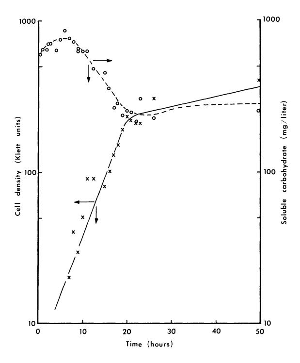
Figure 34. Cell density and soluble carbohydrate concentration versus time for a batch fermentation.
