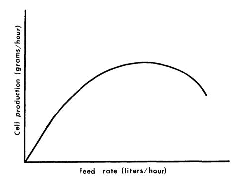
Figure 40. Determination of maximum cell production and optimum feed rate.
