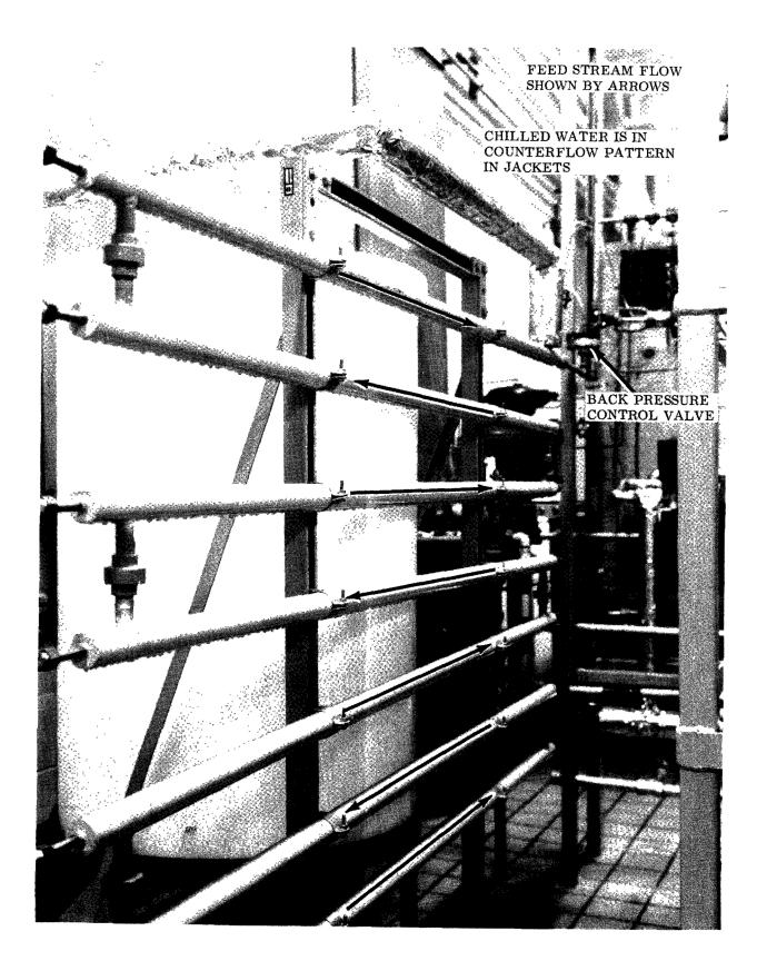
Figure 17. Chilled-water heat exchanger.
