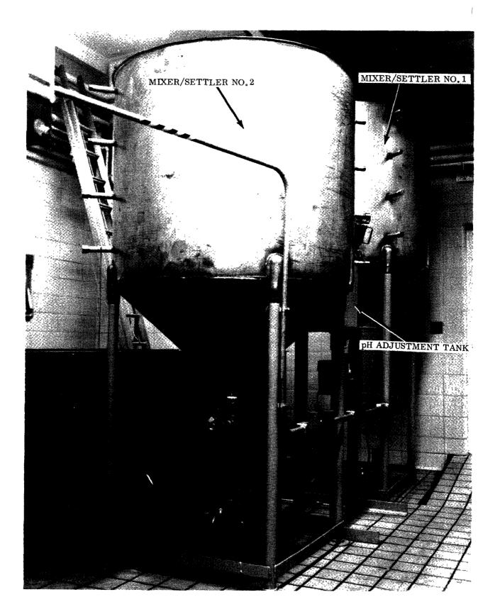
Figure 23. Mixer/settlers and flocculent tank.
