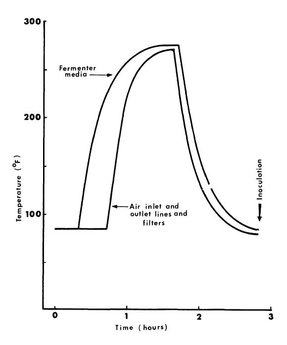
Figure 31. Initial sterilization profile.
