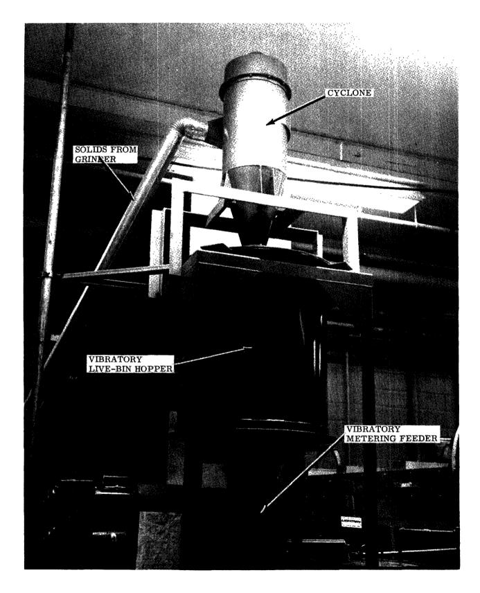
Figure 6. Solids cyclone, hopper, and metering feeder.
