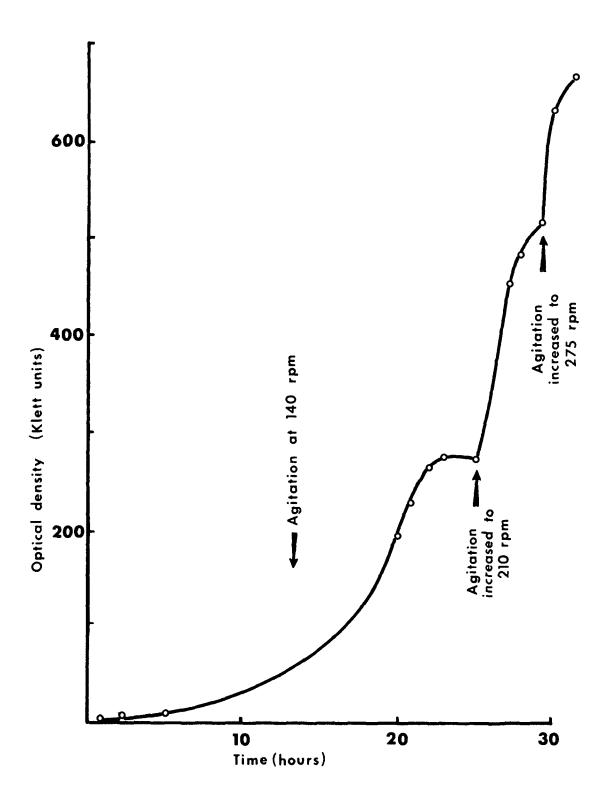
Figure 33. Effect of changing agitation in a batch fermentation.
