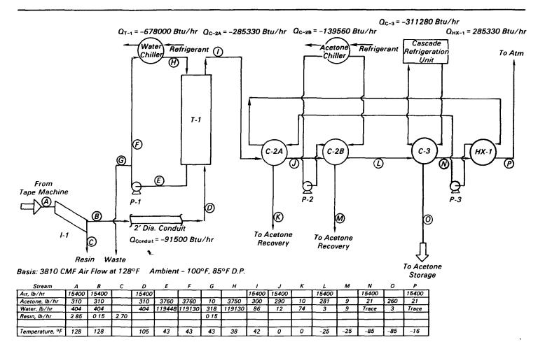
Figure 1. Process flow sheet for Acetone Recovery Project.
