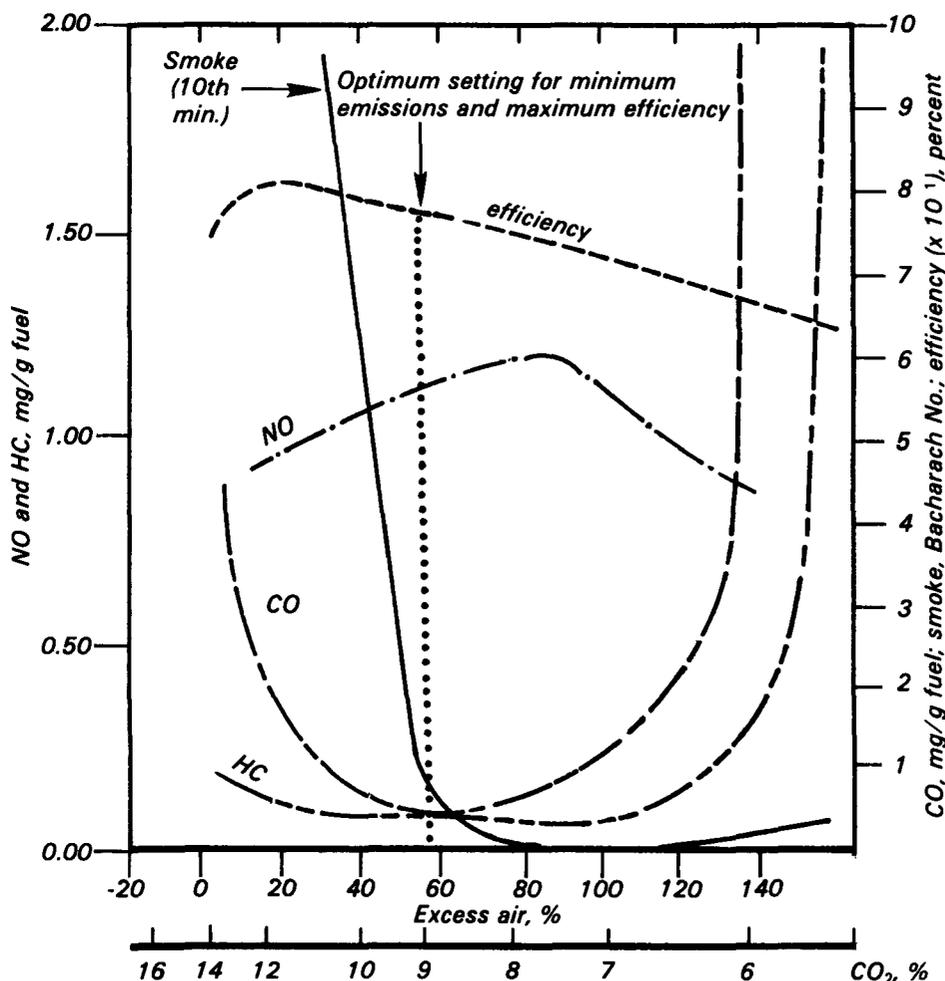
Figure 2. General trend of smoke, gaseous emissions, and efficiency versus stoichiometric ratio for a residential oil burner.
