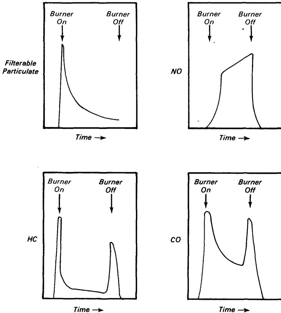
Figure 3. Characteristic emissions of oil burners during one complete cycle.
