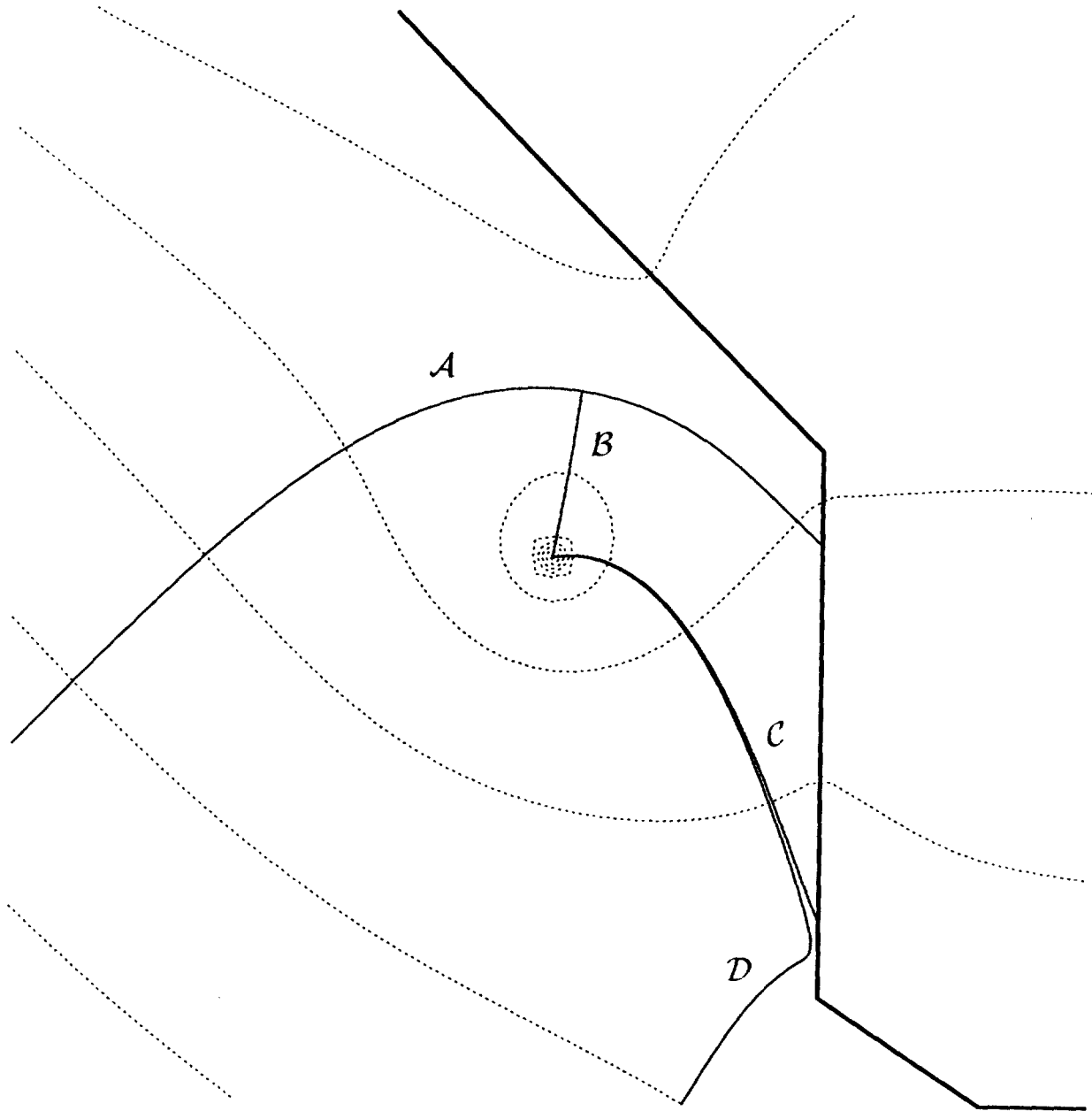
Figure 3.1 Capture zones generated for a well discharge of 1500 \text{ m}^3/\text{day} .
