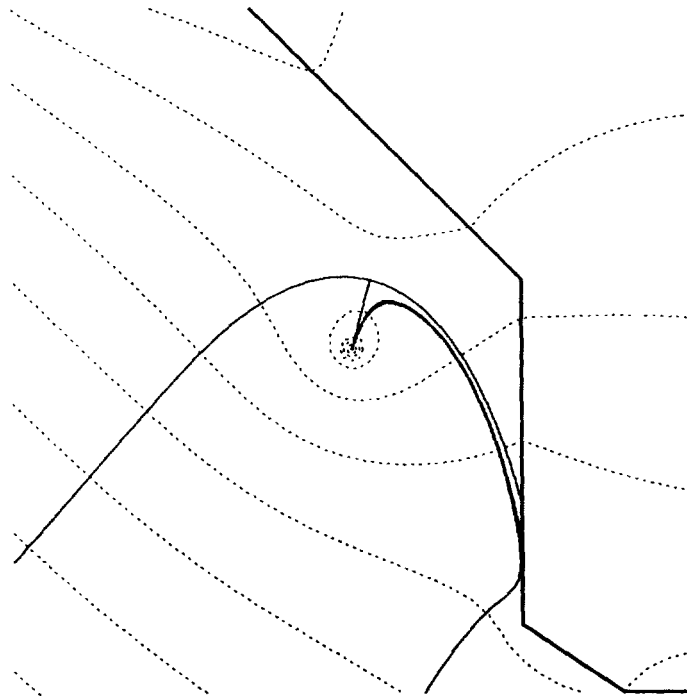
Figure 3.2 Capture zones generated for a well discharge of 1000 \text{ m}^3/\text{day} .
