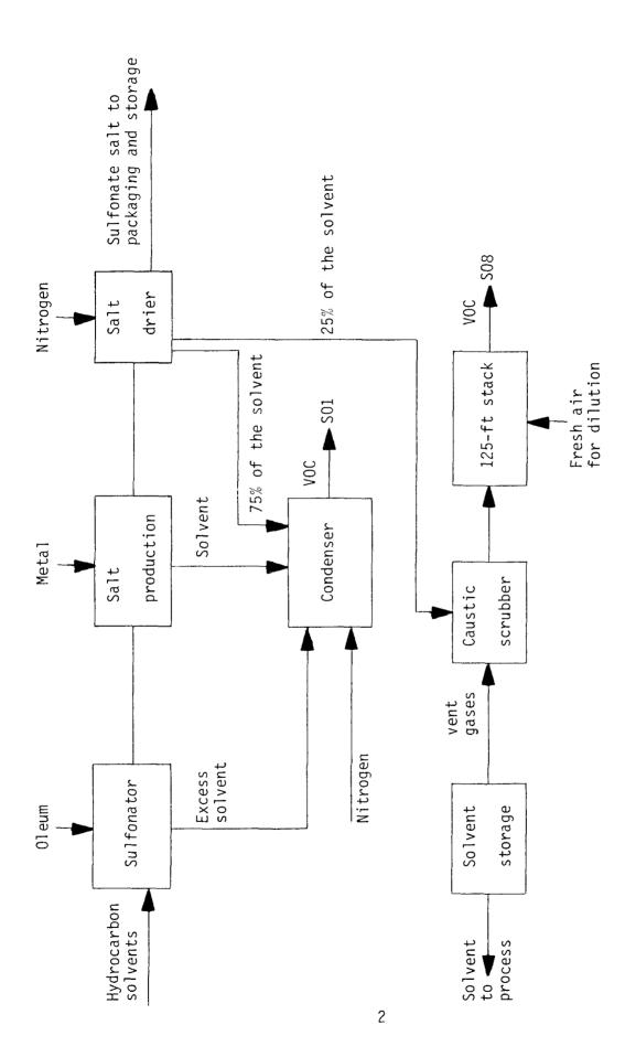
Figure 1. Flow diagram for the Witco plant.
