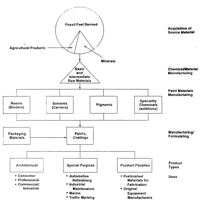
Figure 3-1. Coating industry structure.
