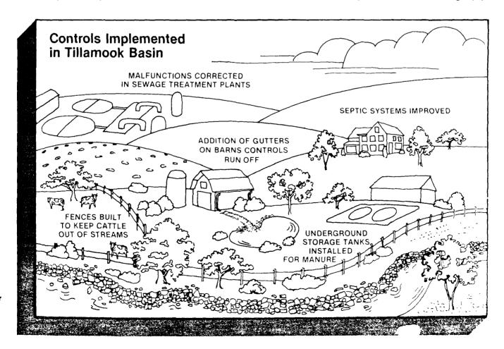
ment problems did occasionally occur. To rectify the problem, alarms and shutdown devices were installed at the sewage treatment plant. The Fecal Waste Management Plan instituted procedures to notify health officials of malfunctions so that shellfish beds could be closed. In addition, many failing septic systems have been eliminated as a pollution source by the expansion of a municipal sewer line.
