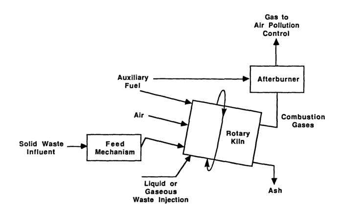
Figure 4-12 Rotary Kiln Incinerator
