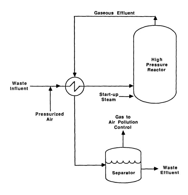
Figure 4-15 Wet Air Oxidation
