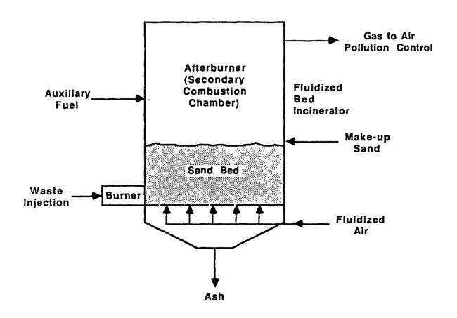
Figure 4-13 Fluidized Bed Incinerator
