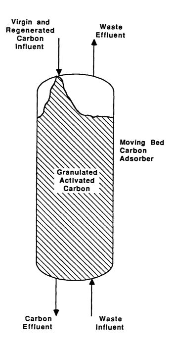
Figure 4-2 Moving Bed Carbon Adsorption
