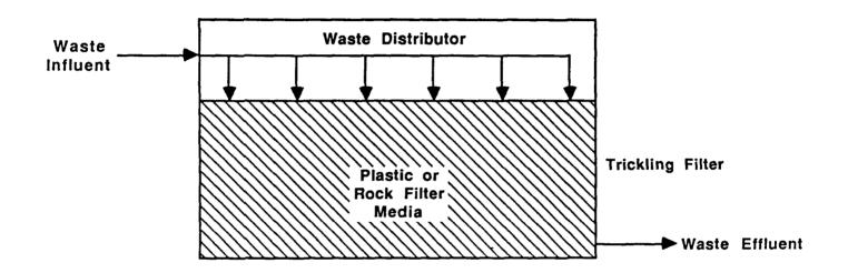
Figure 4-9 Trickling Filter
