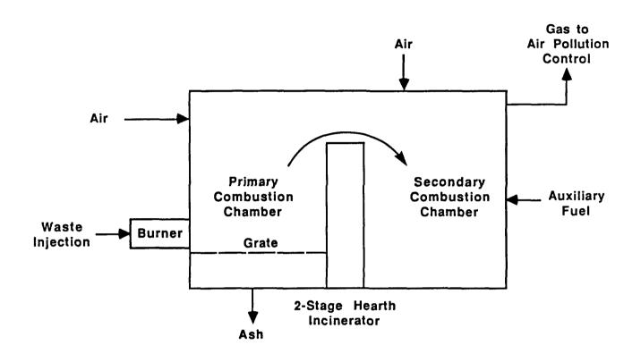
Figure 4-14 Hearth Incinerator
