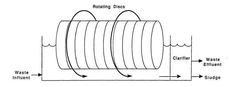
Figure 4-10 Rotating Biological Contactor
