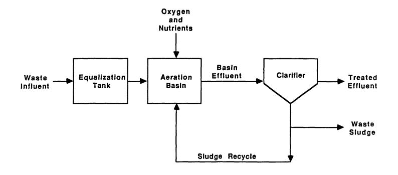
Figure 4-8 Activated Sludge
