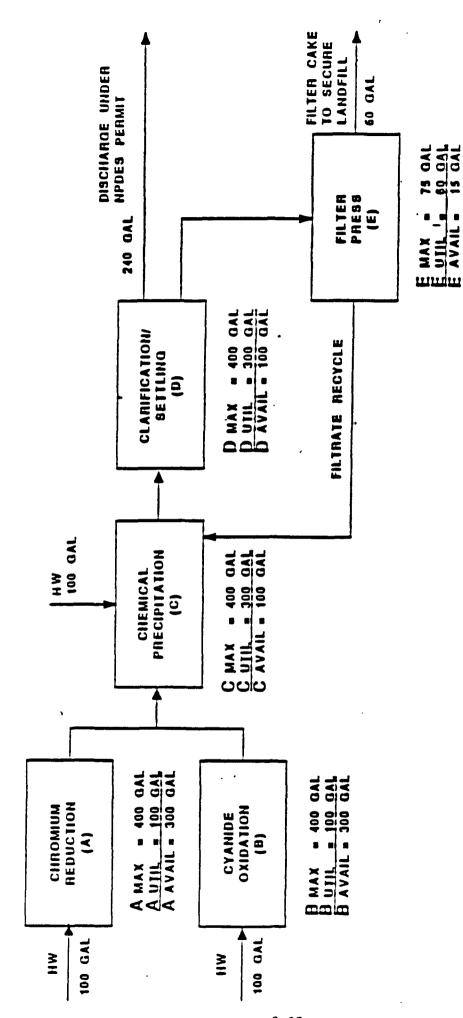
FLOW DIAGRAM OF THREE SYSTEMS WITH UNIT PROCESS CAPACITIES Figure 3-3
