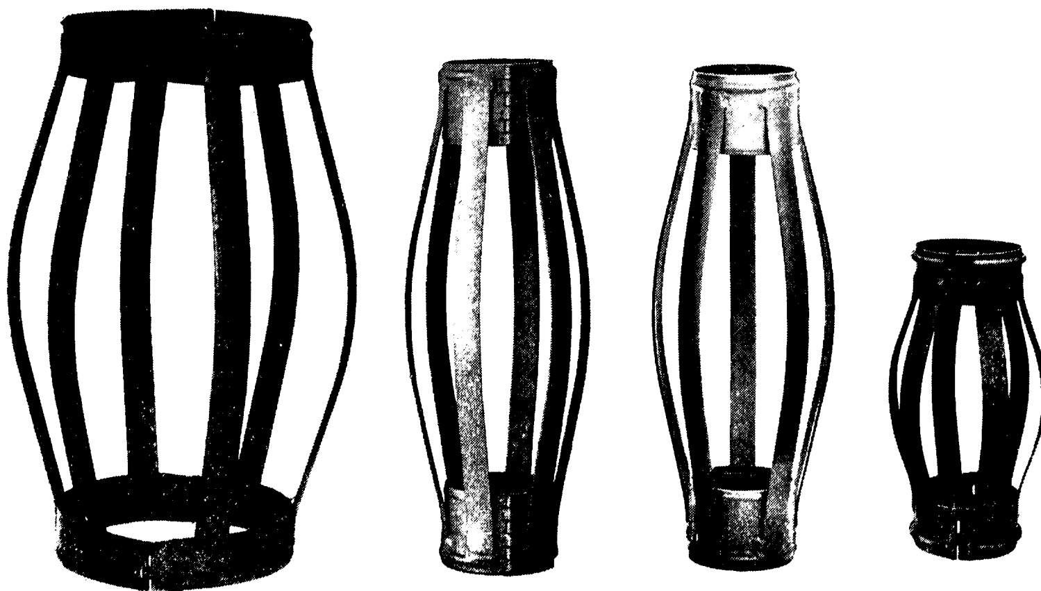
FIGURE 7-10. TYPES OF CASING CENTRALIZERS (SMITH, 1976).
