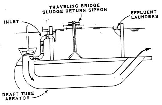
Figure 5. INNOVA-TECH, Inc. Pumpless Integral Clarifier (5).
