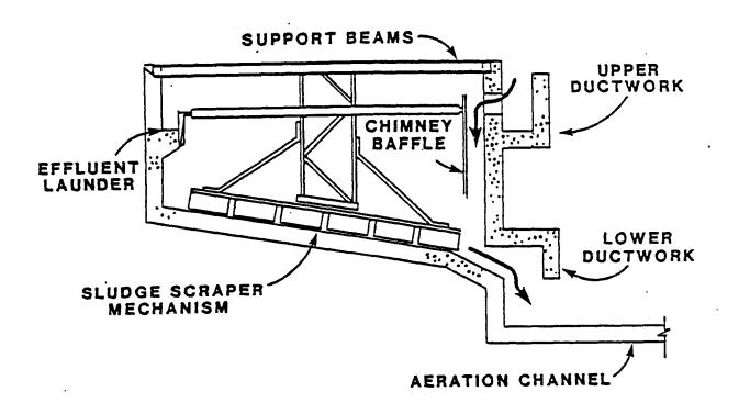
Figure 7. Mixing Equipment Co. Lightnin Integral Clarifier (7).
