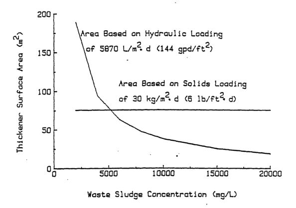
Figure 10. Impact of Waste Sludge Concentration on Size of Sludge Handling Facilities for Example Plant.
