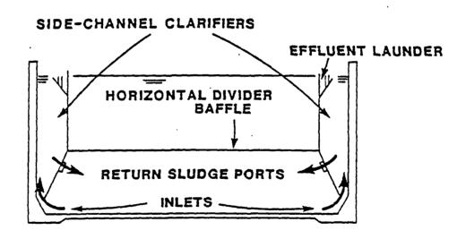
Figure 4. Envirex, Inc. Side-Channel Clarifier in a Vertical Loop Reactor (4).
