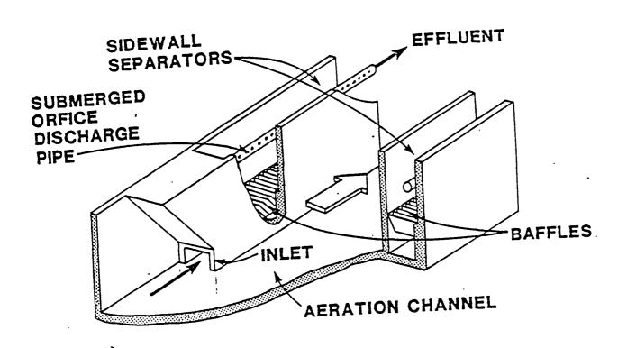
Figure 6. Lakeside Equipment Corp. Sidewall Separator (6).
