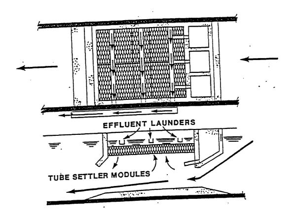
Figure 8. SYDLO, Inc. Integral Clarifier/Oxidation Ditch System (8).
