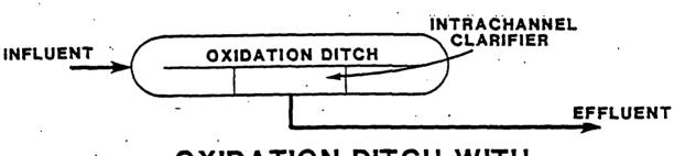
OXIDATION DITCH WITH INTRACHANNEL CLARIFIER
