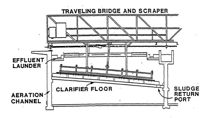
Figure 3. EIMCO Process Equipment Co. Carrousel Intraclarifier (3).
