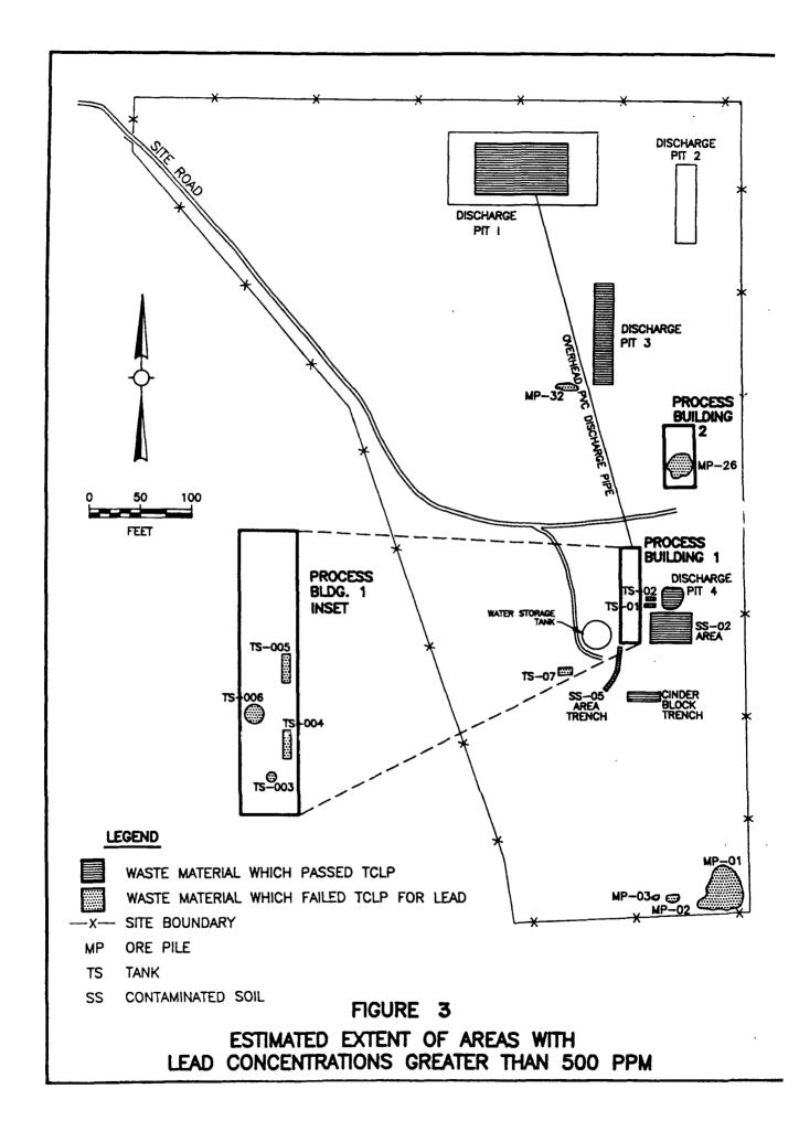
tank sediments, where the majority of samples indicate high elevated concentrations of lead, only four of the 34 waste pile samples analyzed indicate contamination with lead at levels in excess of the 500-1000 ppm guidance levels. Two piles, MP-01 and MP-26, with lead concentrations of 18,900 ppm and 18,700 ppm, respectively, are the only piles that demonstrate significantly elevated lead levels. All other waste pile samples contain lead at concentrations of 114 ppm or less.
