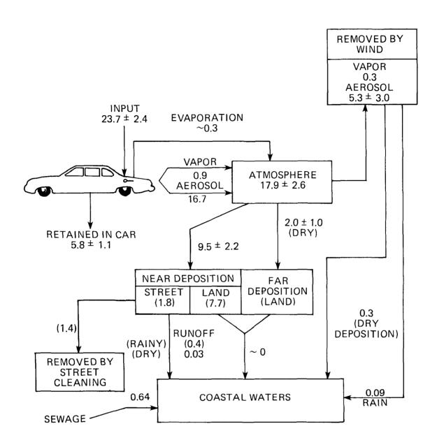
FIGURE 2-2. THE FLOW OF AUTOMOBILE EMITTED LEAD THROUGH THE LOS ANGELES BASIN. (With the exception of far deposition and wind removal fluxes, which are for dry weather only, the values are daily averages calculated by dividing the yearly totals by 365. All fluxes are in metric tons/day. Numbers in parentheses are model-dependent and in need of a more extensive data base. From Huntzicker et al. 1975a).
