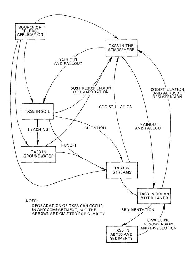
FIGURE 5-3. PATHWAYS FOR TOXIC SUBSTANCES (TXSB) IN THE PHYSICOCHEMICAL ENVIRONMENT SYSTEM (from Eschenroeder et al. 1978).
