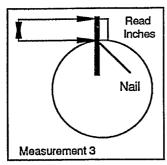
Measurement 3 is the distance from the bottom of the fitting to the the top of the riser pipe. This measurement is taken by using a tape measure or by driving a nail into the 1" point at a right angle to the dipstick.
