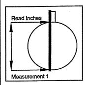
**Measurement 1** is the inside diameter of the tank at a fitting opening. Measure from the bottom of the tank to the bottom of the fitting. This measurement should be taken prior to placing any backfill.
