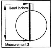
**Measurement 2** is the distance from the bottom of the tank to the top of the riser pipe. Backfill should be to subgrade at this time.
