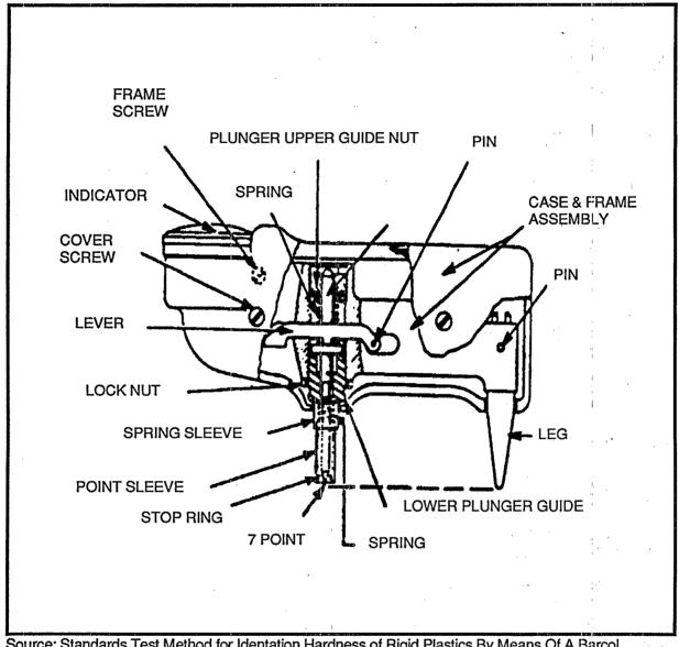
Source: Standards Test Method for Identation Hardness of Rigid Plastics By Means Of A Barcol Impressor. ASTM D2583-87. Reprinted with permission.
