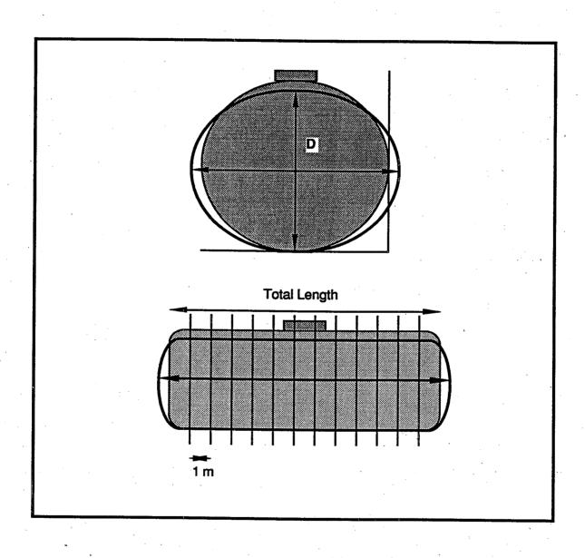
Figure 6. Two Drawings Showing Exaggerated Elliptical Deflection in Cross-Section
