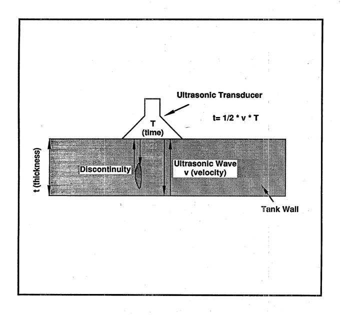
Figure 1. Example of Wave Activity Through Tank Wall Using Ultrasonic Test
