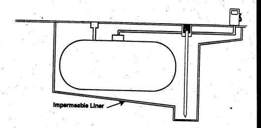
Monitoring wells can provide leak detection for tanks and distribution lines where secondary containment liners are used.
