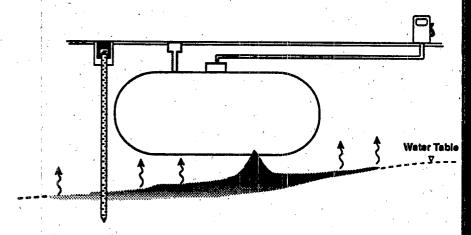
The vapor monitor will detect hydrocarbon gases in the soil air collected from above the water table. The liquid monitor will detect hydrocarbons floating on the water table.
