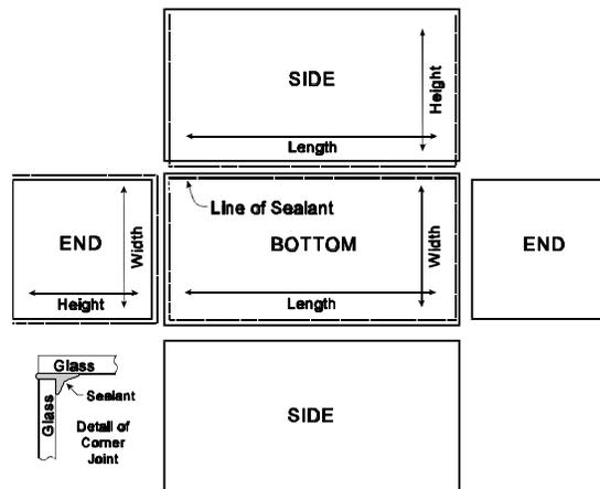
Figure 4-2. Schematic of aquarium construction.
