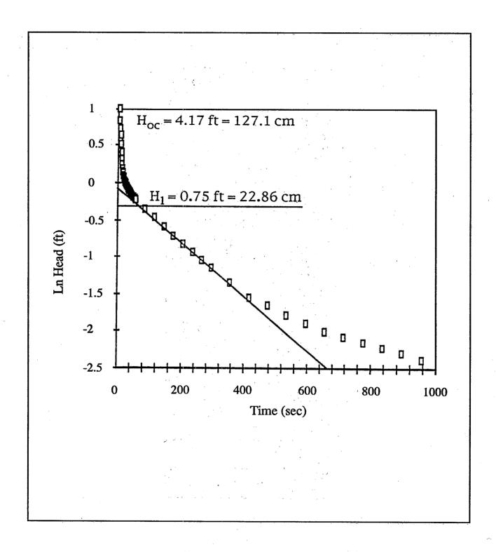
Figure 27. Determination of the transition point (H<sub>i</sub>) on the recovery curve of a typical monitoring well with a partially submerged screen exhibiting filter sand pack drainage in early time.
