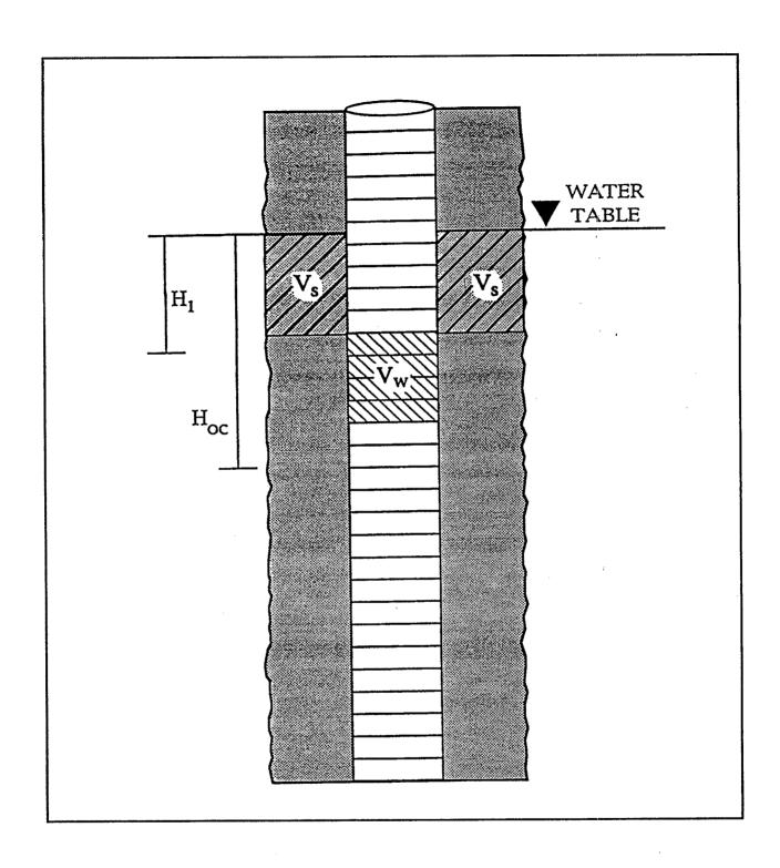
Figure 28. Illustration of parameters used to estimate the specific yield of the filter sand pack from early time recovery data.
