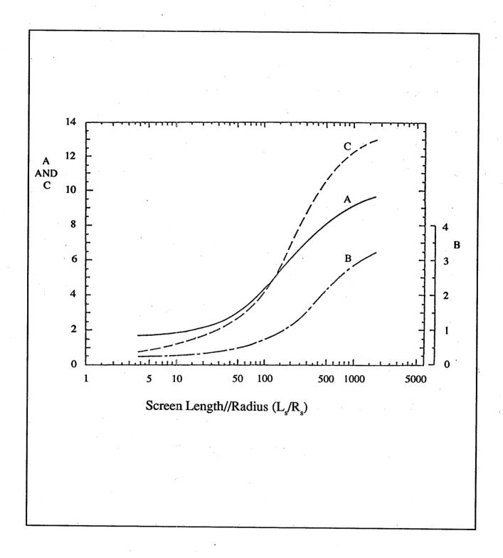
Figure 13. Dimensionless parameters A, B, and C for the Bouwer and Rice (1976) model.
