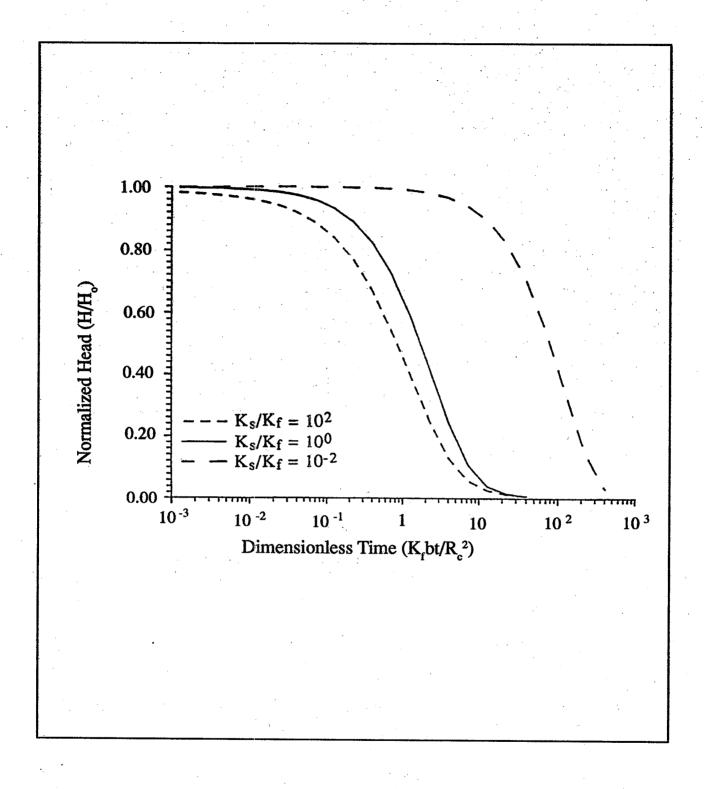
Figure 19. Effects of borehole skin on recovery curves for a fully penetrating well in a confined aquifer. K and K, are the skin and formation conductivities, respectively. After McElwee et al., 1990.
