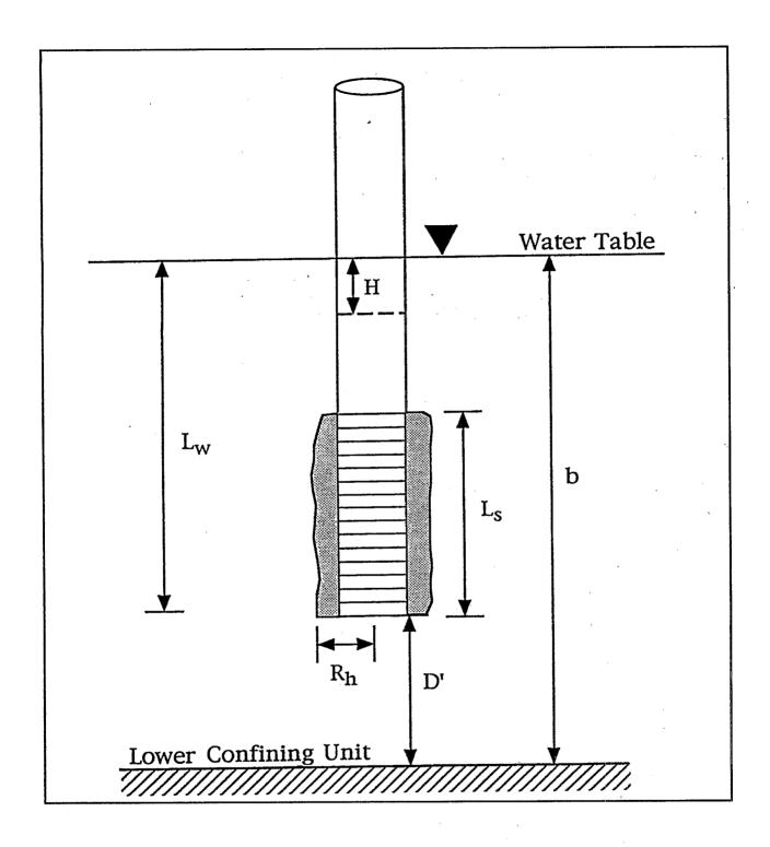
Figure 12. Well and aquifer geometry symbols for the Bouwer and Rice (1976) model.
