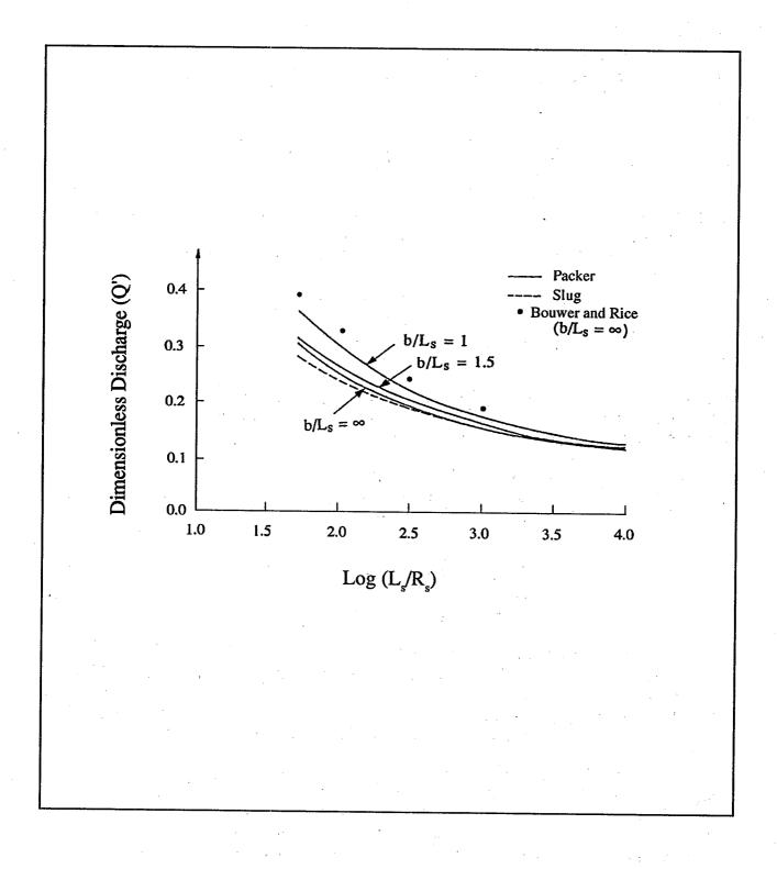
Figure 6. Comparison of dimensionless discharge (Q') curves for different slug test models. b = aquifer thickness,  $R_a = well$  screen radius, and  $L_a = well$  screen length. After Dagan, 1978.
