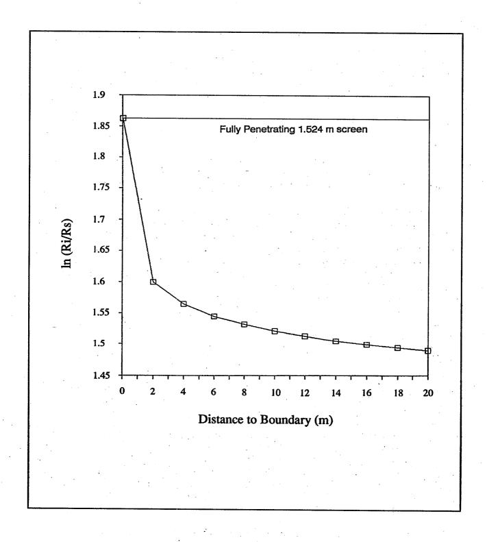
Figure 24. Effects of partial penetration on the ln(R/R) term as a function of the distance to a lower impermeable boundary (D') for a 11.43 cm radius, 1.524 meter long, well screen. Using method of Bouwer and Rice, 1976.
