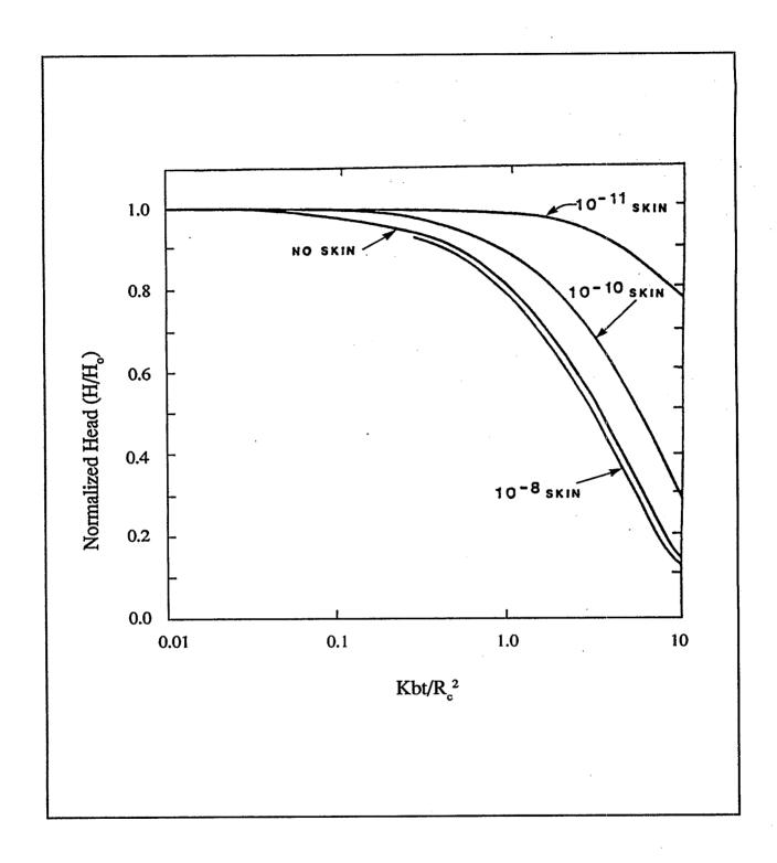
Figure 16. Recovery curves for varying skin hydraulic conductivities. Numbers adjacent to curves represent skin conductivities in m/s. K = formation hydraulic conductivity, b = aquifer thickness, t = time,  $R_o =$  well casing radius, and  $H/H_o =$  normalized head. After Faust and Mercer, 1984.
