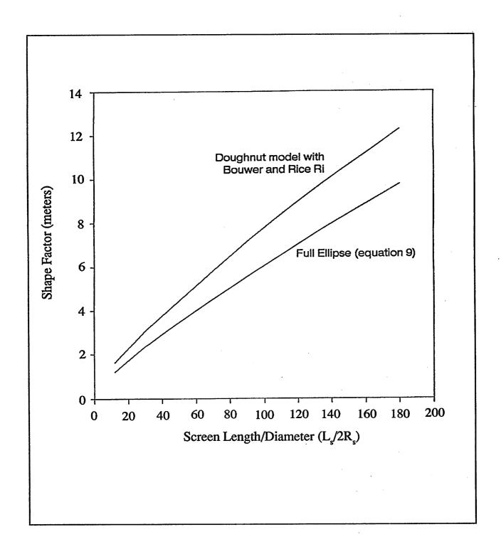
Figure 15. Comparison of shape factors for the doughnut model using Bouwer and Rice (1976) radii of influence, and for the full ellipse model for a 2.54 cm radius well screen.
