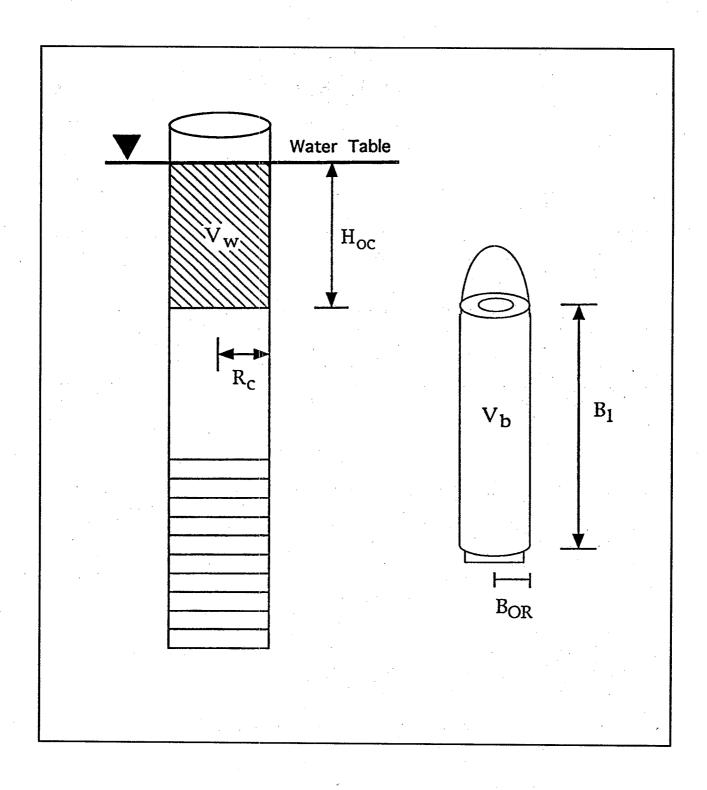
Figure 26. Illustration of parameters needed to calculate the initial head drop.
