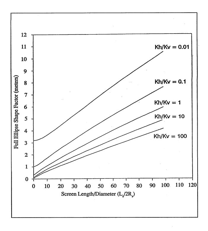
Figure 22. Influence of anisotropy on the full ellipse shape factor for a 2.54 cm radius well screen.  $K_h$  and  $K_v$  correspond to the horizontal and vertical hydraulic conductivities, respectively.
