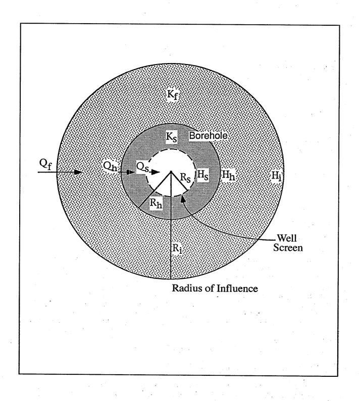
Figure 20. Plan view of a well identifying parameters used to derive effective hydraulic conductivity equation. Q, R, K, and H represent the flow, radius, hydraulic conductivity and hydraulic head at the labeled boundaries, respectively.
