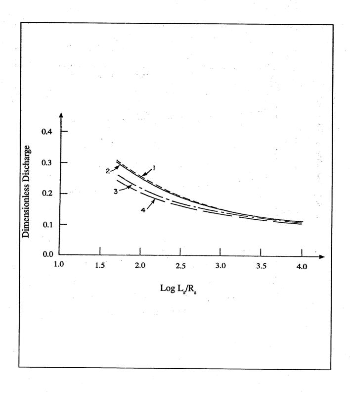
Figure 17. Comparison of cylindrical intake dimensionless discharge terms. (1) Braester and Thunvik's (1984) numerical solutions; (2) Dagan, 1978; (3) Hvorslev, 1951; and (4) Moye, 1967.  $L_s$  = well screen length;  $R_s$  = well screen radius. After Braester and Thunvik, 1984.
