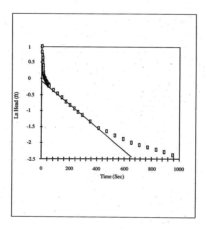
Figure 25. Slug test recovery curve from a typical monitoring well with a partially submerged well screen. Well MMW-8; UCONN Motorpool, August 6, 1991. After Binkhorst, 1992.
