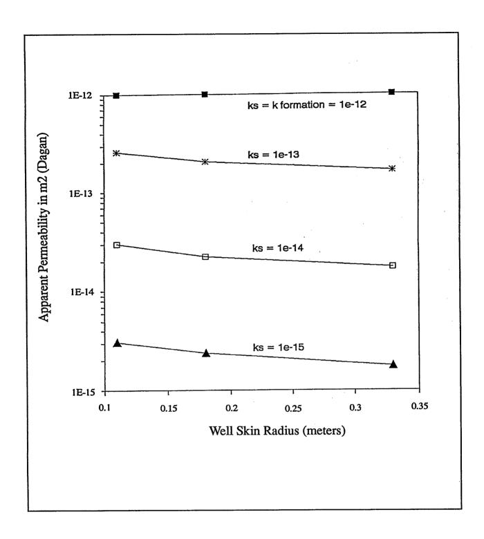
Figure 18. Apparent formation permeability for different well skin permeabilities ( $k_s$ ) and thicknesses, using data from Braester and Thunvik, 1984.
