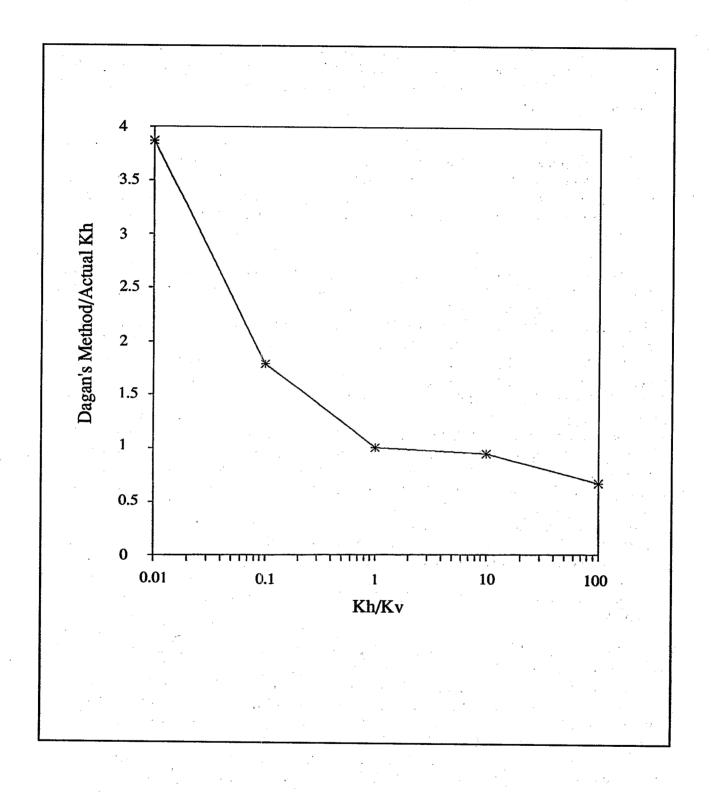
Figure 23. Comparison of the isotropic hydraulic conductivity of Dagan (1978) with the anisotropic conductivity of Braester and Thunvik (1984); developed using data from Braester and Thunvik.
