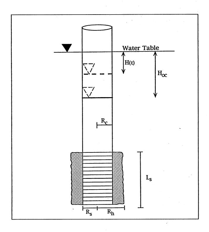
Figure 3. Hydraulic head representation following a slug out test.  $L_s$  = screen length,  $R_h$  = borehole radius,  $R_o$  = well screen radius,  $R_o$  = well casing radius,  $H_{oc}$  = calculated initial drawdown, and H(t) = head at any time t.
