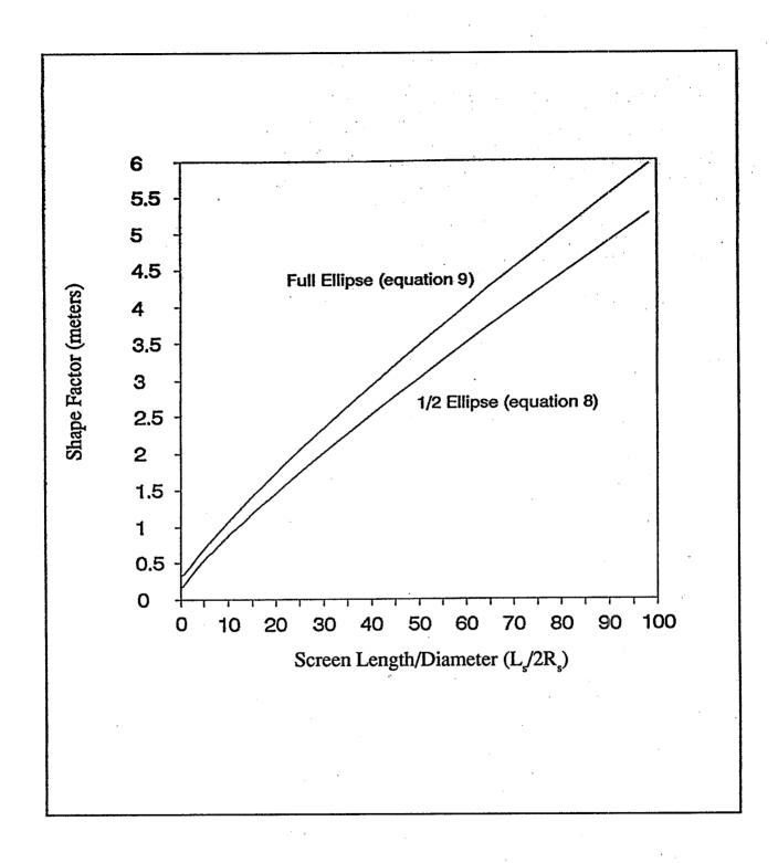
Figure 9. Comparison of analytical shape factors for the 1/2 and full ellipse models for 2.54 cm (1 inch) radius well screen and screen lengths ranging from 0.01 to 5 meters.
