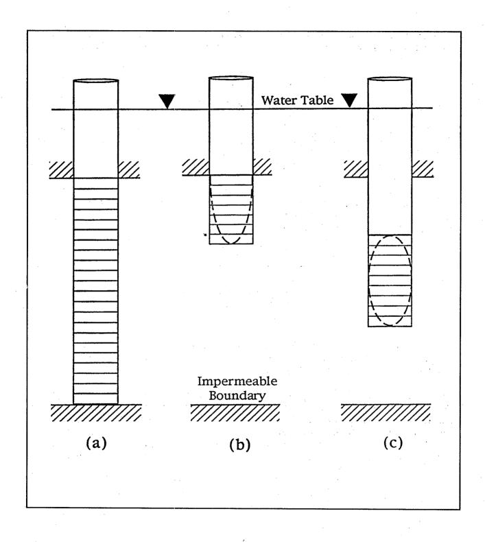
Figure 2. Slug test geometries for (a) doughnut, (b) 1/2 ellipse, and (c) full ellipse models.
