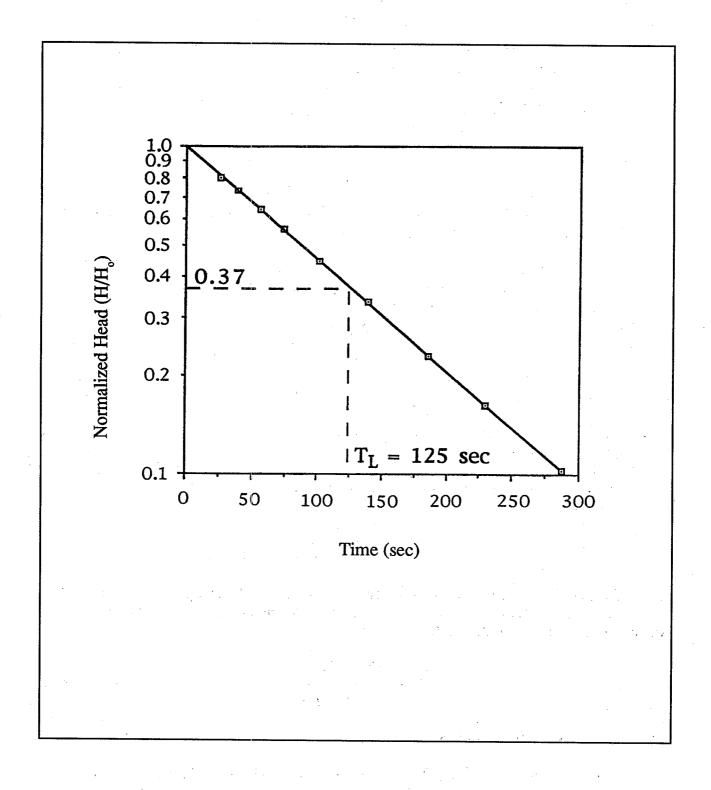
Figure 5. Hvorslev Basic Time Lag method. H = head at given time,  $H_o = initial$  head drop, and  $T_L = the$  Basic Time Lag.
