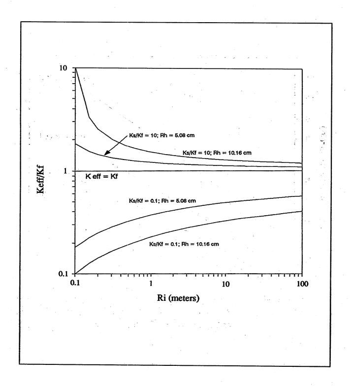
Figure 21. Effects of well skin and radius of influence on the effective hydraulic conductivity for a 2.54 cm radius well screen. The radius of the well skin is given as the hole radius  $(R_h)$ .
