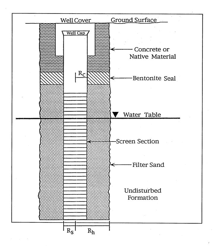
Figure 1. Typical ground water monitoring well with partially submerged well screen.  $R_s$  = screen radius;  $R_h$  = borehole radius;  $R_c$  = well casing radius.
