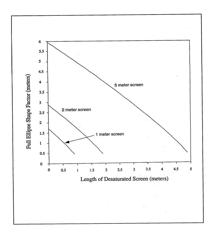
Figure 29. Changes in the full ellipse model shape factor caused by screen length reduction resulting from filter sand pack drainage-for a 11.43 cm radius borehole.
