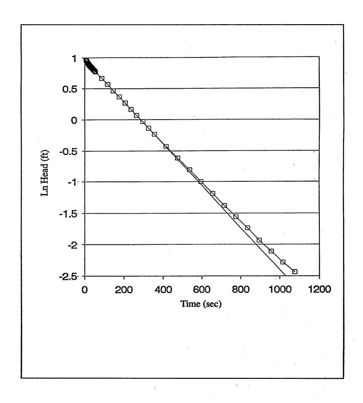
Figure 4. Typical slug out test recovery curve for a monitoring well with a fully submerged well screen. Well TJ-1; UCONN Beach Hall; March 27, 1991. After Binkhorst, 1992.
