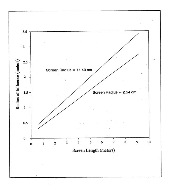
Figure 14. Impact of screen length and screen radius on the radius of influence, calculated using the Bouwer and Rice (1976) method.
