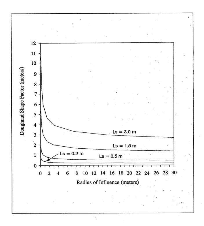
Figure 11. Impact of the radius of influence and screen length  $(L_s)$  on the doughnut model shape factor for a 2.54 cm radius well screen.
