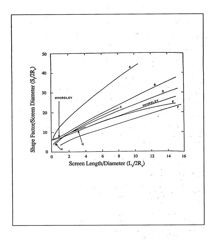
Figure 10. Comparison of analytical, electric analog, and numerical shape factors (normalized to the screen diameter) for cylindrical intakes. A = Randolph and Booker, 1982; B = Wilkinson, 1968; C = Tavenas et al., 1968a; D = Brand and Premchitt, 1980; E = Kallstenius and Wallgren, 1956; F = Raymond and Azzouz, 1969; G = Al-Dhahir and Morgenstern, 1969; H = Smiles and Young, 1956. After Chapuis, 1989.
