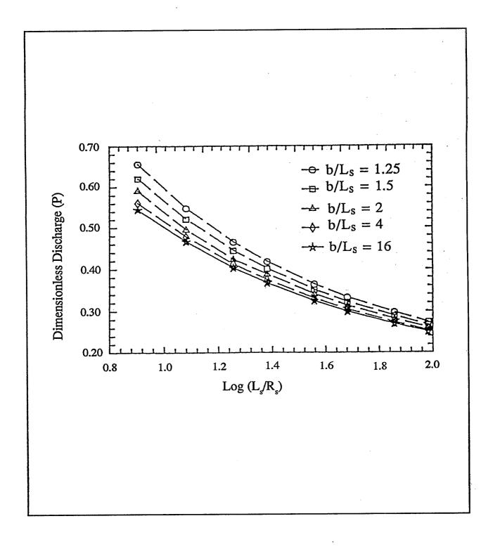
Figure 8. Variation in dimensionless discharge (P) for different degrees of partial penetration. b = aquifer thickness,  $R_s$  = well screen radius, and  $L_s$  = well screen length. After Widdowson et al., 1990.
