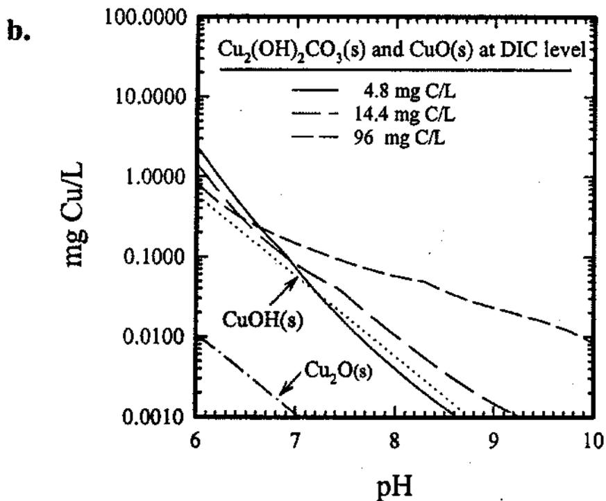
Figure 13. Copper(II) solubility of different DIC levels compared to copper(I) solubility, at  $I = 0.01$ ,  $25^{\circ}\text{C}$  for: a) new pipe with  $\text{Cu}(\text{OH})_2(\text{s})$ ; b) aged pipe.
