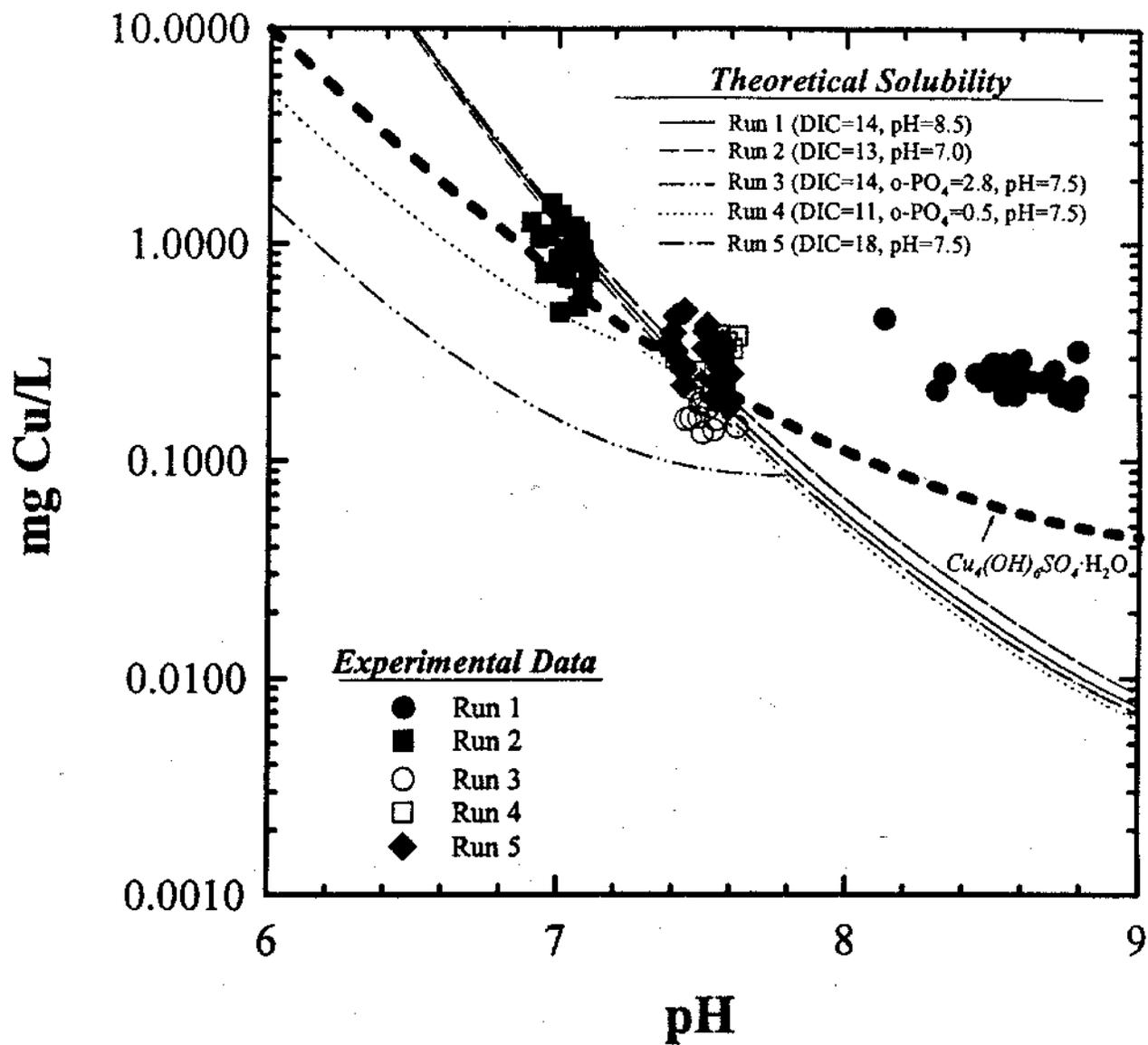
Figure 20. Comparison of theoretical and observed copper levels for coupon study. The wide dashed line indicates the predicted solubility of a hydrated cupric hydroxysulfate in comparison to cupric hydroxide or cupric orthophosphate phases.
