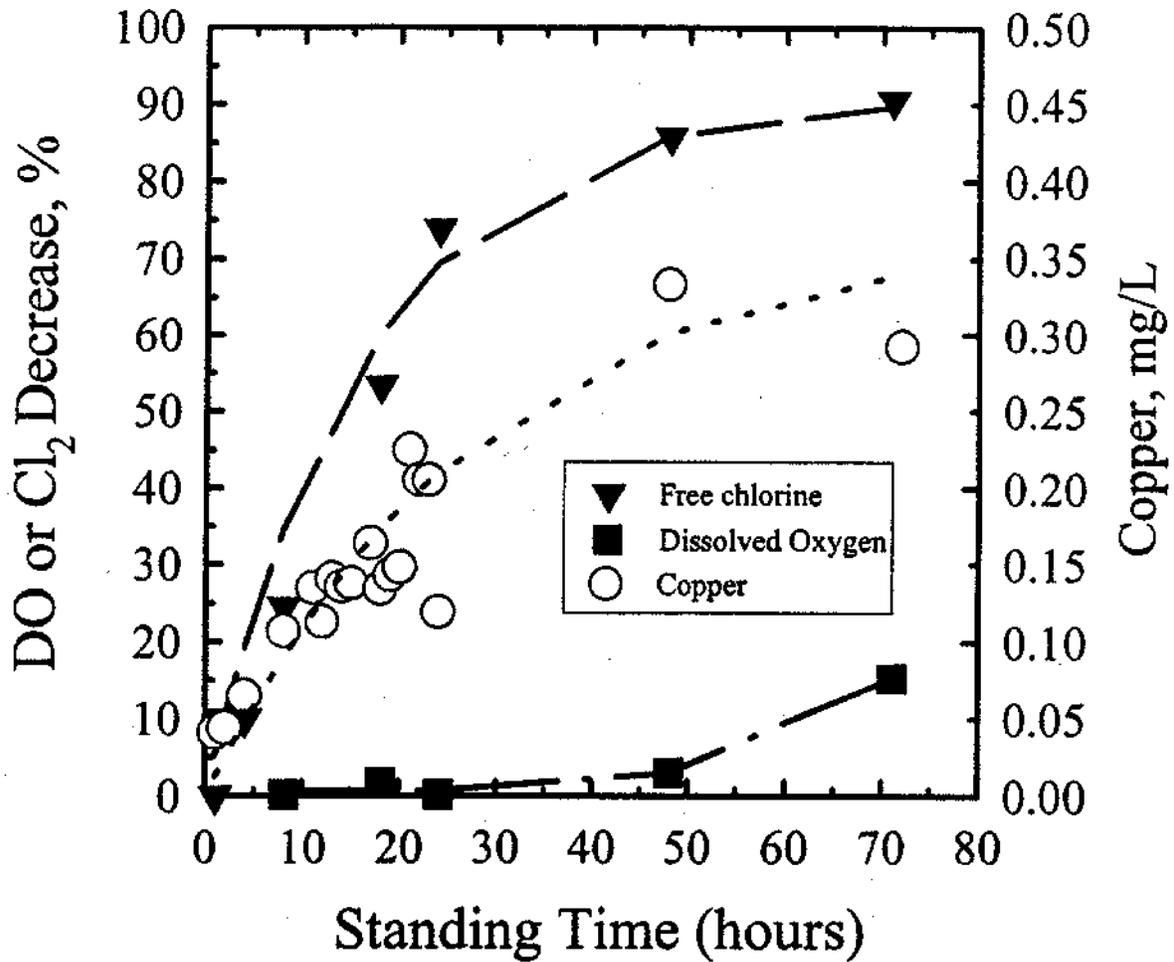
Figure 15. Relationship among depletion percentage for free chlorine residual, dissolved oxygen, and copper concentration over varying stagnation lengths, after 250 days of pipe use.
