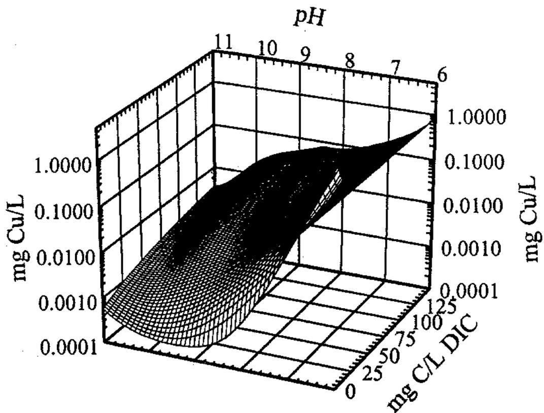
Figure 6. Three-dimensional surface plot of the effect of DIC and pH on copper(II) solubility for aged systems, assuming equilibrium with  $\text{Cu}_2(\text{OH})_2\text{CO}_3$  and  $\text{CuO}$  ( $I=0.02$ ,  $25^\circ\text{C}$ ).
