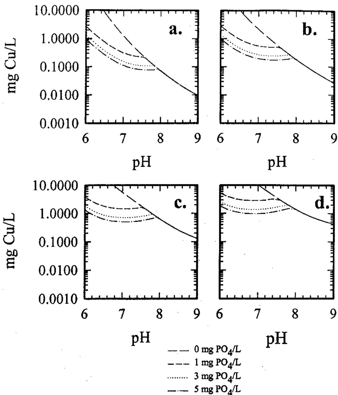
Figure 10. Copper(II) solubility for different DIC levels with orthophosphate addition, assuming formation of  $\text{Cu}(\text{OH})_2(\text{s})$  and  $\text{Cu}_3(\text{PO}_4)_2 \cdot 2\text{H}_2\text{O}(\text{s})$  at 25°C: a) DIC = 4.8 mg C/L, I = 0.005; b) DIC = 14.4 mg C/L, I = 0.005; c) DIC = 48 mg C/L, I = 0.01; d) DIC = 96 mg C/L, I = 0.02.
