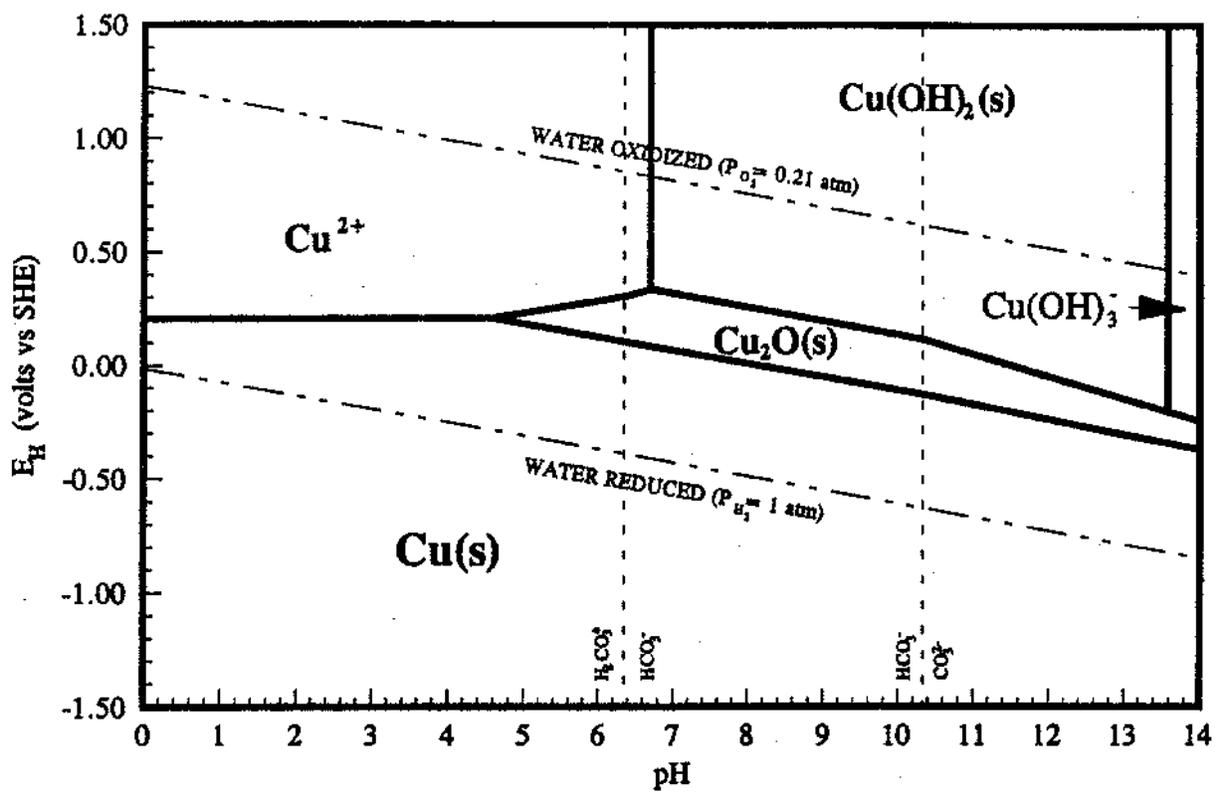
Figure 11. EMF-pH diagram for copper in water containing carbonate, assuming formation of cupric and cuprous hydroxide at DIC = 4.8 mg C/L,  $I = 0$ , copper species concentrations of 1.3 mg/L, and 25°C.
