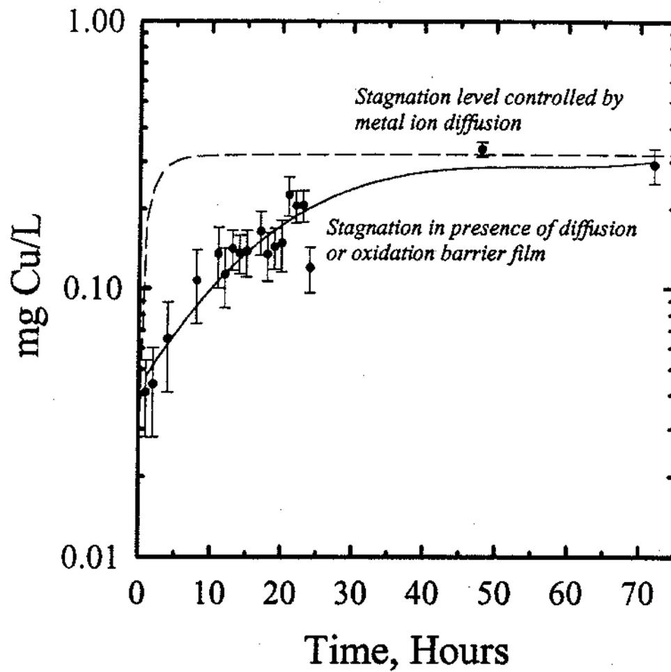
Figure 17. Schematic illustration comparing metal concentrations that would be observed after standing different amounts of time given different controlling chemistry factors.
