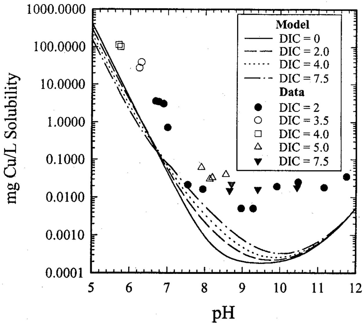
Figure 18. Precipitation date of Patterson (1981) superimposed on two theoretical models for Cu(II) solubility at low DIC concentrations. Models computed for  $I = 0.01$ , and  $25^\circ$ . Controlling solids were assumed to be: a)  $\text{CuO(s)}$  and  $\text{Cu}_2(\text{OH})_2\text{CO}_3(\text{s})$ ; b;  $\text{Cu}(\text{OH})_2(\text{s})$
