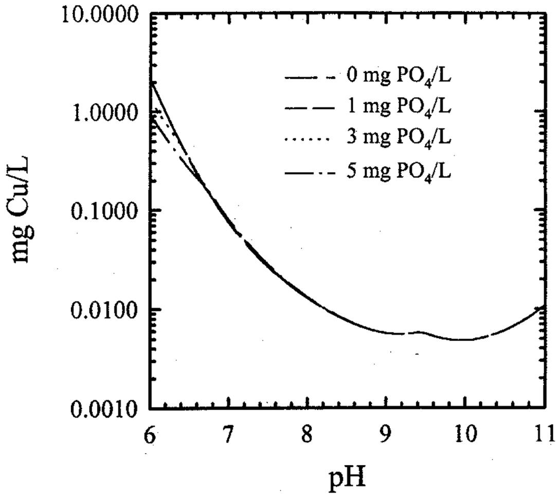
Figure 9. Effect of orthophosphate on copper(II) solubility at DIC = 4.8 mg C/L, I = 0.005 and 25°C, assuming the formation of  $\text{Cu}(\text{OH})_2(\text{s})$ ,  $\text{Cu}_2(\text{OH})_2\text{CO}_3(\text{s})$ , and  $\text{Cu}_3(\text{PO}_4)_2 \cdot 2\text{H}_2\text{O}$ .
