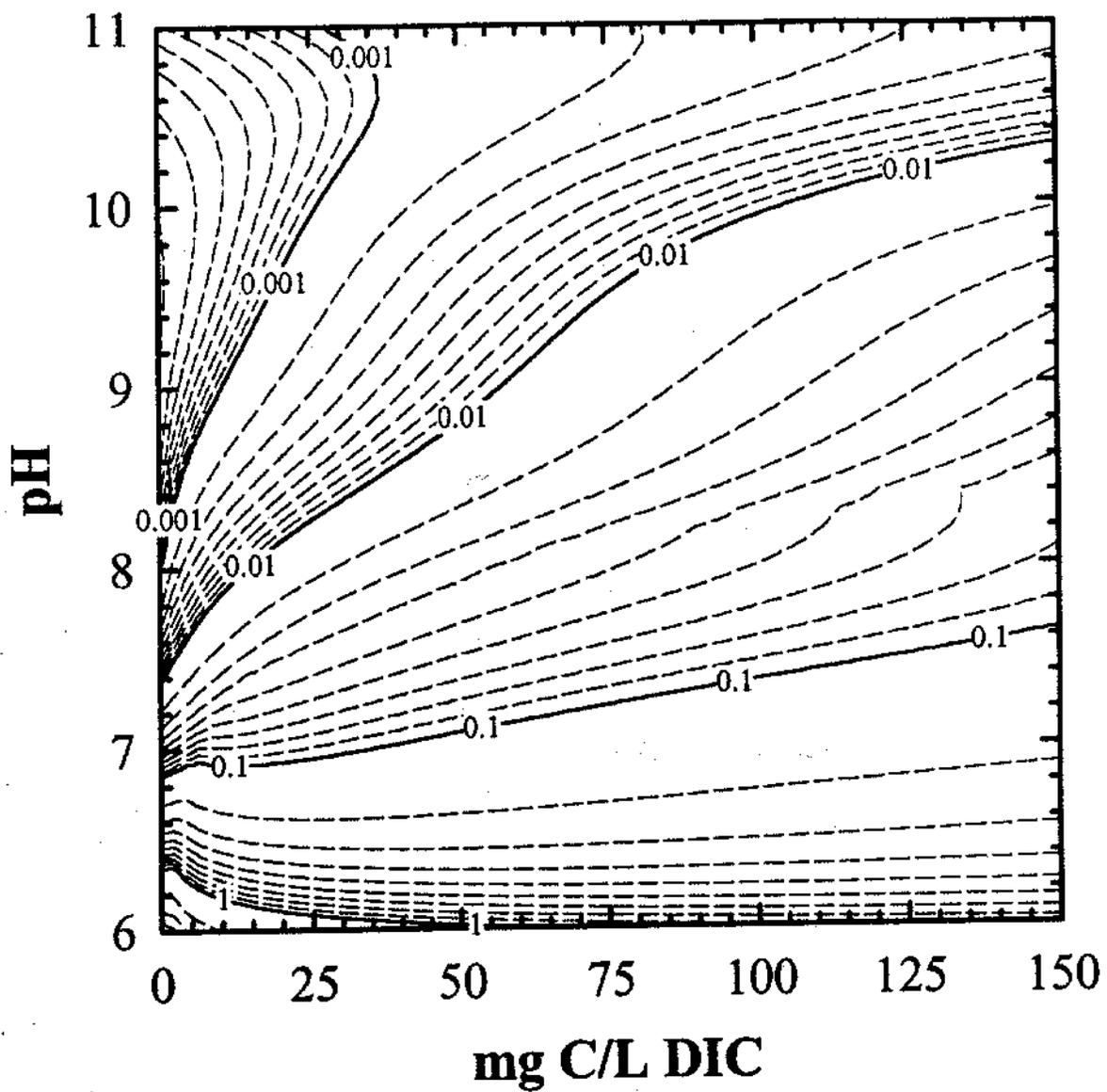
Figure 7. Contour diagram showing the effect of DIC and pH on copper(II) solubility, assuming equilibrium with the stable solid phases  $\text{Cu}_2(\text{OH})_2\text{CO}_3$  (malachite) and  $\text{CuO}$  (tenorite) at  $I=0.02$  and  $25^\circ\text{C}$ .
