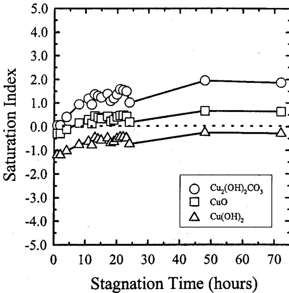
Figure 16. Saturation index changes for three solids during stagnation of different durations in copper pipe loop study. Pipe was aged approximately 250 days
