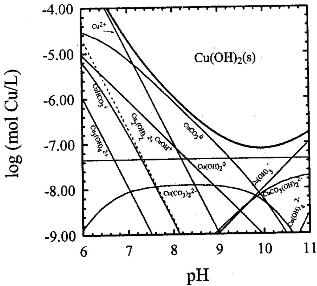
Figure 5. Copper(II) speciation assuming formation of solid  $\text{Cu}(\text{OH})_2$ ; a)  $\text{DIC}=4.8 \text{ mg C/L}$ ,  $I=0.005$ ,  $25^\circ\text{C}$ ; b)  $\text{DIC}=96 \text{ mgC/L}$ ,  $I=0.02$ ,  $25^\circ\text{C}$ .
