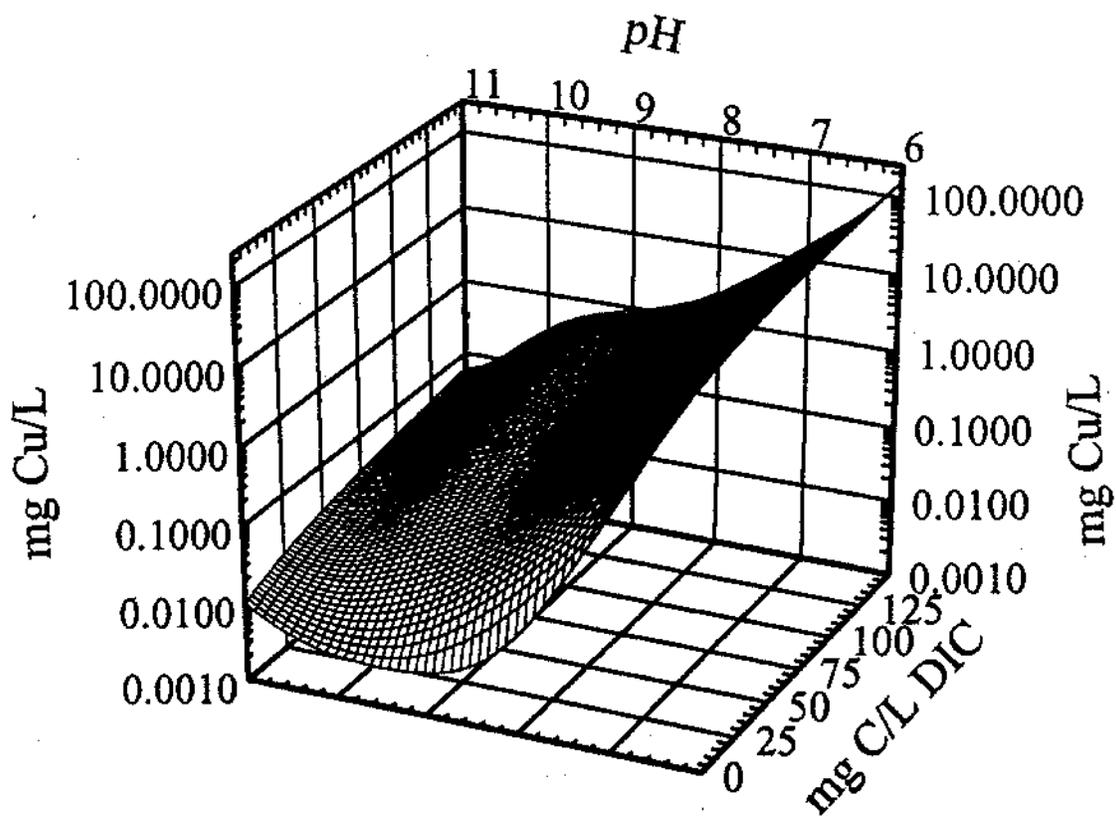
Figure 3. Three-dimensional surface plot of the effect of DIC and pH on copper (II) solubility, assuming equilibrium with  $\text{Cu}(\text{OH})_2$  having a large molar surface ( $I=0.02$ ,  $25^\circ\text{C}$ ).
