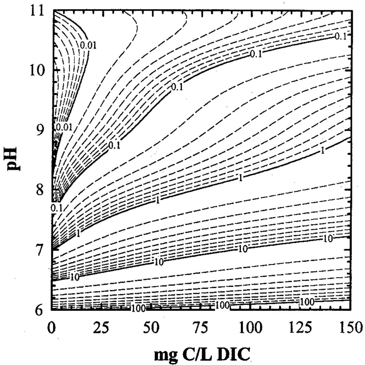
Figure 4. Contour diagram showing the effect of DIC and pH on copper(II) solubility, assuming equilibrium with  $\text{Cu}(\text{OH})_2$  solid having a large molar surface ( $I=0.02$ ,  $25^\circ\text{C}$ ).
