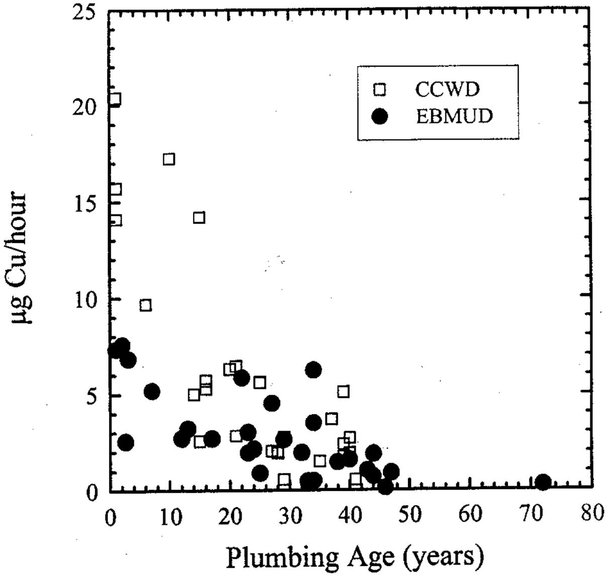
Figure 22. Distribution of adjusted copper leaching rates versus age of plumbing for one litre samples from the residential metals study of the Contra Costa Central Sanitary District.
