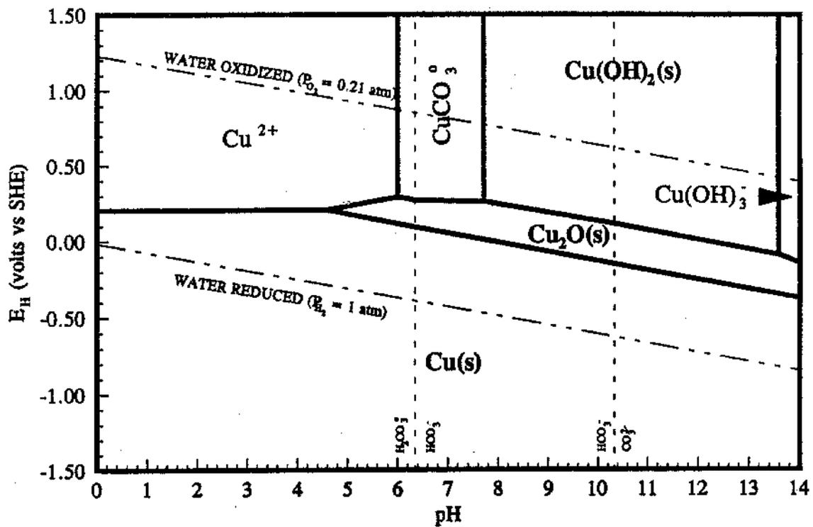
Figure 12. EMF-pH diagram for copper in water containing carbonate, assuming formation of cupric and cuprous hydroxide at  $DIC = 96 \text{ mg C/L}$ ,  $I = 0$ , copper species concentrations of  $1.3 \text{ mg/L}$ , and  $25^\circ\text{C}$ .
