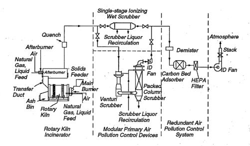
Figure 1. Schematic of the IRF rotary kiln incinerator system.
