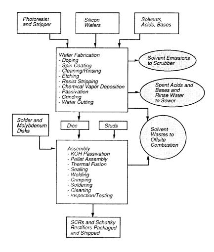
Figure 1. Abbreviated process flow diagram.
