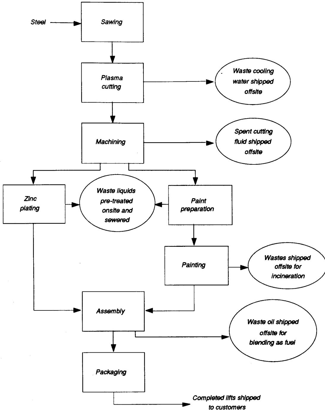
Figure 1. Abbreviated Process Flow Diagram for Lift Manufacturing.
