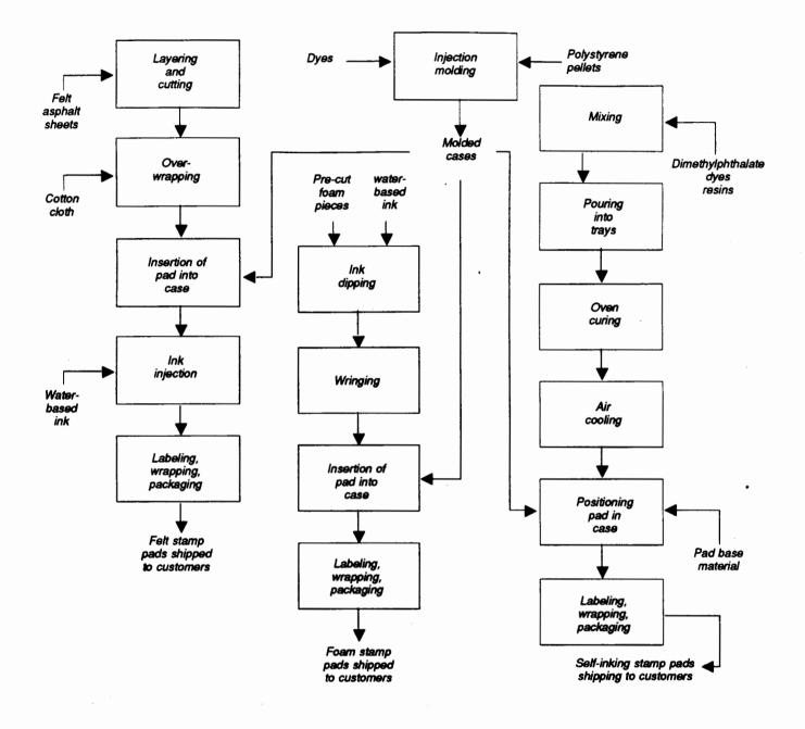
Figure 2. Abbreviated process flow diagram for stamp pad production.
