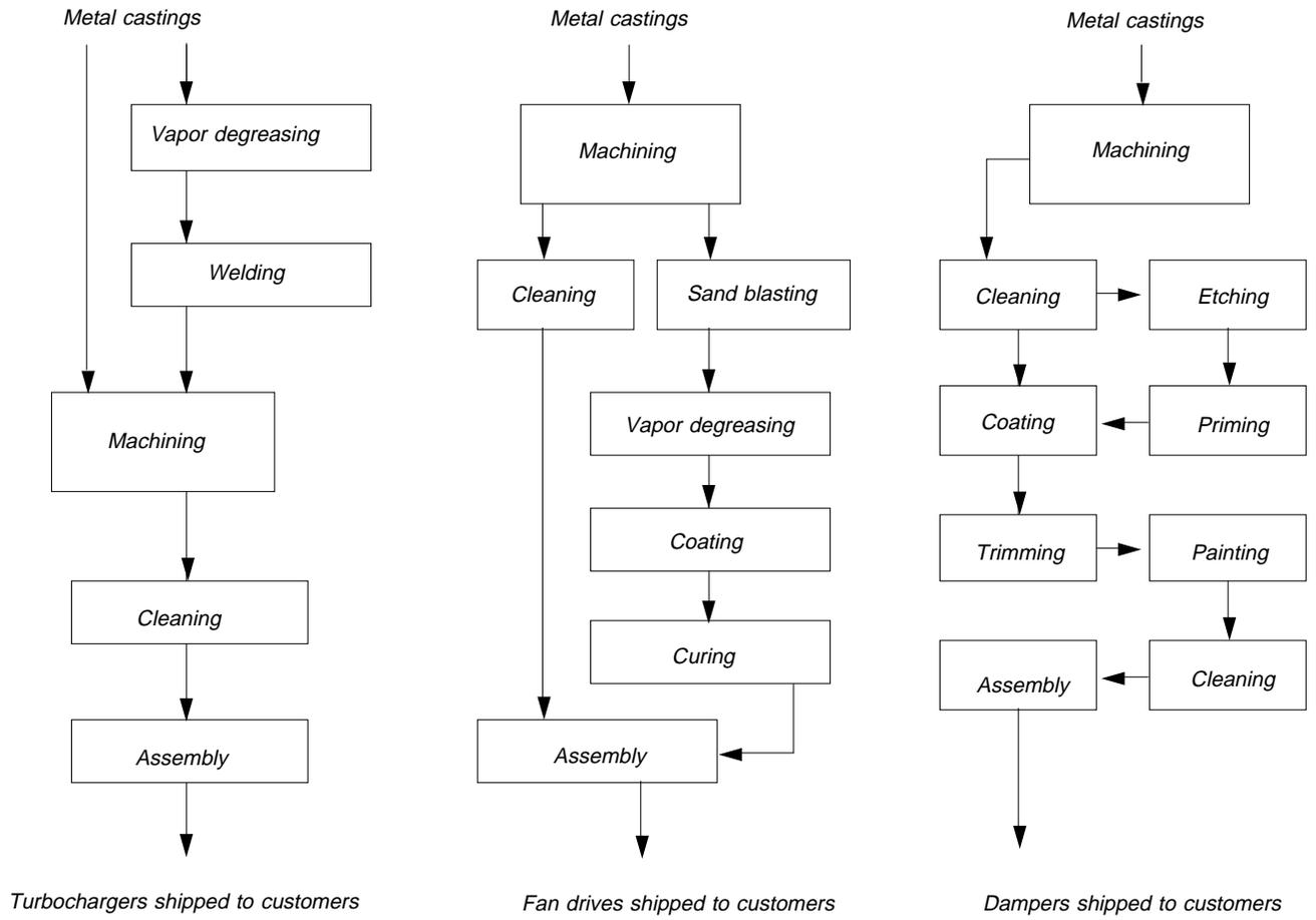
**Figure 1.** Abbreviated process flow diagram for truck engine parts manufacture.
