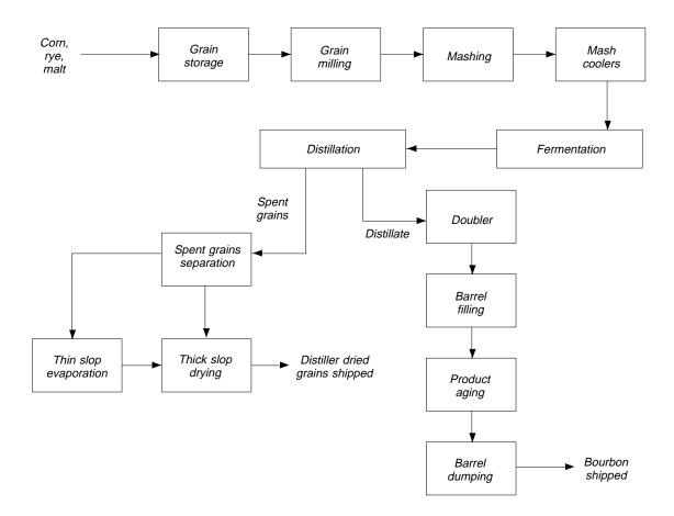
Figure 1. Abbreviated process flow diagram for bourbon whiskey production.
