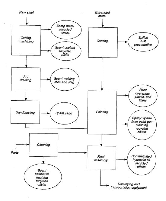
Figure 1. Abbreviated process flow diagram for conveying and transportation equipment manufacture.
