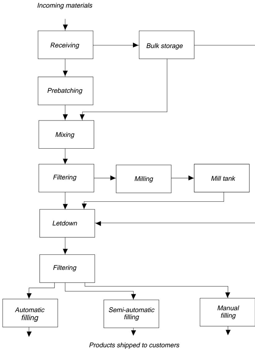
**Figure 1.** Abbreviated process flow diagram for paint formulation.
