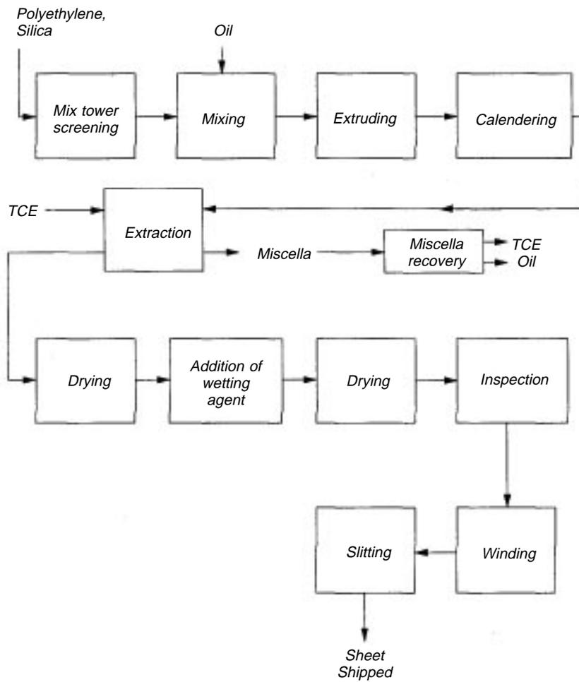
**Figure 1.** Abbreviated process flow diagram for polyethylene/silica sheet production.
