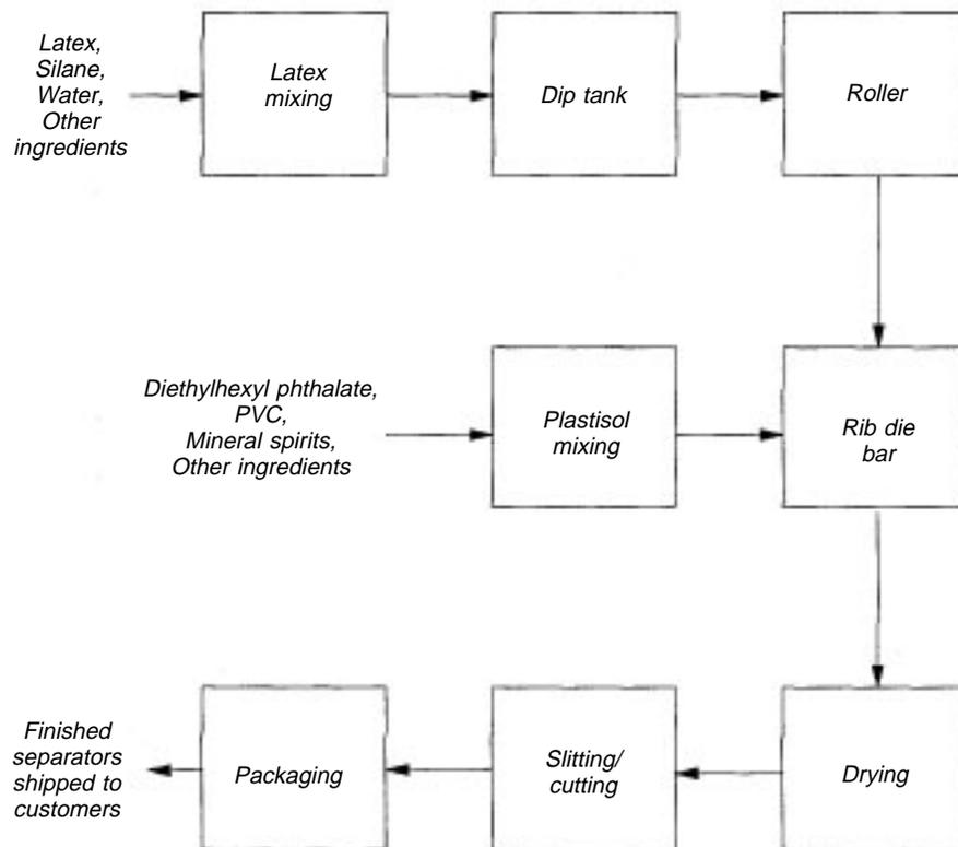
**Figure 2.** Abbreviated process flow diagram for vinyl rib separator production.
